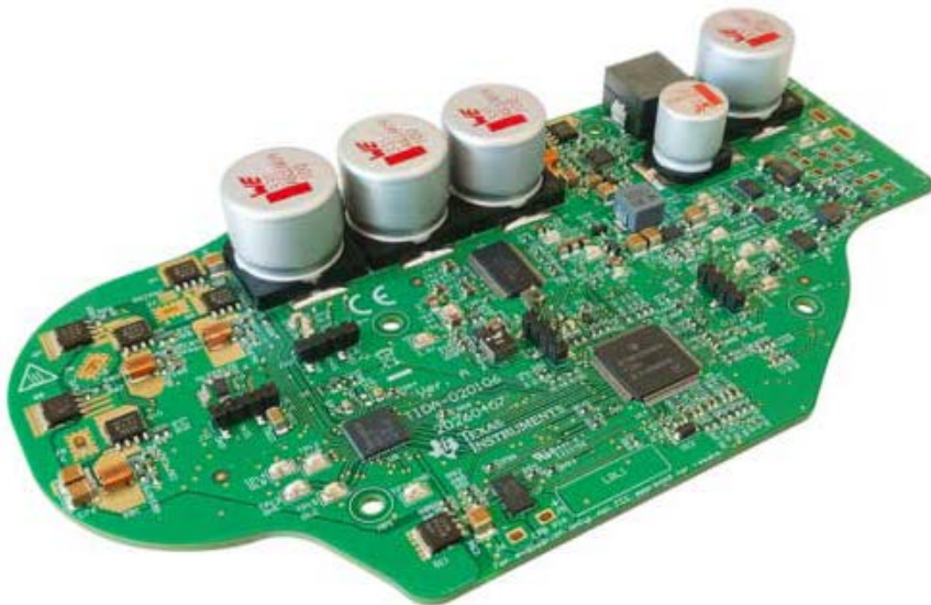
2. TI has assembled a board based on its TIDA-020106 reference design for testing and validation. (Credit: Texas Instruments)
