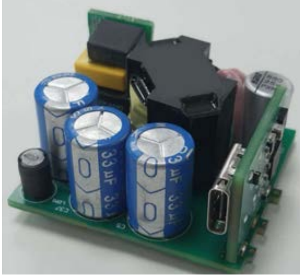
3. Shown is a 65-W USB-C QR flyback converter on a PCB measuring 39 × 34 × 17 mm.
