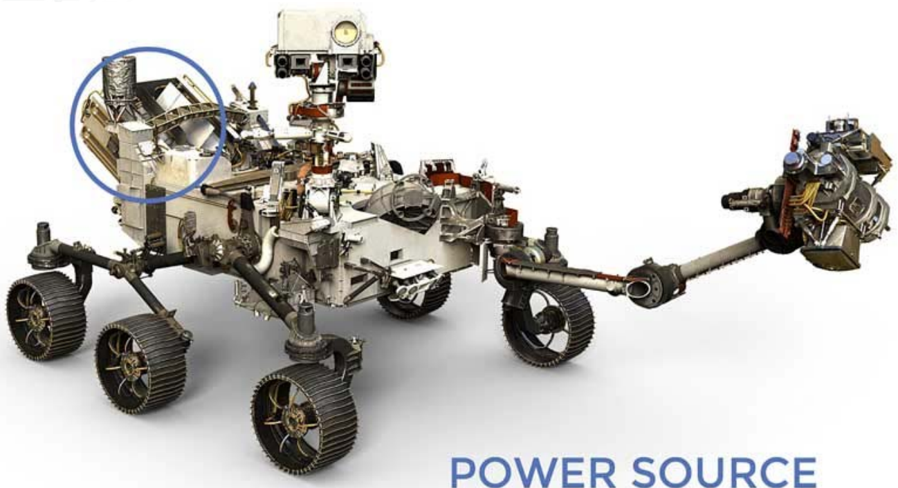
3. The Mars Perseverance Rover radioisotope power system is circled in blue. (Image: NASA)
