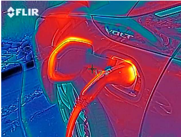
2. FLIR MSX (Multi-Spectral Dynamic Imaging) adds visual imagery outlines, words, numbers, and other high-contrast edge details to the thermal image for better image definition and accuracy.
