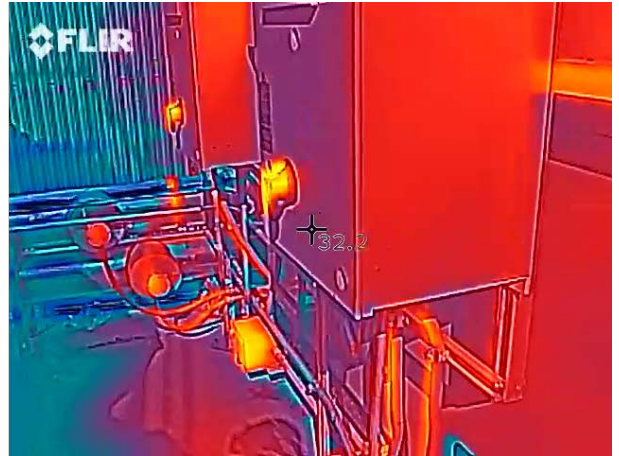
2. FLIR MSX (Multi-Spectral Dynamic Imaging) adds visual imagery outlines, words, numbers, and other high-contrast edge details to the thermal image for better image definition and accuracy.
