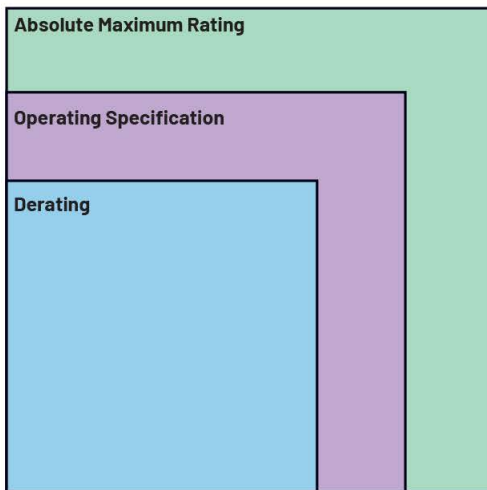
(a) Component Derating Illustration
