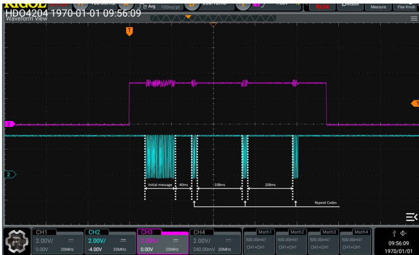
11. Shown are the modulated output signal covering the initial message and repeat code obtained on the demonstration board.
