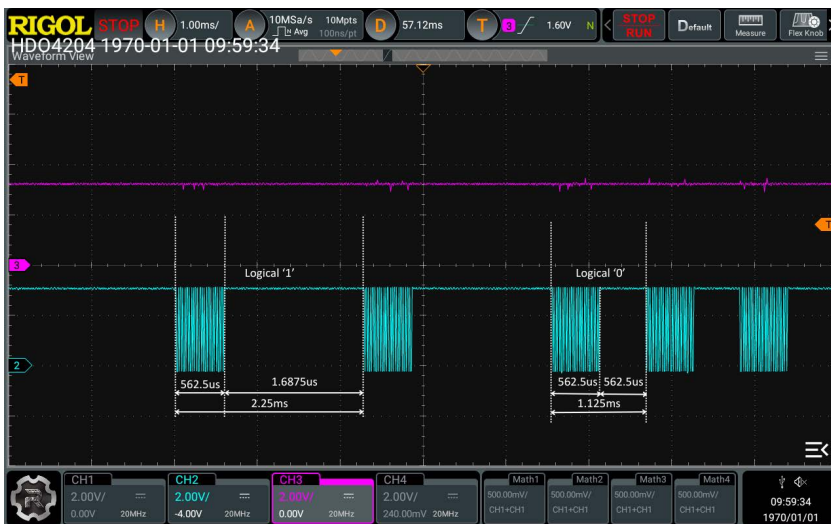
13. Logical '1' and '0' standardized timeframes are shown to be further confirmed via Cursor measuring tool.
