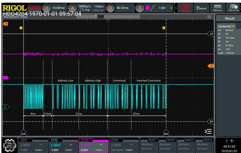
12. The initial message timeframe measured via Cursor tools to confirm that the message transmission timing complies with the NEC protocol specification.
