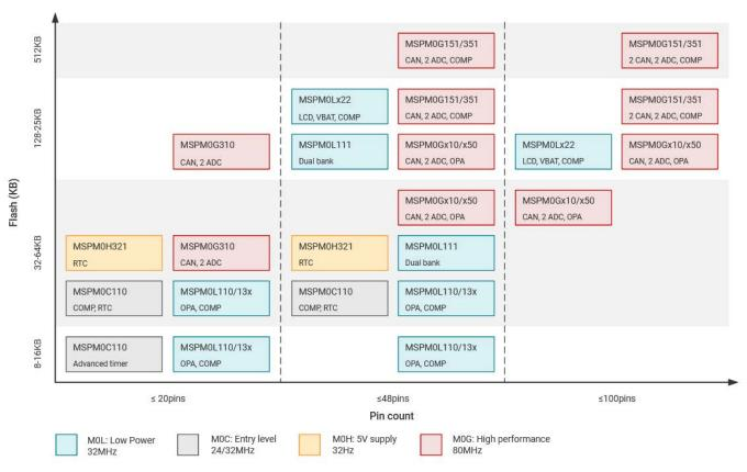
2. TI offers an array of Arm Cortex-M0+ devices with pin-to-pin scalability across memory and packages (Source: TI).
