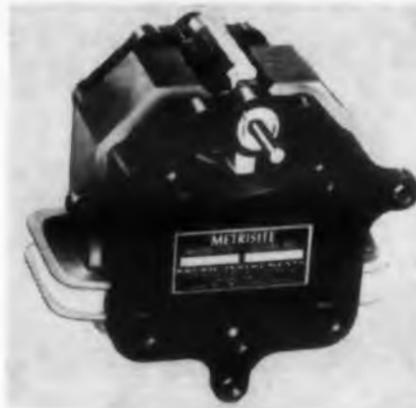
Type 34A rugged, angular motion Metrisite transducer converts angular motion of up to  $\pm 40$  deg to voltage outputs with 0.25% linearity. The device has a negligible reactive force. It measures 3 x 2-5/8 x 1-7/8 in. and weighs 20 oz.
