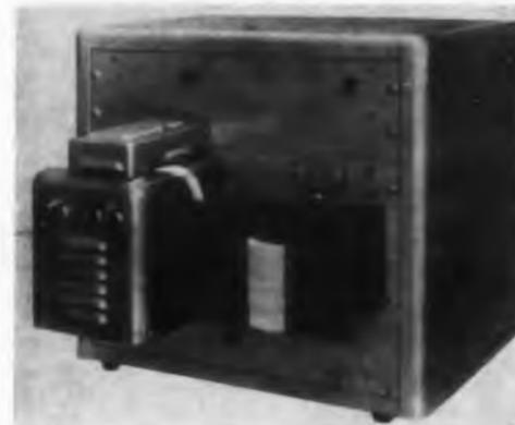
The model 600 Tape Reader is capable of providing outputs at up to 600 characters per sec, on a start-stop basis. The reader, especially suited to industrial automated control systems, reads 5, 6, 7, or 8 level code combinations on
