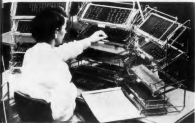
Parts are removed from individual component boards for attachment into actual Minuteman circuits.
