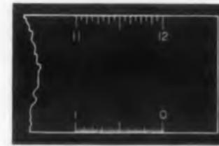
Fig. 8. Shortening length of lines on linear scale of Fig. 6 improves readability.
