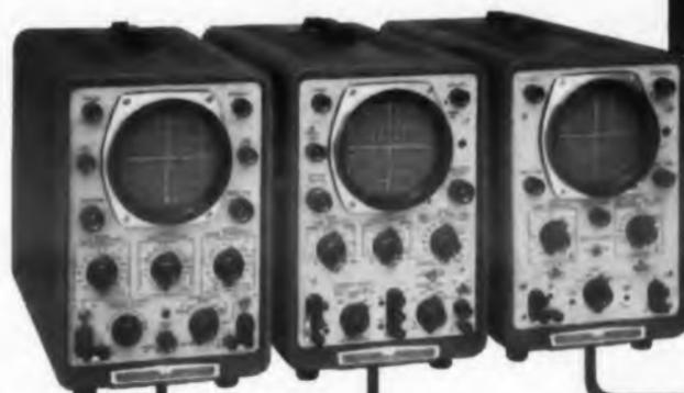
Production or lab instruments—Simple to use, even for non-technical personnel—Moderately priced—Full 10 cm x 10 cm display—Automatic calibration waveforms—Low phase shift—Automatic triggering for optimum presentation—"Times-5" sweep expander magnifies trace, improves resolution.
