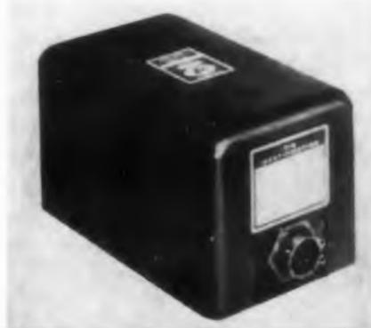
These static inverters, series 115SA, available in three power ratings, have fast response, low distortion, and lightweight design. They provide 400 cps power for airborne or missile applications at either 100, 250, or 500 v. Units, transistorized, measure 7 x 10 x 6 in. max and weigh from 6 to 20 lb. MIL specs are met.
