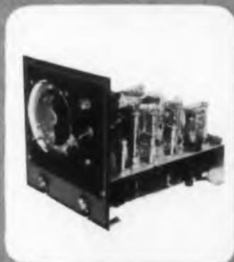
Basic chassis, with sub-assemblies in place, provides for fast, easy accessibility. Simple half turn of special Serve-a-Unit lock guides, locks or ejects for easy service checks, repairs, or 30-second replacement.
