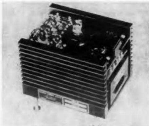
This line of ac to dc power supplies provides 0.1% regulation for line and load variations on units rated at 5 v and up, and a 0.5% regulation on units rated below 5 v. Response time is less than 100  $\mu$ sec for 10% line transient or 50% load transient. Ripple is 0.02% or 5 mv rms. Temperature coefficient is 0.01% per deg C. Outputs are 2 to 305 v dc from 100 ma to 1 amp. The units are plug-in type and are built on heat-sink chassis.
