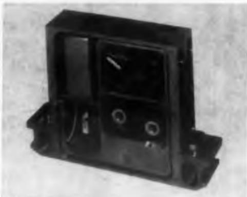
Model 2900 dc differential amplifier has over 500-meg input resistance, voltage gains of 2 to 50, and over-all linearity of 0.05%. A missile-grade mechanical chopper and a silicon-transistor carrier amplifier are used. Output voltage is  $\pm 5$  v. Power consumption is 140 ma from an unregulated 28-v source. Construction is of cast magnesium alloy.
