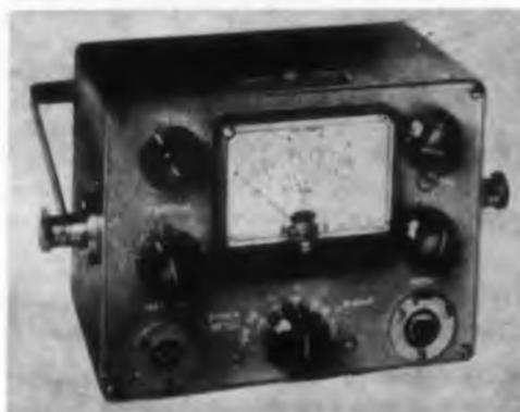
Model B832T temperature-compensated power meter measures cw or pulsed rf power in five full scale direct-reading ranges from 30  $\mu$ w to 3 mw. Values can be read in mw or dbm. Readings are
