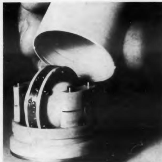
The tiny ceramic spin motor of the gyro is encased in its gimbal, also of ceramic. The ability of the ceramic material to withstand heat up to 1,500 F without losing its original dimensions represents a major improvement over ball bearings.
