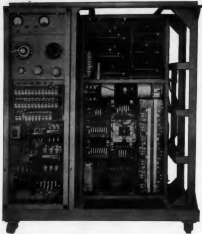
Regulated, multiple voltage output +250 volts, +150 volts, +70 volts, +70 volts, +250 volts, -35 volts, -50 volts, -60 volts, -70 volts, -250 volts D.C. 6.3 volts, 115 volts, A.C. Total power capacity approx. 15 KW
