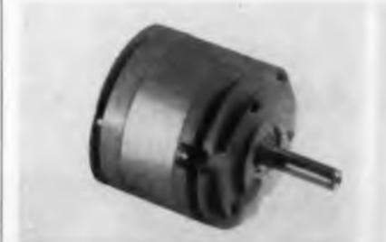
These easily detachable heads are available in various frame sizes, and supply reductions in ratios ranging from 7.22:1 to 42,471.90:1. Ball bearings are Class A. B. E. C. 5, or better, and gears are cut to AGMA Precision II tolerances, or better, with backlash held to 30 minutes, or better. Adaptable to variety of motors and motor generators. Write for details.
