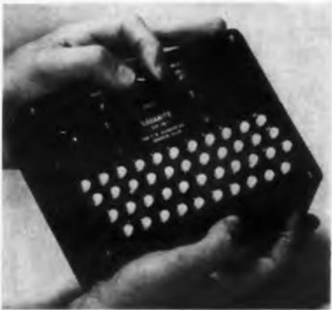
The Codamite transistorized code generator, measuring 6.25 x 5.25 x 2.25 in., produces 43 different code characters. Circuitry includes a ten-bit magnetic core memory to retain each character until transmitted. A speed control provides for rates of transmission from 5 to 40 words per min. R. W. Johnson Co., Dept. ED, 9372 Hillview Road, Anaheim, Calif.
