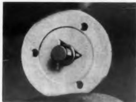
These miniature disk cathodes with triangular ceramic insulators provide a minimum heat sink by reducing the area of contact between the tank and the ceramic. The temperature of the cathode can be as high as 850 C. Shank diameter is about 0.09 in. and length, 0.22 to 0.28 in. The disk cathodes can be furnished with a 0.365- or 0.40-in. OD ceramic.
