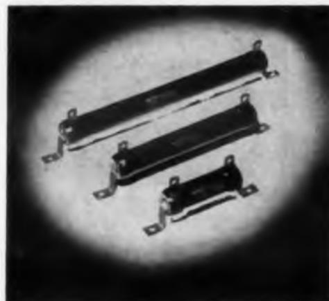
The TO-RW series of wirewound resistors are made to exceed the requirements of MIL-R-26c with "V" characteristics. They use alloy terminals which match the thermal expansion of tube and enamel. Minimum wire size is 0.00175 in.
