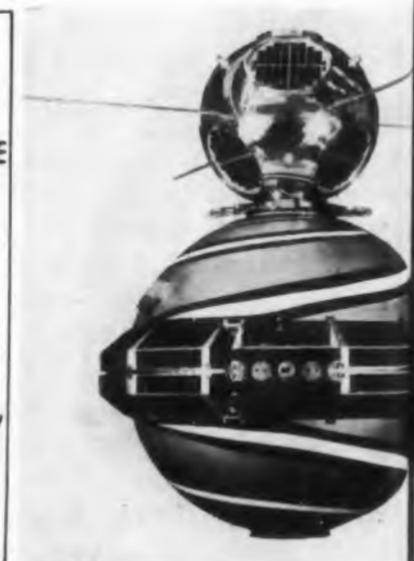
Transit II-A and the radiation-measuring satellite above it orbited together.
