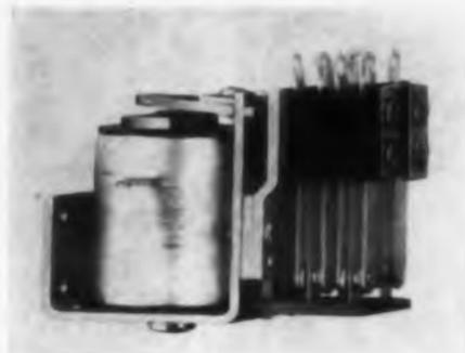
Series TW medium power telephone type relay is available with contact arrangements up to 4 pdt. In voltages from 6 to 220 v ac and dc, 3/16-in. diam contacts made of fine silver and gold flashed are rated at 5 amp at 115 v, and 60 cps, noninductive. Coil resistance is 10 K as standard, higher on request. Applications include: communications equipment, computers, industrial programming devices, and other applications requiring a small, fast-acting multi-contact relay.
