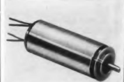
The CK-1066-40-A1 Bendix low inertia motor is a two-phase, four-pole, 400-cycle induction type and is one of the smallest motors available for servo systems. Measured only 0.50" in diameter and 1 1/4" in length. Unit consists of a squirrel-cage rotor that rotates on precision ball bearings, a two-phase stator, and a stainless steel housing. Standard motor has tapered shaft but units can be obtained with other type shafts and with center-tapped control windings.
