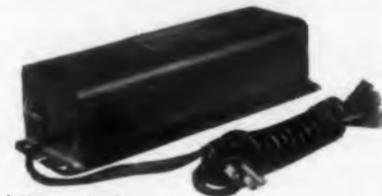
This compact stabilizer design occupies a minimum of space and is especially adaptable as a component in electronic devices where output voltages must be maintained  $\pm 1\%$  of normal. Available in ratings of 15, 25, 50 VA.
