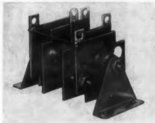
For all basic circuit configurations, these pre-assembled silicon rectifier stacks have piv ratings from 50 to 600 v and current ratings from 2 to 35 amp. Sizes are 2 x 2 in., 2 x 3 in., and 5 x 5 in., all 0.064 in. thick.
