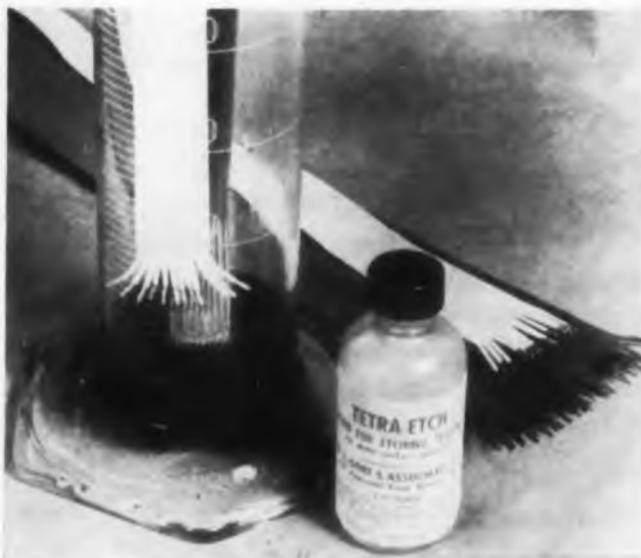
**Fig. 1.** After the cable is slit, it is immersed in the etchant for about 2 min; then residue is removed with water and all surfaces are wiped with acetone. Carbonaceous film formed on the Teflon is the key to tight bonding.
