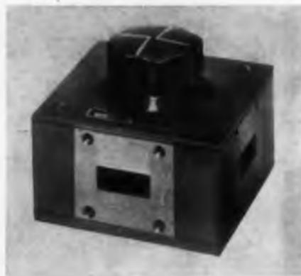
Series 641 waveguide switches cover the range of 3.95 to 40 kmc. Each switch operates over the full waveguide bandwidth. They can be operated manually or driven by a 28 v dc solenoid actuator. Maximum vswr is 1.1; minimum isolation is 60 db for 3.95 to 26.5 kmc and 50 db for 26.5 to 40 kmc.
