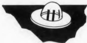
The rounded end of clear-glass gives a distortion-free light when viewed end-on from any angle. Because of its smooth round end, this lamp can be used as a protruding element, thus improving the appearance of the panel.
