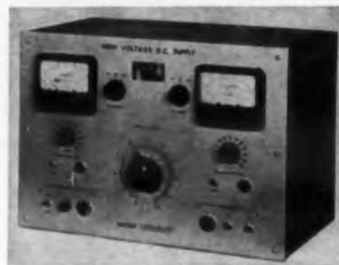
Model PSC 30-5-1 power supply provides an output of 35 kv at 1 ma and 30 kv at 5 ma. Input is 115 v at 60 cps. Ripple is less than 0.5% per ma rms. The unit is portable, measuring 12 x 14 x 12 in. and weighing 60 lb.
