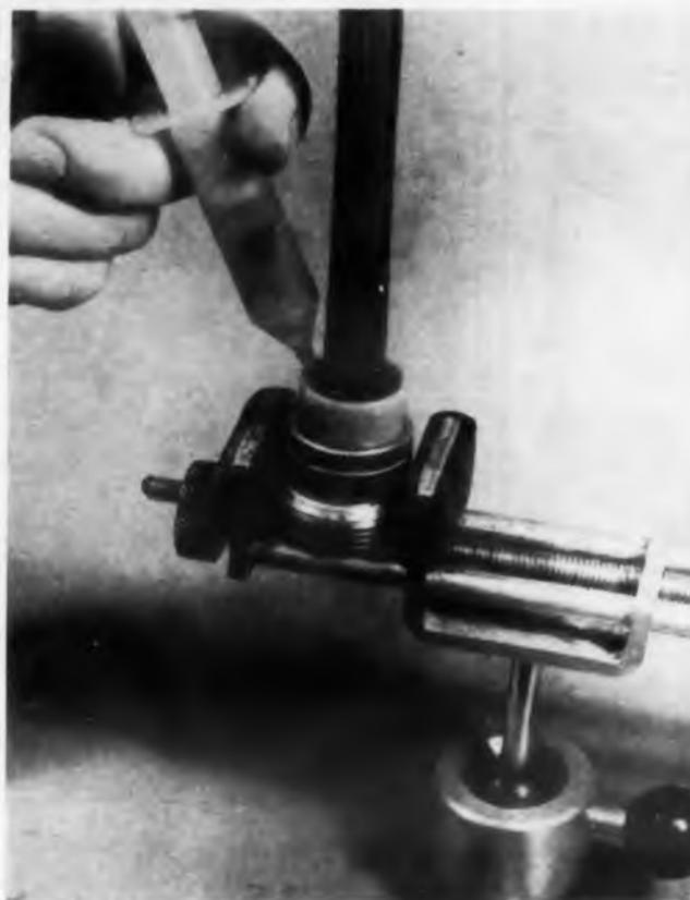
Fig. 3. Finally, the unit is potted. Mechanical fixture assures rigid clamping during subsequent resin cure under heat lamps.
