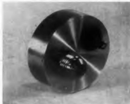
The 800 series pressure transducers use a free-edged, circular diaphragm of Ni-Span-C in the sensor to increase system accuracy. Full scale ranges are 1 to 100 psi; differential or absolute measurements can be made. Units are sensitive to less than 0.01% of full scale for a 0 to 1 atmosphere pressure range. Hysteresis effects are less than 0.03%. Temperature range is -55 to +100 C. The sensor stands 100% overpressure.
