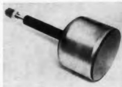
Type 7BCP- magnetic focus and deflection cathode-ray tube is designed for flying spot scanner applications. It has a minimum useful screen diameter of 6-3/4 in., an over-all length of 18-3/8  $\pm 4$  in., and a spot size of 0.0035 in. average. Accelerator voltage is 37,000 v dc and screen current is 300  $\mu\text{a}$ .
