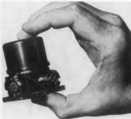
A line of electrically actuated, high-response, hydraulic servo valves is offered for 500-3000psi hydraulic systems. Controlled maximum output flows are 0 to 9gpm with a time constant of approximately
