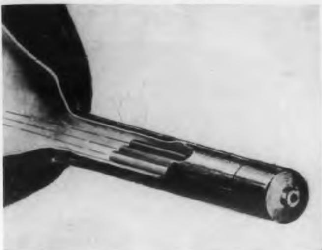
The three electron guns are mounted in the horizontal plane.
