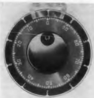
The 900 Series "Duo-dial" turns-counting dial, which replaces this firm's W series, consists of two coaxial dials: the inner counts hundredths of each turn, and the outer counts the number of completed turns. The dial is integrally mounted with the inner dial and connects di-
