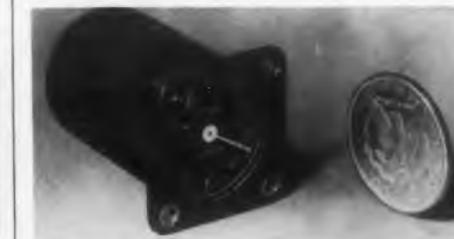
The Model 7008 Running Time Meter indicates up to 10,000 hr on a dial-type face. It weighs less than 6 oz and has a power drain of approximately 2w. It is hermetically sealed in accordance with MIL-I-7793 (AER) and meets military shock (25g) and vibration requirements. Haydon Manufacturing Co., Inc., Dept. ED, Torrington, Conn.
