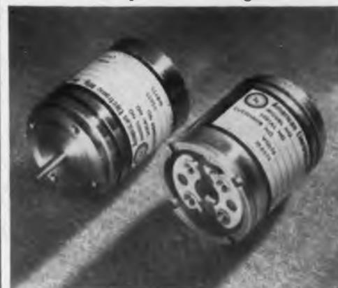
To qualify for the job, the molded parts withstood five room temperature shock tests at 50 "G's" plus constant vibration in the order of 25 "G's" for 4 hours at 600 F. Finally, the potentiometer was subjected to 1050 F for 15 minutes. The terminal blocks molded of Dow Corning 301 Molding Compound were somewhat shrunken and charred, but the brass inserts were still firmly retained. No. 9
