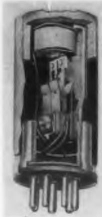
The 1700 Series Heavy-Duty Vibrator, designed especially for communications service, incorporates a design which eliminates the usual contact buttons. The spring leaves themselves, made of special contact alloy, act as contacting members, affording greatly increased contact area.
