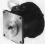
**MODEL 430 AIRCRAFT DRIVE MOTOR** — 1/12 h.p. 11,000 r.p.m. Teflon insulation.  $-65^{\circ}\text{F}$ . to  $+160^{\circ}\text{F}$ . Completely qualified to MIL 7969 specs.
