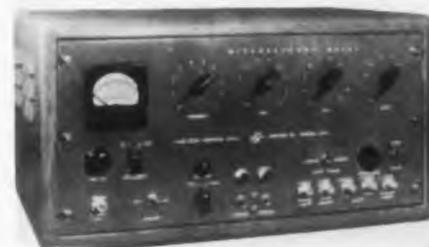
The 1000-A is a precision variable time delay generator which provides a positive pulse variable in delay in increments of 0.1  $\mu$ sec. The delay
