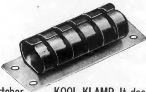
This is a Birtcher **KOOL KLAMP**. It does two jobs. Being made of 99½% pure heat treated silver, it reduces bulb temperature. It also serves to hold miniature and subminiature tubes secure against shock and vibration. If you have a problem of heat and/or retention write today for a catalog and complete details to The Birtcher Corporation, Industrial Division, 4371 Valley Blvd., Los Angeles 32, California.
