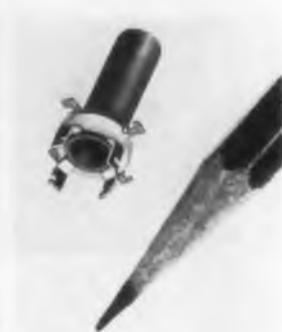
This phenolic coil form, Type SPC, is for printed circuitry. It is available in two diameters with four terminals each, and can be dip soldered after mounting.
