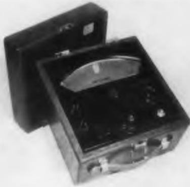
This ohmeter and megohmmeter permits measurement of high resistance values to a fraction of 1%. It has a zero adjustment which compensates for varying battery voltages; once zeroed for one scale, the adjustment is accurate for all scales.
