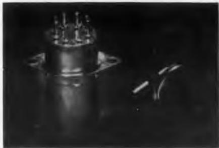
This sensitive subminiature dpdt relay is for jet aircraft, guided missiles, and other airborne applications. It is hermetically sealed and dry nitrogen filled, is only 0.656" diam x 1.500" long, and weighs only 1 oz.
