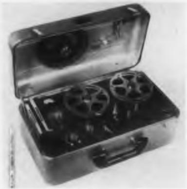
This self-contained tape recorder is housed in a weather-tight aluminum case and it weighs only 19 lb. A VU meter is incorporated to act as a level indicator, and "A" and "B" battery meter. It also simplifies the correct setting of recording
