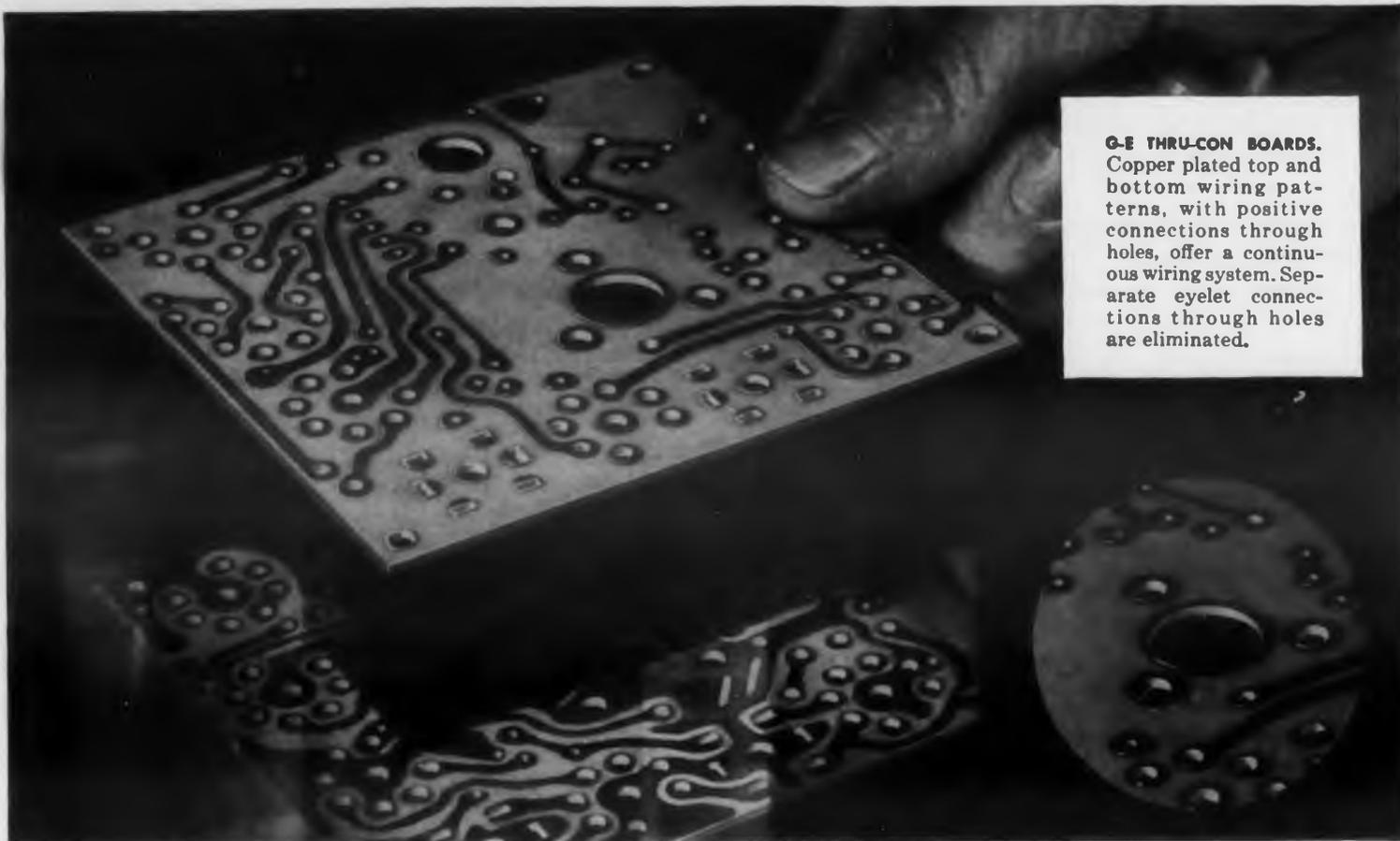
**G-E THRU-CON BOARDS.** Copper plated top and bottom wiring patterns, with positive connections through holes, offer a continuous wiring system. Separate eyelet connections through holes are eliminated.
