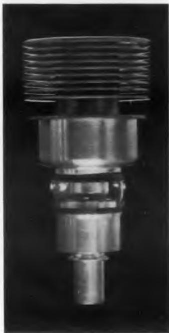
**ML-322** U.H.F. diode for modulation clipper at frequencies to 1500mc. Extremely rugged. Oxide coated disc cathode (also used in ML-381 and ML-2C39A). Convection cooled anode; 15 watts diss. Peak inverse volts: 1800. Peak plate ma: 600. Average plate ma: 100.
