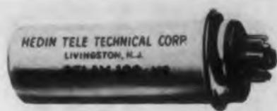
Relay 100 MS incorporates a through wiping effect and has the fast operating speed of 10millisec. Available either hermetically sealed or with dust cover, it is designed for d-c applications in contact combination from spst to dpdt.
