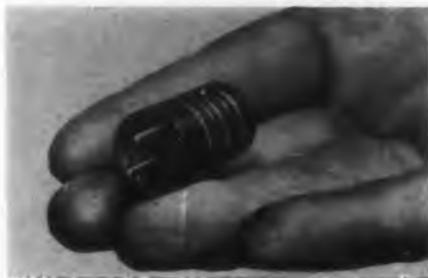
Type 89P "Autocon" one-ended case solid dielectric paper tubular capacitors are designed for printed wiring board assemblies. They are enclosed in a pre-
