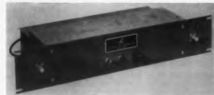
This distributed amplifier, Model 500, is designed for use as an oscilloscope drive, or for general laboratory uses. It has particular application in the field of amplification of narrow pulses, such as are found in the nuclear instrumentation field. Size is 13 1/2" x 2 3/8" x 5 1/4" over-all (approx). The power supply is a separate unit.
