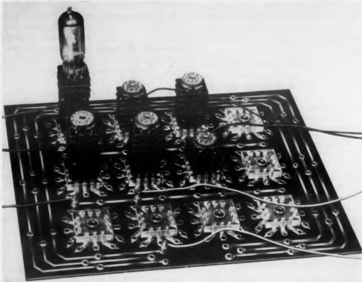
Breadboards such as the one above help the engineer interconnect standard circuit modules into complete electronic subassemblies.
