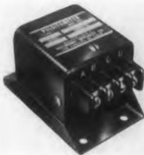
This small, lightweight, dual Pi noise filter for actuator motors consists of four 0.5mfd capacitors and two 0.5mh toroids, and is rated at 2amp 200v d-c. It is only 7/8" x 7/8" x 9/16" in size, and weighs 7/8 oz. The unit brings noise level
