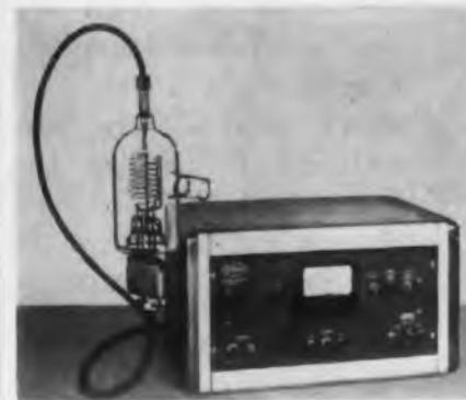
Nos. RG-2 and RG-3 Ionization gage controls measure pressures from 1 micron to  $2 \times 10^{-10}$  mm Hg. High stability and linearity are provided by a new type of circuit using an ion current amplifier
