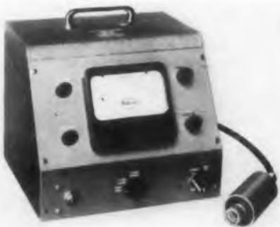
The Model F-2 Power Meter operates over the entire frequency range of d-c to 11,000Mc. Power is measured in three ranges: 0-1-mw, 0-10mw, and 0-100mw. Accuracy of readings
