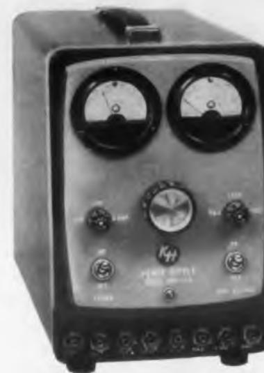
For the most exacting d-c regulation, the Krohn-Hite Model UHR-225 POWER SUPPLY provides unsurpassed performance. It is low priced and compact (7 1/2" wide x 10" high). It has 0.002% regulation and 100 microvolts ripple over the entire operating range (150-500 volts and 0-200 MA). For line voltages between 105 and 125 volts, full rated current can be drawn continuously with a substantial margin of safety. The internal impedance is less
