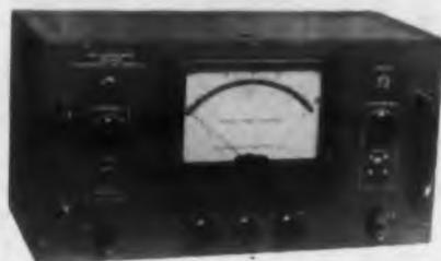
Type 405 Precision Phase Meter has its meter reading independent of both signal amplitude and frequency over wide ranges, 0.3 volt to 120 volts rms and 8 cps to
