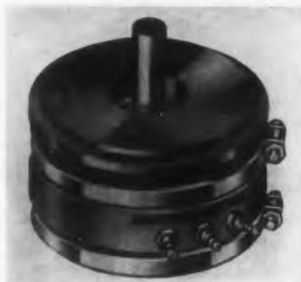
The Series Y "Helipot" precision potentiometer is a single, continuous-rotation component designed for servo or bushing mounting. As many as 14 sections may be ganged on a common shaft during manufacture, with
