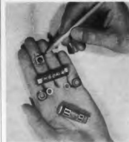
This "wafer cell" is designed to make possible a 30% increase in battery power and life, while eliminating traditional hand operations from cell manufacturing. It consists of a sandwich of artificial manganese dioxide mix between tiny disks
