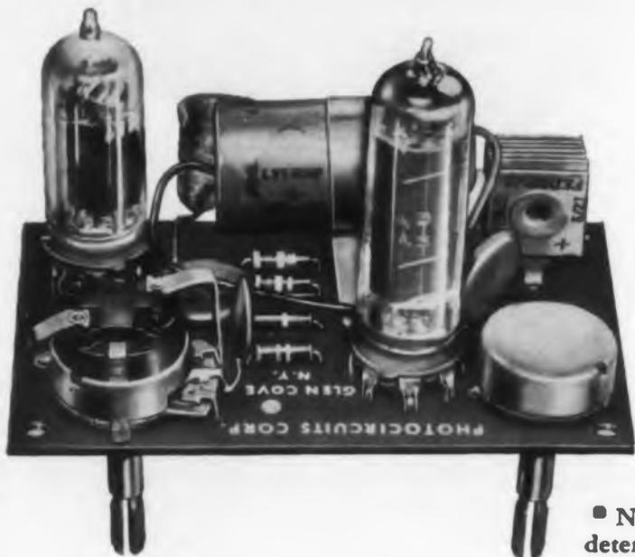
Audio amplifier unit by Photocircuits Corp., Glen Cove, N. Y., using Revere Rolled Printed Circuit Copper.
