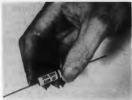
The "Royal Cub" paper-dielectric capacitor combines high temperature and high stability operation with mechanical toughness and long-life characteristics, achieved by the
