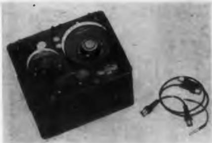
The Type 1606-A Radio - Frequency Bridge retains all the desirable features of this firm's older Type 916-A, and adds several new ones. A new broadband bridge transformer efficiently covers a range from below 400kc to 60Mc. New milled-plate variable air capacitors, which have very low losses, are used as reactance standards. General Radio Co., Dept. ED, 275 Massachusetts Ave., Cambridge 39, Mass.
