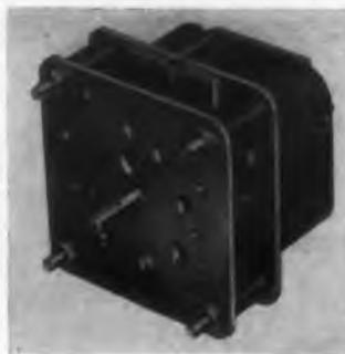
An open-type geared motor designed for overhanging or radial thrust loads, this unit offers ruggedness, quietness, and dependability. It uses double-supported gear shafts running in sintered-bronze bearings, heavy-duty gears
