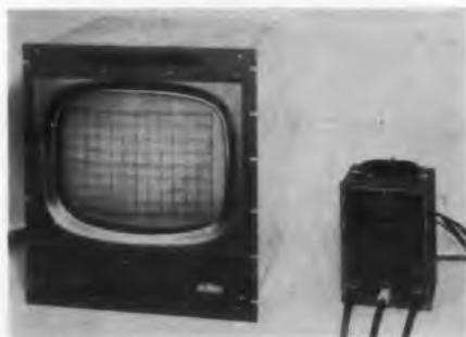
These two new units, 17" and 21" indicators, employ television-type cathode-ray tubes and are designed primarily for use in conjunction with low-frequency, laboratory-type oscil-
