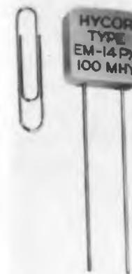
This "Postage Stamp" Toroid Coil configuration was designed specifically for use in printed circuitry. Its tinned No. 20 AWG wire leads are spaced in accordance with the standards recently proposed the RETMA Automation Committee.
