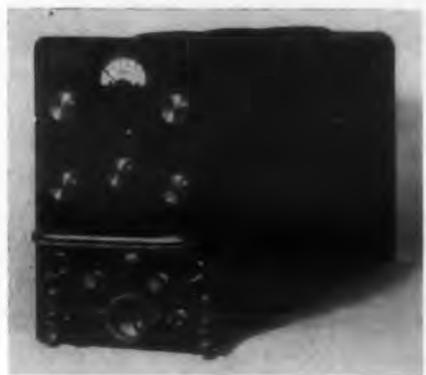
The Model 25 Traveling Wave Tube Amplifier permits 2-4kMc or 4-8kMc operation with two readily interchangeable TW tubes. The gain over both bands is at least 30db, and the maximum power out-
