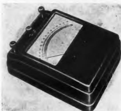
These "AEC" (Allgemeine Elektrizitaets-Gesellschaft) moving-iron instruments are of the 0.2% precision class. Both ammeters and voltmeters are available in a variety of ranges (and in multi-
