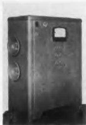
With three-phase 230-250v 60cy input, this portable laboratory power supply transformer unit has two output ranges: 211-640v 31-amp, in 10v steps, and 100-295v 66amp, in 4v steps. Adjustment is by eight fine steps and eight coarse steps with overlap. Taps are changed on three phases simultaneously. It is de-
