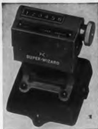
Named "Super-Wizards", these improved electric counters have an average life expectancy of 300 million counts. Rated at 1000cpm, they operate at speeds to 1600cpm with suitable actuation.
