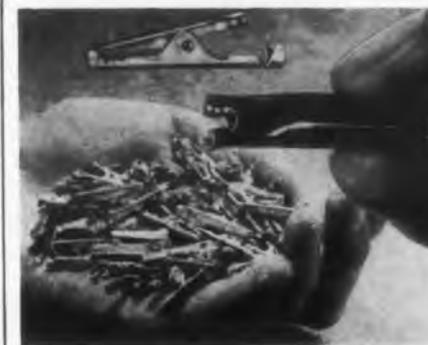
"Mini-gator" clips are only 1-1/16" long, with a nose of 11/64" OD and a weight of 1/20 oz. They are manufactured in both steel (cadmium plated) and solid copper. One piece insulators are
