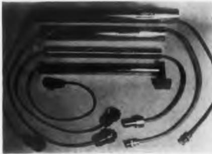
A series of four backward-wave oscillators features electronic tuning across the units' respective frequency ranges. Tuning is accomplished by varying or sweeping a single voltage
