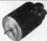
**MODEL 323 ELEVON ACTUATOR** — Develops 1/2 h.p. at 11,200 rpm. 200 V. line-to-line, 3 phase, 4 wire, 400 cycles. Teflon insulated for  $-65^{\circ}\text{F}$ . to  $+160^{\circ}\text{F}$ . operation. Meets MIL M 7969 specifications.
