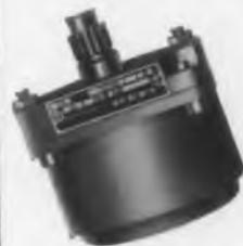
2-phase reversible motors. High torque. Fully enclosed. Self-lubricating. No-load speeds of 27, 54, 167, 333, and 1650 rpm available. Operate from 115-volts, 60-cycles. Numerous variations in pinion, shaft, leadwires, and materials available for special requirements. Prices from \$40.50.
