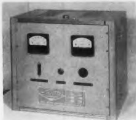
Illustrated is a typical "Sel-Rex Reactronic", a regulated d-c power supply unit for continuous output of 5-amp at 150v. Static regulation is  $\pm 1\%$  from no load to full load.
