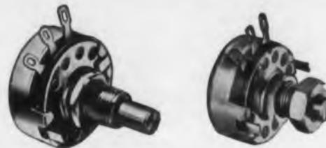
Allen-Bradley Type J molded variable resistors are made in single, dual, and triple unit construction in total resistance values from 50 ohms to 5 megohms. They are rated at 2 watts at 70C ambient. They are outstanding for their low noise characteristics, initially and after use. Metal parts are made of corrosion-resistant materials. Taps can be supplied at 40, 53, and 68% of effective rotation. A Quality product throughout.
