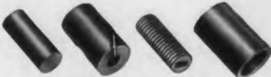
PLAIN CORE HOLLOW CORE THREADED CORE SLEEVE CORE
