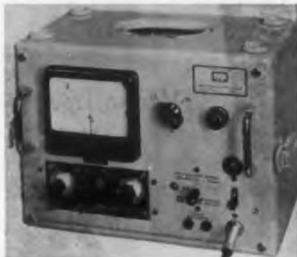
The FT-KZS Tolerance Indicator permits rapid testing of resistors, capacitors, and inductors by comparison with an external standard. Direct readings in per cent are given on a 4" meter with
