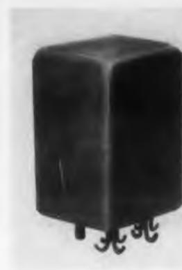
Contacts are silver, rated 2amp 28v d-c, and 115v a-c; 100,000 operations is the life expectancy at rated resistive loads. Operating power is 40mw for dpdt, and 20mw for spdt. The unit contains a high-efficiency double-coil magnetic circuit with a resistance up to 12,000 ohms, with a maximum dissipation of 1w. Size is (approx) 1" x 1" x 2" long. Magnadyne Co., Dept. MS, 84 S. Water St., Port Chester, N. Y.
