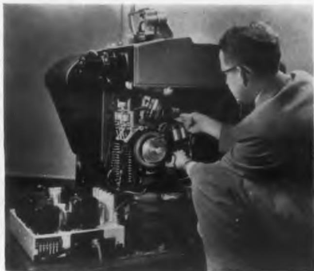
The working parts of an electronically controlled camera that helps prepare directories.
