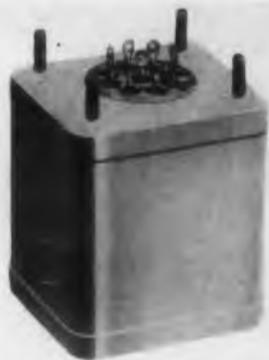
Stock units are available over wide ranges of impedance, power gain, response time, and supply frequency. Toroidally wound reactors are used throughout, and the units are available in hermetically sealed cases or plastic-encapsulated forms.
