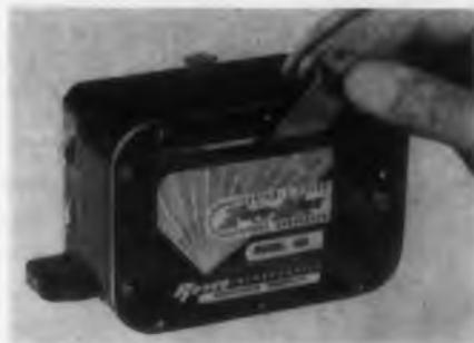
The Model 143 "Zero-Max" infinitely variable speed reducer has a constant torque rating of 30 in-lb throughout its speed range of true zero to 1/4 the input speed (0-450-rpm with an 1800rpm input speed). At about 400-rpm it is rated at 1/3hp. Speed can be changed while running. Heat is not developed at zero speed. It weighs 5-1/4 lb. Reveo, Inc., Dept. ED, 2 E. Franklin Ave., Minneapolis, Minn.
