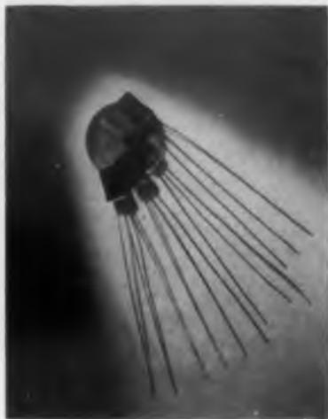
These p-n-p fused junction germanium transistors which are one-quarter to one-third the size of former units have a volume of only 0.0087 cu. in. They are designated types 2N130, 2N131, 2N132 and 2N133. The first three are intended for use in audio or low radio frequency applications; the fourth is a
