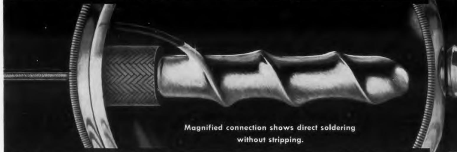
Magnified connection shows direct soldering without stripping.
