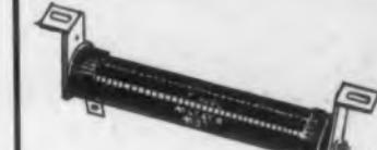
**HIGH-POWER—STYLE R** • 25 to 1,000,000 ohms; ratings from 7- to 115-watts; non-inductive. Standard tolerance ±2% 10 to 1,000,000 ohms. Exceptionally good noise and frequency characteristics. Superior moisture resistance and overload capacity.
