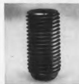
Compare UNBRAKO-recommended tightening torques with those of ordinary socket set screws and you readily see why you can set an UNBRAKO and then forget it. The reasons are simple. UNBRAKOS have deeper sockets, which give you better purchase with the wrench; rounded socket corners, which eliminate the sharp corners where cracks start; fully formed threads, which make them stronger; and knurled cup points, which keep them tight.
