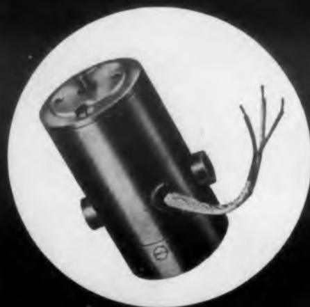
Interchangeable DC and Universal AC motor—1500 Series (1 1/2" diameter). Horsepower: 0.02. Drives coaxial transfer switches and actuators. Series, split-series, shunt or compound windings. 6 to 30 volts D.C. 115 volts, 60 cycle, A.C. Torque up to 2 oz. inch. Brake and speed governor optional.
