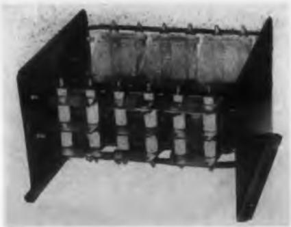
Because the resistance wire is virtually suspended in free air, with no other obstruction to impede the flow of cooling air, the heat dissipating capacity is very high. The construction provides a compact, lightweight unit.
