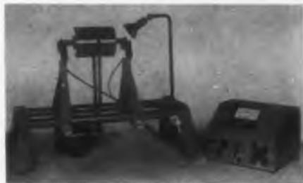
A fully electronic dynamic balancer, Model 5V-6 will handle any rotating body from 4 oz to 100 lb, yet is simple enough that operation can
