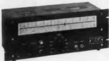
**MODEL 20 DC VOLTMETER** is a servo-actuated, fast, accurate and sensitive instrument. Has large, easy-to-read scale for general laboratory use where ranges from 3 millivolts to 300 volts are desired. For data handling it is furnished with a built-in Coleman digitizer and delivers digital output for operation of printers, typewriters, tape or card punches, etc.
