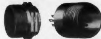
Hermetically sealed connectors... with steel shells and contacts to withstand high pressures. Available in GS (AN type), KH, RKH, U, BFH, TBFH. Insulation is Can-seal glass material, fused under high temperature to shell and contacts... giving true hermetic sealing when soldered or brazed to housing.
