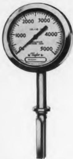
Initially, the hydraulic system used to translate volumetric pressures into the pinion-and-sector gear that controls the dial indicator of the gage, contained a glycerine and water solution. But the viscosity of the solution varied with changing temperatures causing the response time of the gage to vary accordingly.
