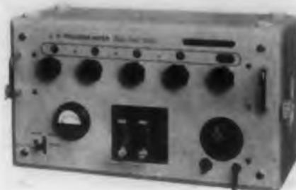
The Type RGV Resistance Precision Meter has a range of 0.01 ohm to 100 megohms. Accuracy is  $\pm 0.1\%$   $\pm 1$  milliohm in the 0.01 ohm to 10 megohm
