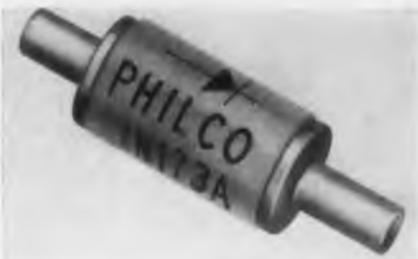
Specifically designed for u-h-f tuners, this mixer diode (1N173A) is made by a special process which results in uniform characteristics for tuner
