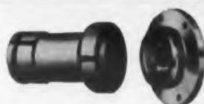
W Waterproof Series... used underwater and on equipment operating in swamps, rivers, lakes, with underground cables—wherever conditions require thoroughly sealed fittings. Exceptionally rugged. AN type inserts. Acme threads on coupling nuts. Special rubber sealing ring. Special heavy duty cable clamp available.
