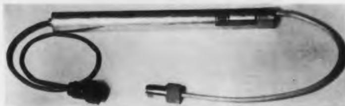
This traveling wave tube features broadband electronically tuned oscillations from 7 to 14kMc, accomplished by the adjustment of a single voltage without any complementary mechanical adjustments. This type of oscillator should find its greatest field of use in swept-signal generators for automatic testing, swept local oscillators, and wide-band transmitter-receiver applications.
