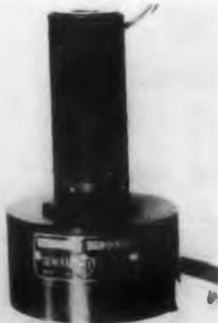
This high-speed precision sampling switch with integral motor and planetary gear reduction is available with 1, 2, or 3 concentric poles, 60 contacts per pole, utilizing a semi-molded contact plate construction for long life and dimensional stability. Connections to each pole are made by wire leads molded into the plate
