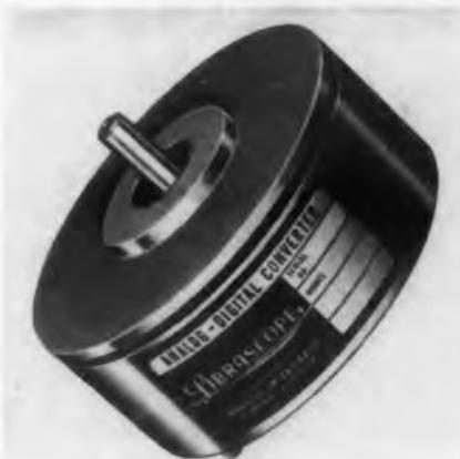
This special shaft - position converter translates the position of an input shaft into the Gray binary-digital code for use in computers and automatic control equipment. A commutator-type code
