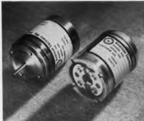
To qualify for the job, the molded parts withstood five room temperature shock tests at 50 "G's" plus constant vibration in the order of 25 "G's" for 4 hours at 600 F. Finally, the potentiometer was subjected to 1050 F for 15 minutes. The terminal blocks molded of Dow Corning 301 Molding Compound were somewhat shrunken and charred, but the brass inserts were still firmly retained. **No. 9**
