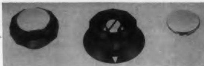
This "Kollet" Knob, with a special locking device for 1/4" shafts, is offered in two types: with and without a skirt. The knobs eliminate the use of set-screws by utilizing a collet-type locking device which permits tightening with screwdriver, coin or socket wrench, from the front. The knob's metal faceplate snaps in to complete the design and cover the locking device. Cambridge Thermionic Corp., Dept. ED, 445 Concord Ave., Cambridge 38, Mass.
