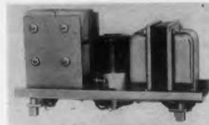
Designed for operating control equipment on unregulated 28v d-c, this power supply is built for continuous duty in laboratory or
