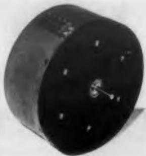
A comparison standard rotation-to-voltage transducer for basic measurement, potentiometer testing and calibration, and analog multiplication, this potentiometer features linearities to 0.002%.
