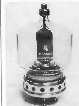
This transmitting triode, the PL-6569, is designed specifically for use as a medium-power grounded-grid r-f amplifier. It combines high perveance with a high amplification factor, to give unusually high power gain in grounded-grid service.
