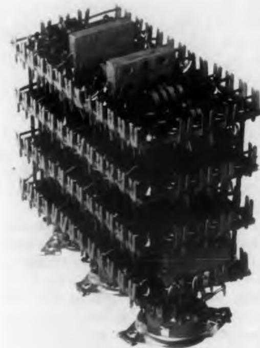
In this type of turret socket, the layers are separated by spacers and long screws.
