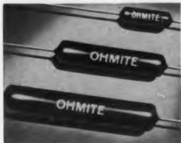
This line of small, power - type wire-wound resistors has steatite cores and axial leads. A special-formula, vitreous-enamel coating is also employed. The resistance wire and terminal lead
