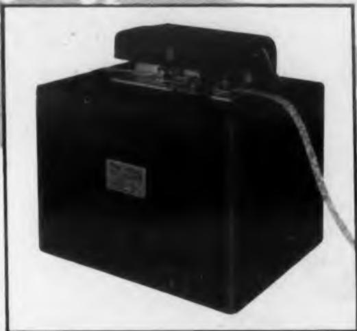
The Ferranti High Speed Tape Reader accelerates to full speed within 5 milliseconds and stops within 3 milliseconds. It has been in use at leading computer installations for over two years and has achieved a sound reputation for simplicity and reliability in regular operation.
