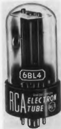
The half-wave vacuum rectifier tube 6BL4 is of the glass-octal type and is particularly suited for use as a damper diode in color TV receivers. Rated to withstand a maximum peak inverse plate voltage of 4500v (absolute), the 6BL4 can supply a maximum peak plate current of 1200ma, and a maximum d-c plate current of 200ma. In addition, negative peak pulses between heater and cathode of as much as 4500v including a d-c component of as much as 900v may
