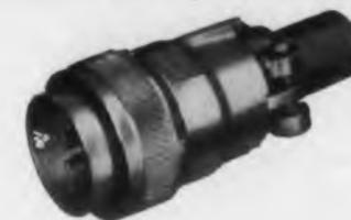
AN-E Series... environment resisting. Replaces "old" AN-M. Meets Specification MIL-C-5015B. Resilient inserts. Completely sealed from cable to cable. Integral clamp and bushing. Grounding lugs. Interfacial sealing with grommet and grommet follower. Available as Interim AN-M with ferrule in place of grommet follower.
