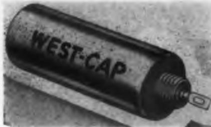
Available in MIL-C-25 CP11 types with axial wire leads, this vertical mounting type capacitor is designed with critical requirements in high vibration and weight. Utilizing deep drawn cases, the unit eliminates a weakness common to capacitors of this style where the solder joint between the threaded bushing and the case is used as a mechanical connection. San Fernando Electric Mfg. Co., Dept. ED, 1509 First St., San Fernando, Calif.
