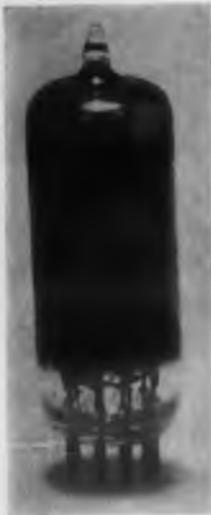
The 6BA8, a miniature, 9-pin medium-mu triode and sharp cutoff pentode, is intended for service in TV receivers employing a series heater string. The pentode section has a plate dissipation rate of 3.25w and is designed to serve as a video amplifier. The triode section has a mu of 18 and is suitable for applications where a low-mu triode is desirable, such as sync amplifiers, etc.
