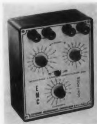
The "Resistance-Capacity Substitution Box", Model 900, is produced in two forms: wired and tested, and in an easy-to-assemble kit. It provides, within 10% accuracy, 36 standard RETMA resistor values from 15 ohms to 10 meg-ohms, and 18 standard RETMA capacitance values from 0.001 to 0.22mfd. Electronic Measurements
