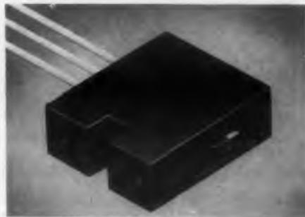
The Model MH 10-A is designed for low-cost recording or reading on magnetic drums in memory systems of digital computers. It features high
