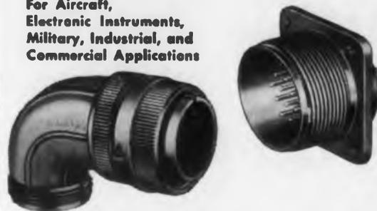
Standard AN-A, AN-B, AN-C... meet Specification MIL-C-5015B. Plastic inserts. 15 diameters, 260 insert layouts, 6 shell styles. AN3100 to AN3108 with all accessories. Interchangeability an outstanding feature. Many type assemblies directly available through distributors.
