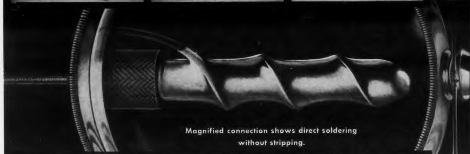
Magnified connection shows direct soldering
