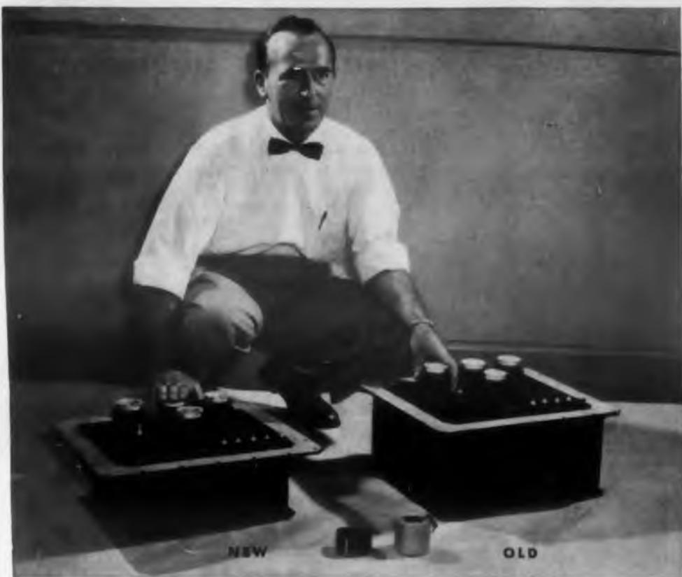
WEIGHT OF A TYPICAL POWER SUPPLY WAS CUT 61 LBS. when redesigned for smaller embedded-layer coil. New and old coils in foreground illustrate typical size reduction now possible.
