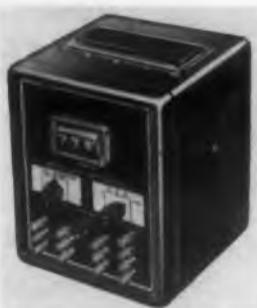
Useful in telemetering, gaging, and quality-control applications, the Model 625 "Digital Ratiometer" provides a rapid three-digit indication of the ratio between two related d-c voltages, accurate to  $\pm 5$  parts in 1000 ( $\pm 0.5\%$  of full scale). The complete indication is automatic, and the average reading consumes only 1 to 2sec. Inputs may vary slowly, because internal balancing is continuous.
