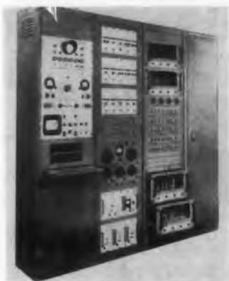
"Servomation" Building Blocks are an array of electro-mechanical general purpose analog computer components. Various component combinations provide means for industrial production control, problem solving for both equations and control system design, experiments, and data processing.
