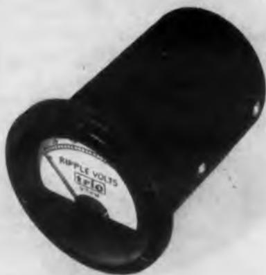
Basic sensitivity is 10MV rms, but it has a scaleplate with 2 ranges, 0-1 & 0-2.5, labeled Ripple Volts. An input resistor chain provides appropriate meter ranges for all the predicted ripple levels and is mounted right on one deck of an external selector switch while the second deck of the switch holds the 11 leads from the power supplies to be tested.
