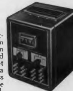
Measures ratio of two DC voltages where one is derived from the other. Ratio is displayed on a three digit servo-positioned counter. Provides a discreet indication of one part in a thousand. Slewing time is less than 4 1/2 seconds full scale. The response is critically damped.
