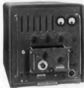
**-hp- 524B Electronic Counter with 525/526 series Plug-Ins.** Revolutionary all-purpose, direct-reading counter. Buy basic counter, plug-ins giving measuring coverage you need now. Later add other inexpensive plug-ins to double, triple counter's usefulness. Basic counter range: Frequency 10 cps to 10 MC, period 0 cps to 10 KC, stability 1/1,000,000. *-hp-* 524B, \$2,150.00A.
