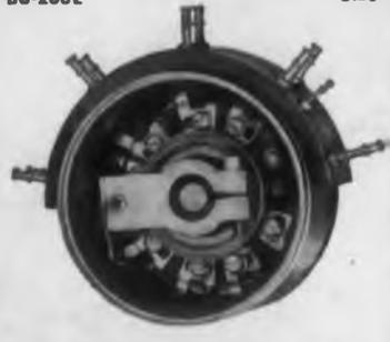
**2" Ball Bearing**— $\frac{1}{2}$  oz. torque per section. Improved linearity. Minimized backlash between ganged sections. Provision for mounting external resistors directly on terminal board. Easily adjusted taps.
