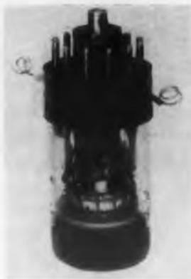
This "Dekatron" cold cathode counting tube, the GS12D, is designed for industrial and scientific counting applications. It is a 12-cathode tube, with all 12 cathodes brought out to pins on the base. It has a 13-pin base, plus extra flying leads. The counting scale of 12 adds to the value of this device in studies
