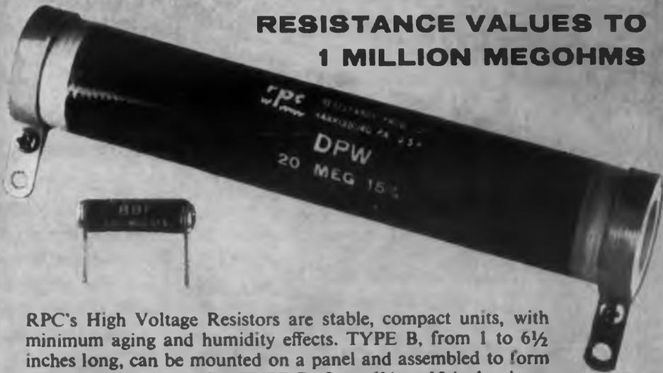
RPC's High Voltage Resistors are stable, compact units, with minimum aging and humidity effects. TYPE B, from 1 to 6½ inches long, can be mounted on a panel and assembled to form tapped or matched pairs. TYPE D, from 6½ to 18 inches long, can be supplied with silver bands, terminal lugs or ferrules.
