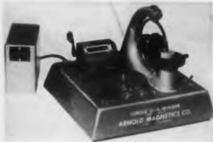
This portable toroidal coil winder is designed for both laboratory and production. It features quick set up and quick wire change. Any of three winding
