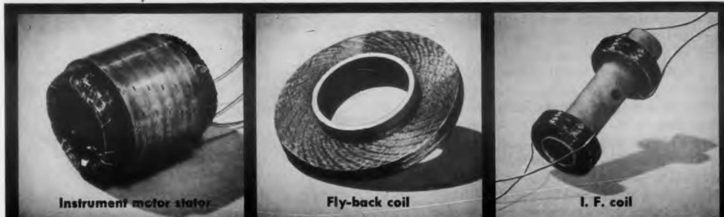
Instrument motor stator
