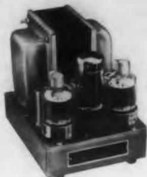
This power supply is designed for general laboratory use or for inclusion in new or existing equipment. The entire compact assembly, including five tubes and rectifier, is mounted on a chassis 7-1/4" x 5-1/2" x 1-3/4" deep. It may be incorporated readily into complete-equipment by removing the bottom plate and fastening the assembly directly to equipment chassis.
