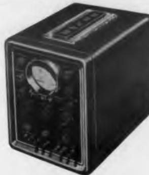
The general purpose scope that gives you most for your dollar... has flat face CRT for usable trace edge to edge. It combines laboratory accuracy with ruggedness and compactness that makes it ideal for field service...
