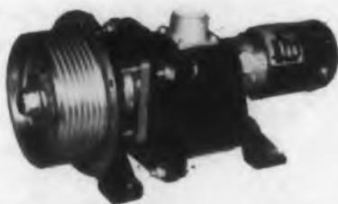
The Series 171 consists basically of a continuous-duty motor driving two counter-rotating magnetic power clutches and gear reduction from the clutches to the output shaft. Its low-inertia factor is due to the magnetic powder clutches. Since the motor runs continuously, it is necessary to overcome only the inertia of the clutch and gearing during acceleration. The clutch has a torque-to-inertia ratio of 440,000-rad/sec<sup>2</sup> and requires less than 1w to produce full output torque.
