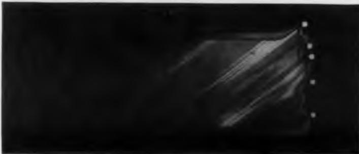
Microscopic views of the foil edge show it when just slit (above). If anodized, points of possible low-voltage breakdown would be formed (white dots).
