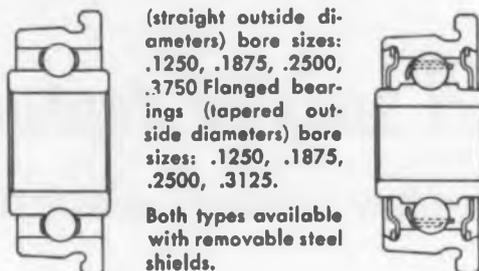
(straight outside diameters) bore sizes: .1250, .1875, .2500, .3750 Flanged bearings (tapered outside diameters) bore sizes: .1250, .1875, .2500, .3125.
