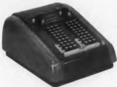
**MODEL 40 KEYBOARD** provides a convenient means for plotting large amounts of tabular data in point-curve form. Self-contained voltage source together with full three column keyboard in both X and Y axes; unit plugs directly into MODEL 2 AUTOGRAF.
