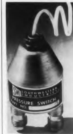
A series of miniaturized, vibration-resistant, differential and gage pressure switches for aircraft and missile systems applications has been developed by this firm. Weighing approximately 1/3 lb, they operate in inert gases and fluids, engine and hydraulic oils, and aromatic fuels, and they are designed to withstand vibration up to 35g. Small and compact, they allow installation in small areas difficult to get at.
