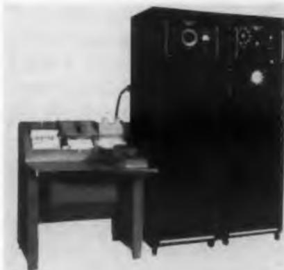
Epsco System No. 177 makes use of magnetic techniques to automatically punch on IBM cards data arriving asynchronously from as many as 10 separate sources. Data consist of time interval measurements
