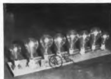
Typical rugged life test using a series of 1000 watt lamps causing the relay to operate under a load 10 times more severe than normal.
