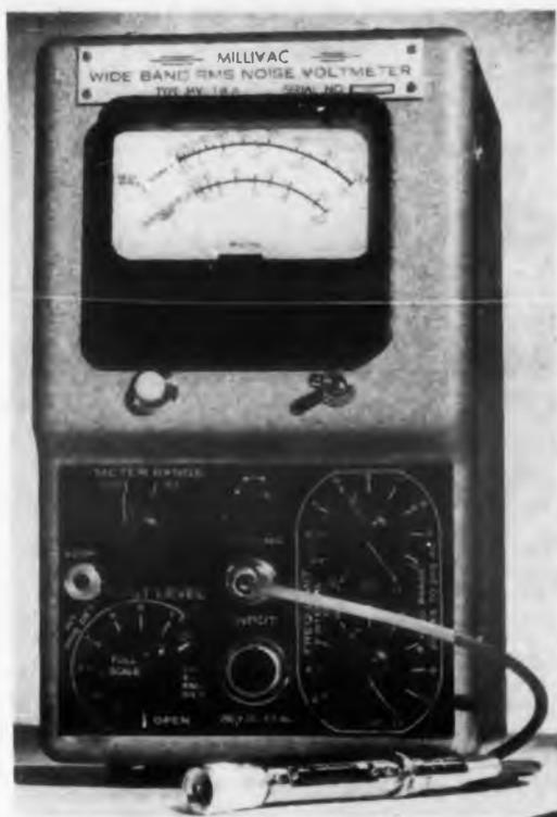
lector switch. For noise measurements above 200kc, special capacitor-divider probes are provided. No bandpass limiting is provided above 200kc since most amplifiers in this range are narrow band types.
