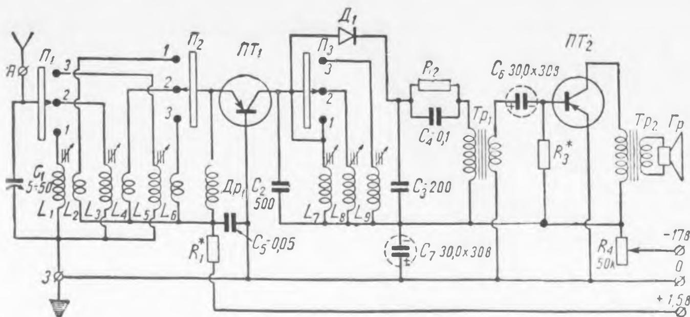
Resistor  $R_2$  and capacitor  $C_4$  equalize the load resistance of the detector for alternating and direct current, which is necessary when the diode is connected to a transformer because of its low d-c resistance. Resistor  $R_2$  serves to increase the d-c resistance of the circuit, while capacitor  $C_4$ , shunting resistance  $R_2$ , passes a-c.
