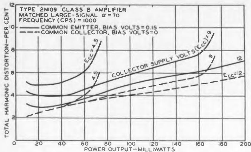
Fig. 7. The common-emitter circuit has less distortion under each operating point.
