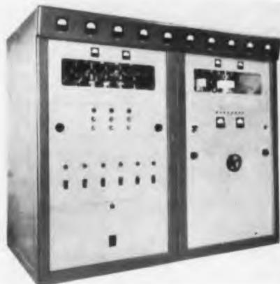
The Electronic Power Supply, Model PP-30-A, is for sine-wave, complex-wave, and flight - simulation vibration testing of airplane and missile components. It will continuously deliver 30,000w into a matched load without overheat-
