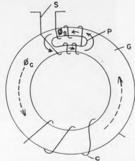
Fig. 1. Shape of basic Magnistor.
