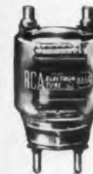
RCA-833-A . . . improved version of the 833 originally developed by RCA more than 15 years ago. The outstanding and continuing popularity of this tube is typical of the many time-proved transmitting, receiving, and special-purpose types originated, developed, and sponsored by RCA. The RCA-833-A is designed for use as an rf power amplifier, oscillator, or class B modulator. It has a maximum plate dissipation rating of 450 watts under ICAS operating conditions with forced-air cooling.
