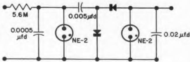
Fig. 2. Schematic of the standard bias supply.
