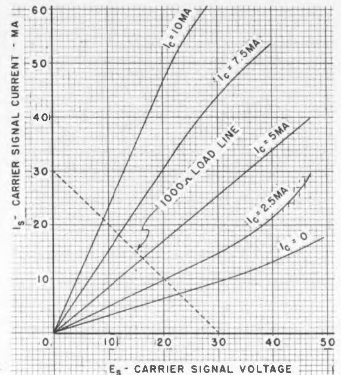
Fig. 8. Characteristic of type ATC1.
