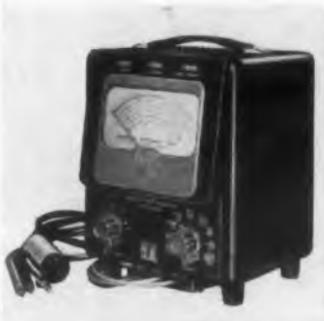
Designated as the type 800B, this multipurpose test instrument is the newest version of the type 800 Vacuum Tube Voltmeter. It is for use at frequencies as high as 700Mc as an a-c voltmeter with full scale ranges from 0.1 to 300v. As a d-c voltmeter, it has
