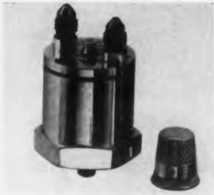
Accelerometers and pressure-measuring pickups that will operate under temperatures as high as 2200°F are now available from this firm.
