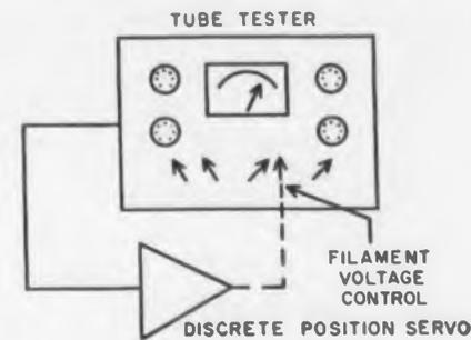
Fig. 3. Tube filaments can not be accidentally overloaded in this unusual tube tester.
