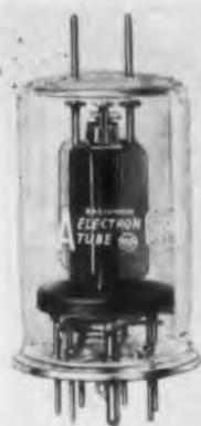
The 5894 is a small, sturdy, twin-beam power tube intended primarily for use as a push-pull r-f power amplifier or as a frequency tripler in fixed and mobile equipment operating in the uhf range between 450 and 470Mc. It has a maximum plate-dissipation rating of 40w under CCS conditions. Under these conditions in class C telegraphy and frequency-modulated amplifier service at 470-
