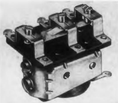
This small, sensitive spdt relay, the "SO" type, occupies only 1-1/8" x 1-7/32" x 1-1/4" and weighs 1-1/2 oz. It is set at the factory to operate on 10mw. The user can adjust it down to 2mw, or any de-
