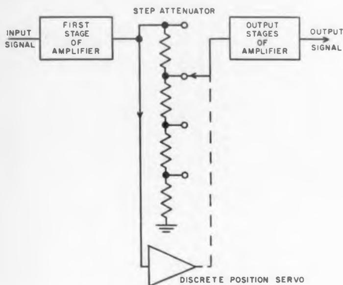
Fig. 11. An automatic-gain-control circuit.
