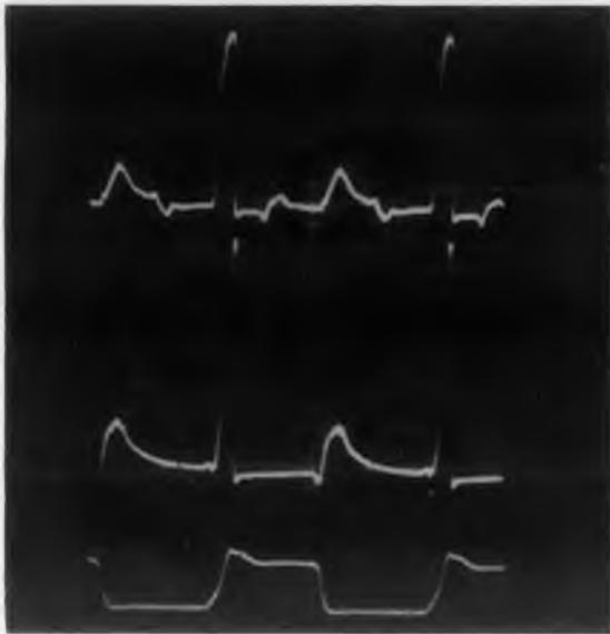
Fig. 6. Oscilloscope shows gated pulse, center, for gating current, bottom. Top trace output is for phase-shifted gate.
