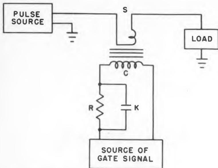
Fig. 4. GTP2 gating circuit: pulses  $1\mu\text{sec}$ , 30v from 200 ohms; gate 40ma in  $1\mu\text{sec}$ .
