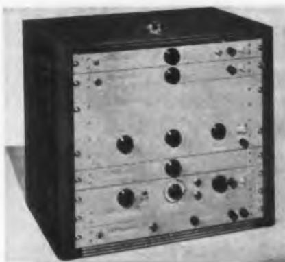
The B-4 Time Measuring System will measure short time intervals to an accuracy of  $\pm 2$ -milli-sec. It is particularly designed to measure the delay time of delay lines and networks and the rise time, fall time, and
