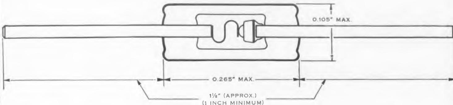
**FEATURES**—High temperature operation . . . extremely high back resistance . . . very sharp back voltage breakdown . . . one-piece, fusion-sealed glass body . . . axial leads for easy mounting . . . subminiature size . . . exceptionally stable characteristics.
