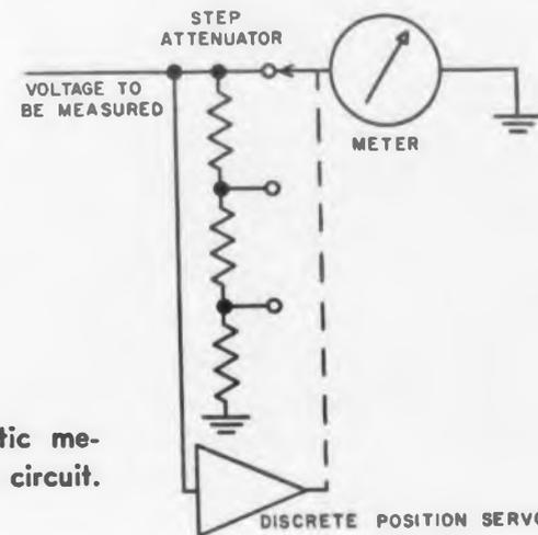
Fig. 4. An automatic meter range switching circuit.
