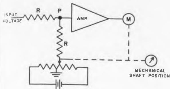
Fig. 1. The conventional servomechanism.
