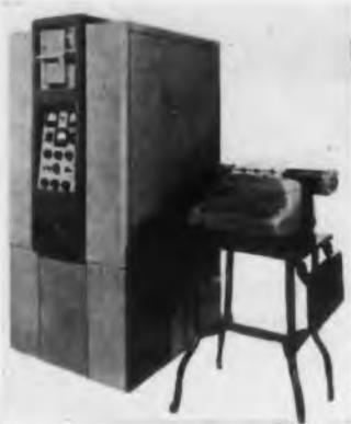
This high-performance moderately-priced electronic computer is capable of solving the lengthy and complex problems of research and engineering organizations. It incorporates an improved two-address command structure which permits greatly increased versatility. The commands provide for addition, subtraction, multiplication, and division, as well as branching and other logical operations.
