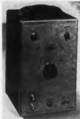
The Model 542 R-F Crystal Calibrator, a compact, portable source of harmonics of 1Mc, 100kc, and 10kc, utilizes signals from WWV to assure a high order of accuracy. Designed especially for frequency measurement or for the calibration of receivers and transmitters, it is also particularly useful as a marker source for panoramic presentations.
