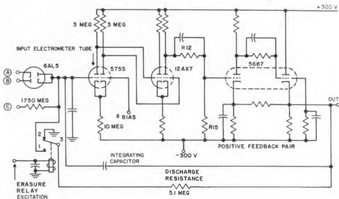
Point A is the negative input, point B is the positive input, and point C is the high impedance input in this circuit of the amplifier.
