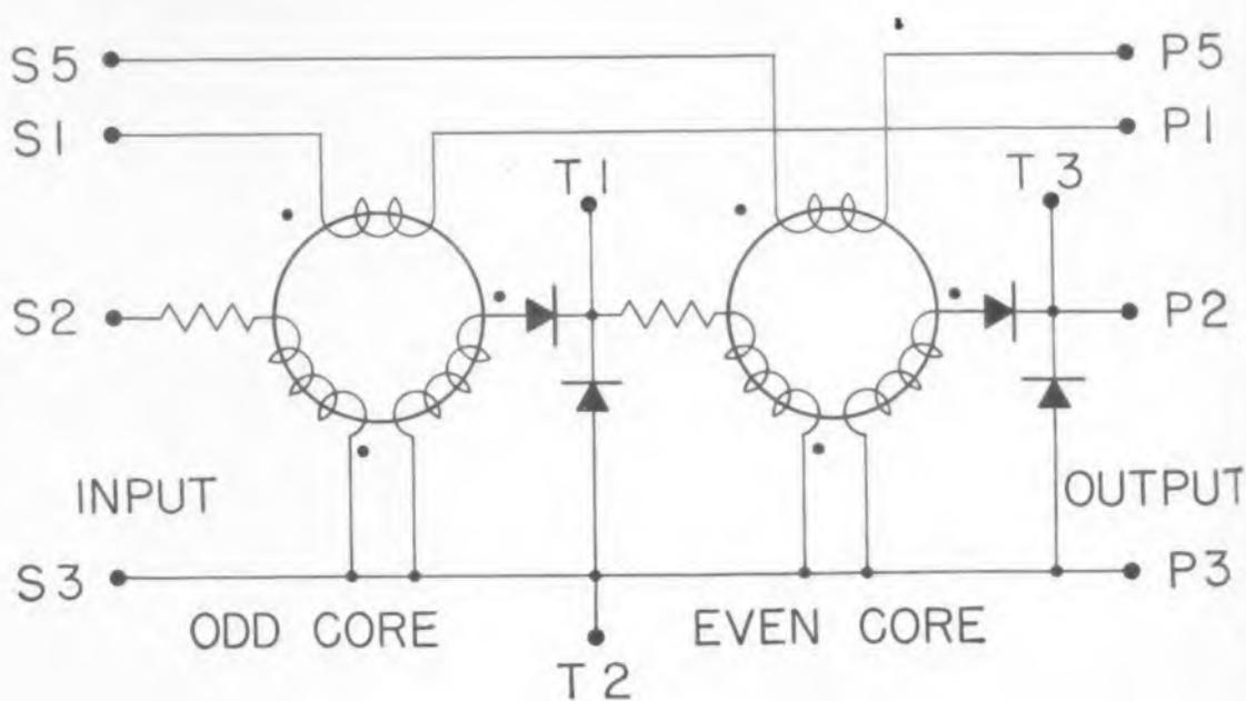
Each unit contains two nickel-iron cores and four diodes; operates from 0 to 20 kc.
