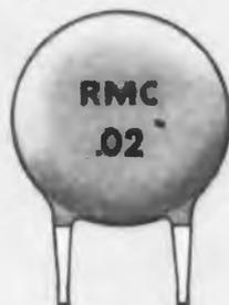
The exclusive wedge design of the leads on these DISCAPS lock them in place on printed circuit assemblies prior to the soldering operation. "Wedg-Loc" DISCAPS are available in capacities between 2 MMF and 20,000 MMF in TC, by-pass and stable capacity types. Suggested hole size is an .062 square.
