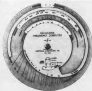
Problems involving frequency, inductance, and capacity are quickly solved with the "Calculaide Frequency Computer". It correlates, in one setting, the natural frequency and wave length of a circuit comprising
