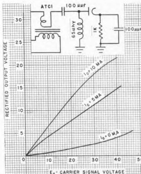
Fig. 14. *ATC1* Magnistor characteristics with a single diode rectifier.
