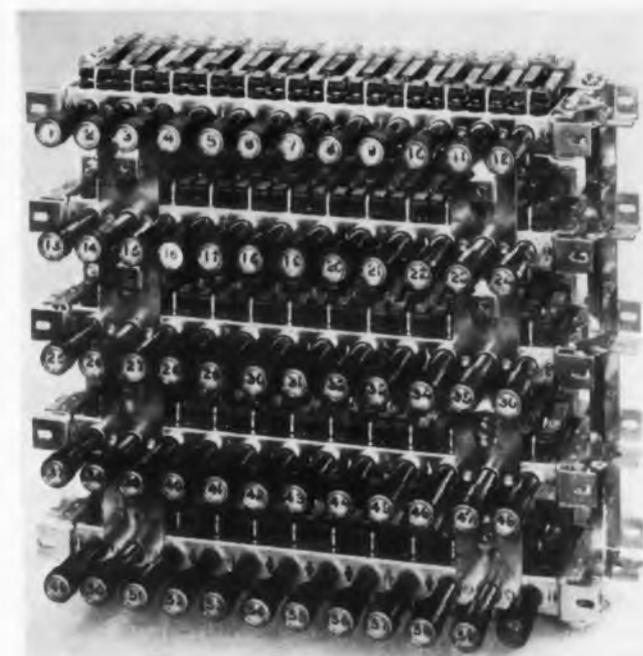
The above bank of 60 illuminated pushbutton switches can perform many functions.
