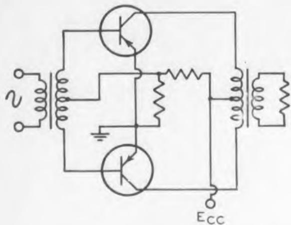
Fig. 1. Both the common-emitter Class B circuit at the top and the common-collector circuit at the bottom have base input.
