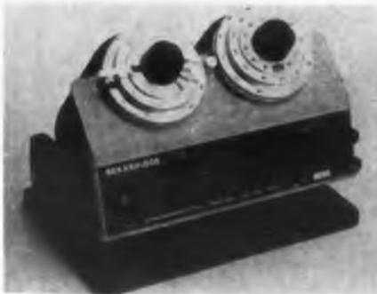
The "Dekabridge" Model 210 Wheatstone Bridge Circuit is designed for easy operation with increased operating speed and improved accuracy. A dual set "Dekadials" provides
