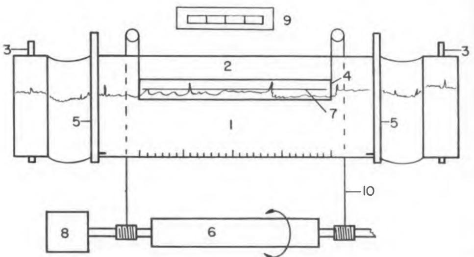
Oscillogram 1, held taut by rods 5, passes over ground-glass screen 2 as spools 3 are rolled. Cable 10 connects cylinder 6 to read head 4. As cylinder is revolved to position read line 7, shaft digitizer 8 converts measured amplitude to a numerical value. Result appears on light bank 9.
