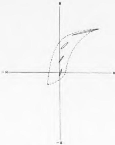
Fig. 3. Displaced hysteresis loops.
