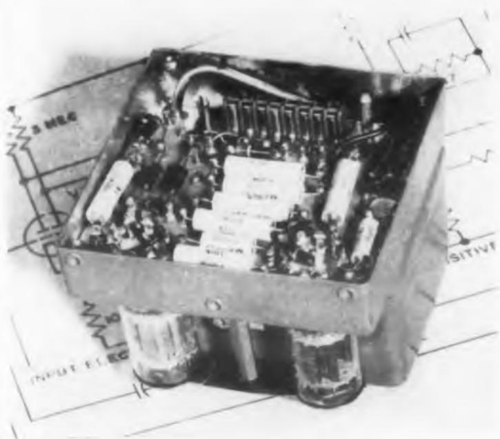
**I**NTEGRATION of video, narrow pulses, and intermittently sampled data and storage of these inputs are the functions of the Type 40 Intergrating Amplifier. This valuable analog computer element has a drift time constant in excess of 40hr. A variety of input and output connections are possible because of the numerous circuit points available. It is also shown on the cover.
