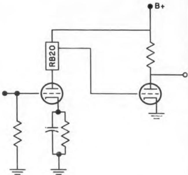
Fig. 3. The unit acts like a coupling battery in this amplifier with low-frequency response.
