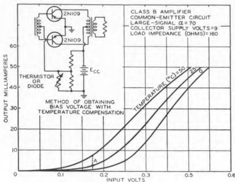
Fig. 9. Temperature characteristics for the circuit enclosed in the chart.
