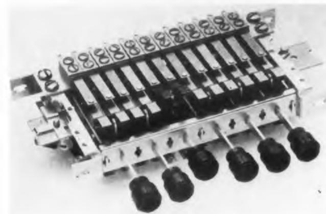
A six-switch frame of the interlock type.
