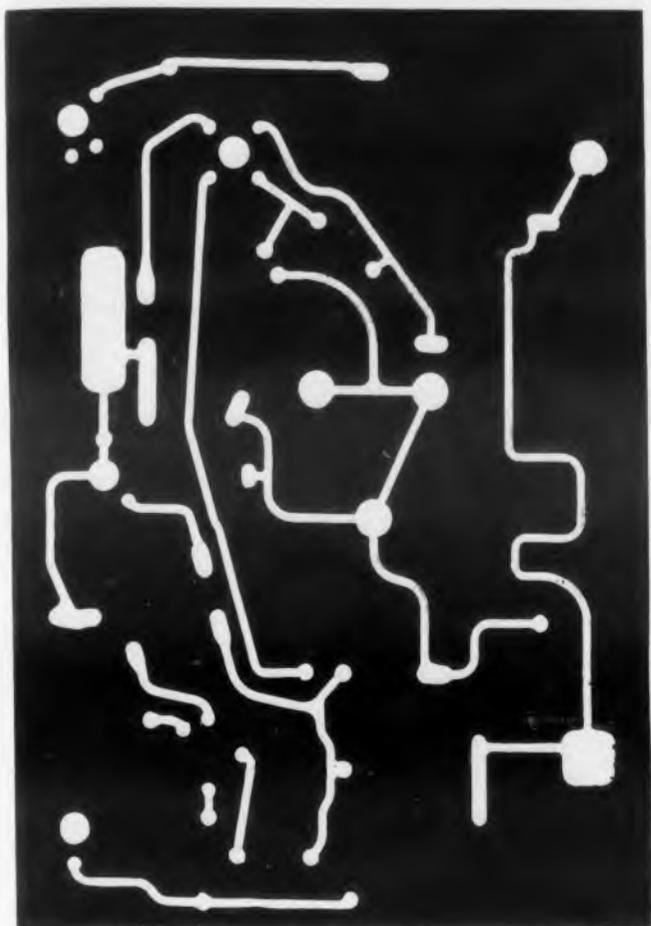
Example of a stamped-out printed circuit. The copper foil is flush with the surface of the RM 2035.
