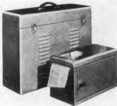
This direct-writing oscillograph, the Type P Portable "Dynograph", is housed in two carrying cases, and it can be set up for use in seconds. The recorder provides
