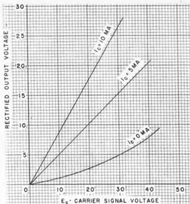
Fig. 12. Rectified characteristics of type *ATC1T*.
