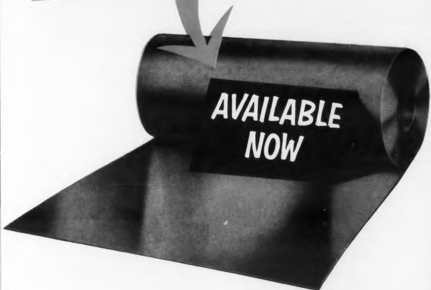
No longer need the lack of material deter you from switching to printed circuitry. Revere Rolled Printed Circuit Copper is now available to laminators in standard coils of 350 lbs. in widths up to 38", and in .0015" and .0027" gauges weighing approximately 1 oz. and 2 oz. per square foot.
