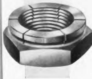
Regular FLEXLOCs are one-piece, all-metal, standard height nuts that lock securely, even under extreme vibration. Thin nuts have the same one-piece, all-metal construction and the same positive locking principle, but these nuts are approximately 30% thinner. Your FLEXLOC industrial distributor stocks both types: regular FLEXLOCs in sizes from #4 to 2"; thin FLEXLOCs in sizes from #6 to 1½". Ask him for catalog information and samples. Or write STANDARD PRESSED STEEL Co., Jenkintown 12, Pa.
