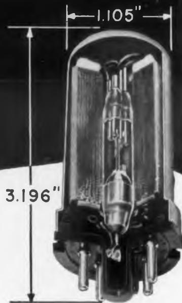
● Cutaway view of HG Relay showing how wick action keeps the mercury at the contacting surfaces continuously replenished.
