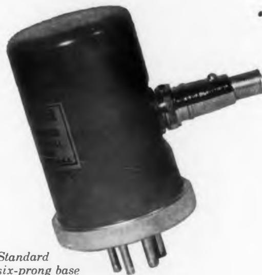
Standard six-prong base with side connection for driving coil.
