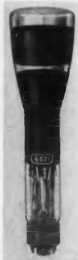
The 6571 is a 3" storage tube designed primarily for use in binary-digital computer systems. It is of the single-beam type, utilizes electrostatic focus and deflection, has its storage surface on the inner surface of the faceplate, and requires an external signal-output electrode shaped to conform to and placed in contact with the entire area of the faceplate. Redistribution writing and capacitance-discharge reading are employed.
