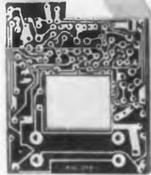
This 12-ounce radio was made possible mainly through the use of printed circuits and transistors!
