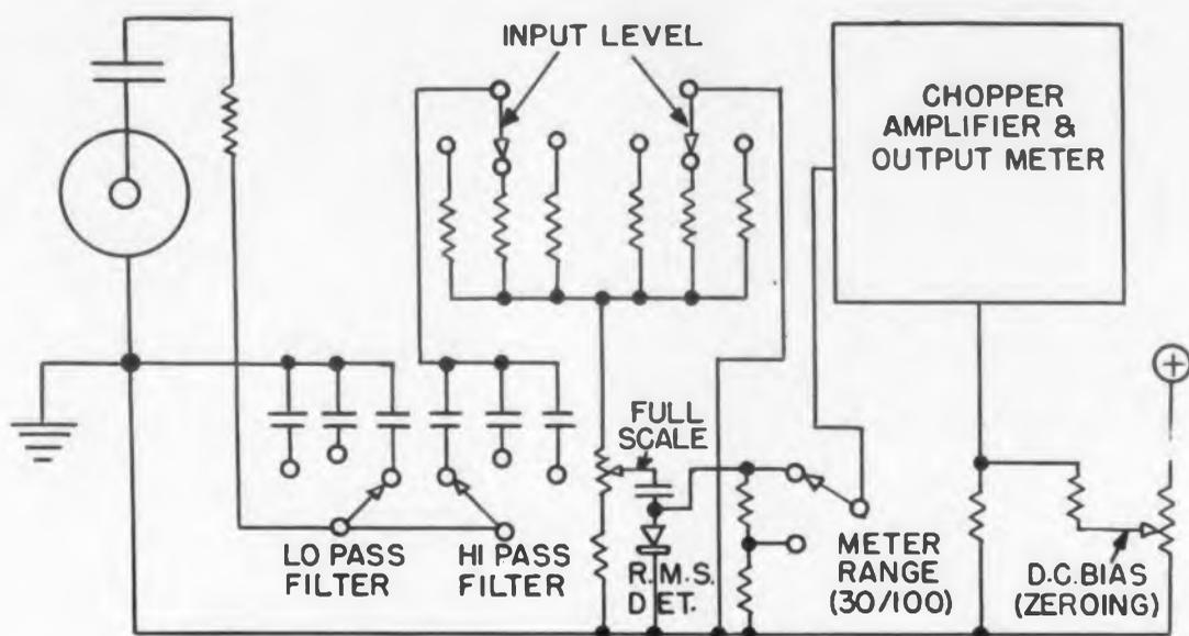
Simplified block diagram of Noise Voltmeter.
