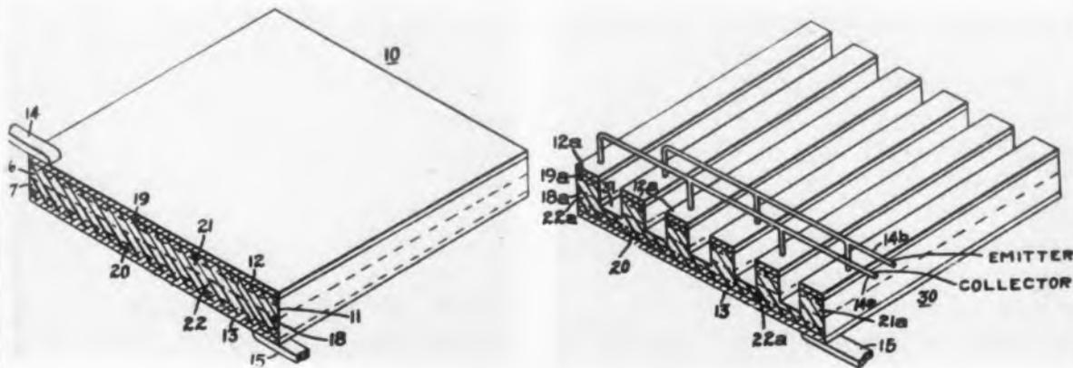
Cross-sections of a rectifier (left) and transistor (right) made by the new process.
