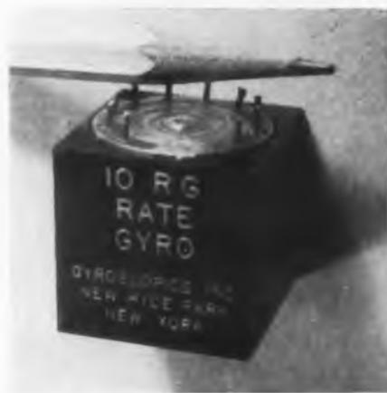
This cubic inch rate gyro weighs 1-1/4 oz. Because of its "floated gimbal" construction, it has excellent shock and vibration resistance. The unit is hermetically sealed with a damping ratio of  $0.7 \pm 0.4$  over temperature range of  $-55$  to  $75^\circ\text{C}$ . Gyro uses 3w of 400cy power. It is capable of measuring very low angular rates. Gyroscopes, Inc., Dept. ED, 15 Birch Drive, Huntington Station, L. I., N. Y. *This product will be displayed at the Wescon Show, Booth 1711-1712.*
