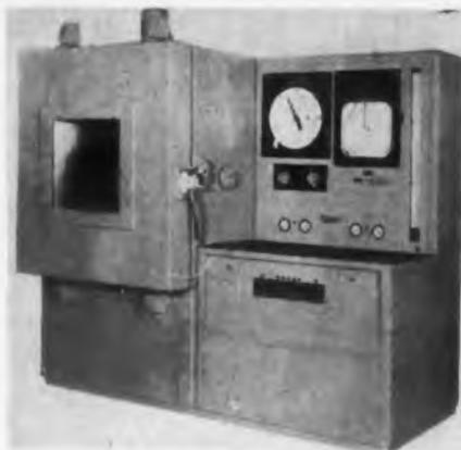
The Model FH-8-2-2 Environmental Test Chamber provides rapid heating of test space. Temperature range is +250 to -100°F, and altitude range is 0 to 100,000' (with up to 150,000' available on special order). The refrigeration system features the "Freon 13—Freon 22" cascade arrangement.
