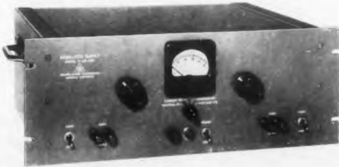
The D50-.05B unit is a dual-output, high-precision regulated power supply for laboratories. It offers wide application as a low-voltage, low-current supply for instrumentation groups. Output is 0-50v at 50ma per side.
