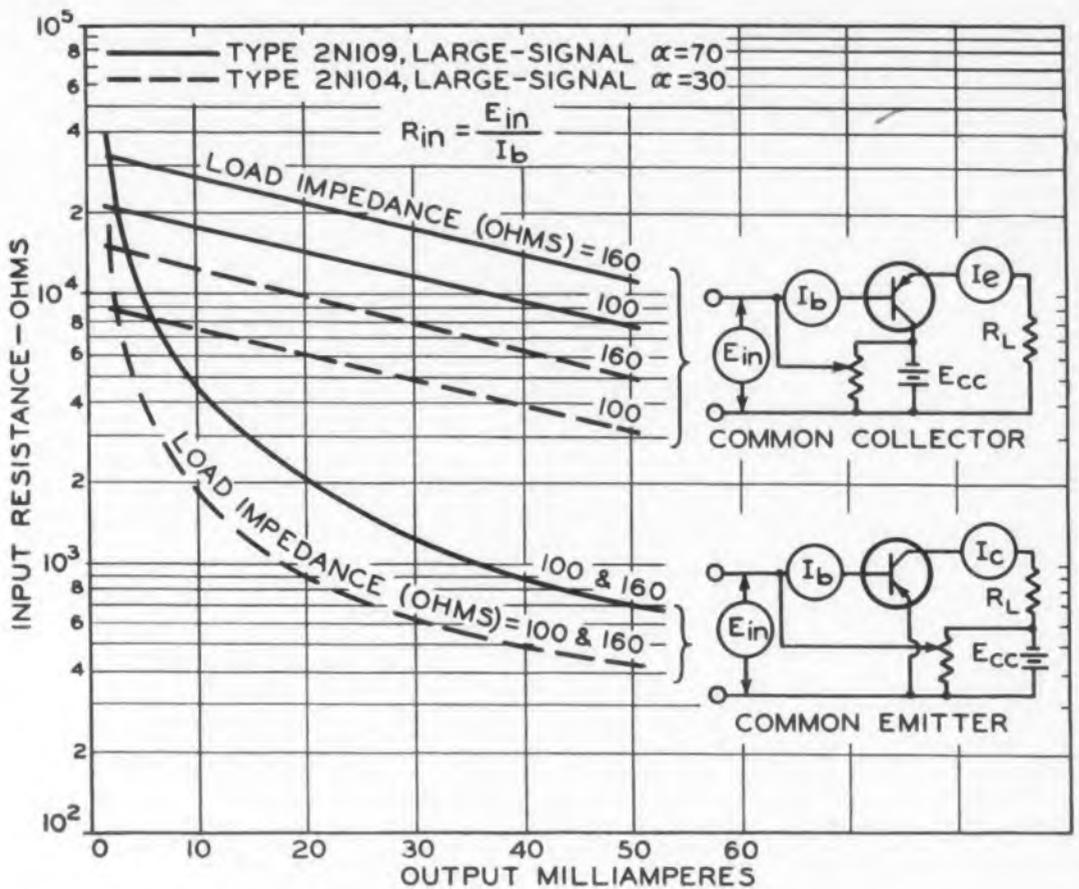
Fig. 3. Input resistance vs. output current for two types of transistors in both common-collector and common-emitter circuits.
