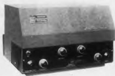
In this combination precision marker generator and pulse generator, all outputs are locked together to provide jitter-free synchronization of output
