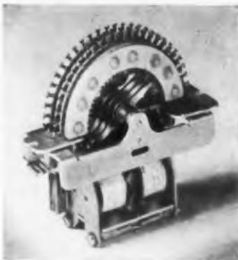
The flexibility of forward and reverse stepping at the operator's choice or by automatic cycling is now obtainable in a compact unit—the G. E. C. two-way stepping selector. Each of these units can replace several conventional one-way stepping relays, thus adding efficiency and versatility to circuit designs.
