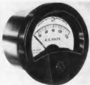
These a-c "Ruggedized" Instruments are shock-proof, vibration-proof, and moisture-proof. Available in 2-1/2" and 3-1/2" hermetically sealed cases, they conform to MIL-M-10304 (Sig. C).
