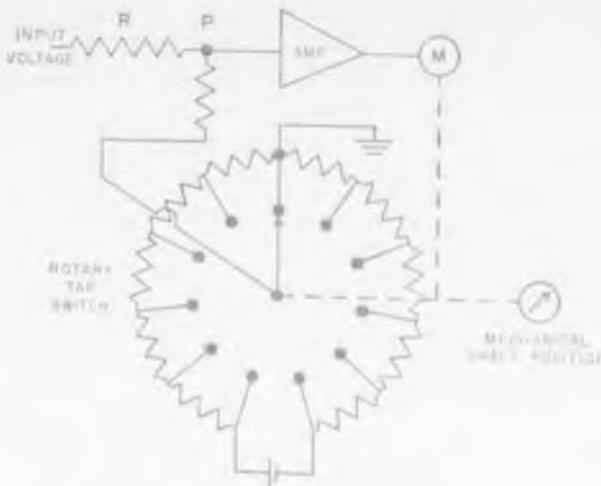
Fig. 2. The discrete-position servomechanism.
