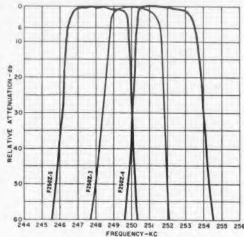
**F250Z** For single sideband signals at a carrier frequency of 250 kc. Bandwidths of 2.7 and 3.2 kc at 6 db attenuation. Transmission loss, 10 db.
