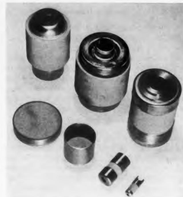
Typical examples of ceramic-to-metal bonding.
