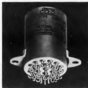
Magnetically held and electrically reset, this latching relay is hermetically sealed in an enclosure of only 1" diam x 1-9/16" long (excluding terminals). It is available in 2, 4, and 6-pole double-throw contact arrangements and is designed to
