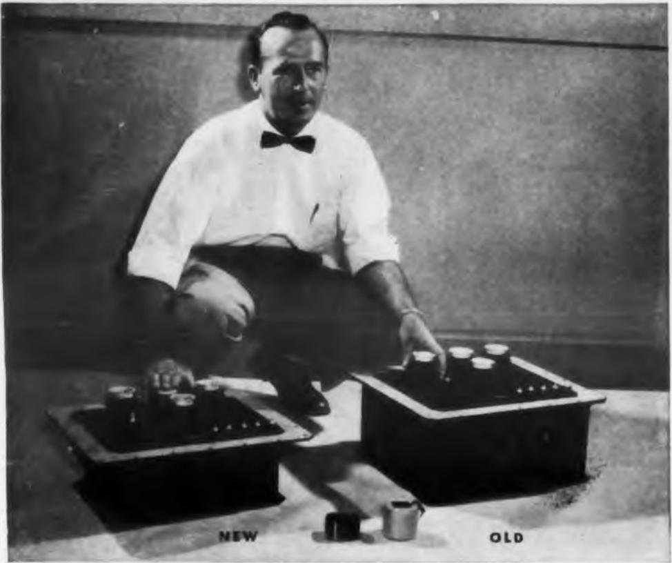
WEIGHT OF A TYPICAL POWER SUPPLY WAS CUT 61 LBS. when redesigned for smaller embedded-layer coil. New and old coils in foreground illustrate typical size reduction now possible.
