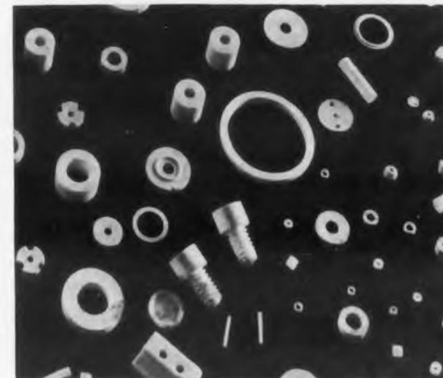
Cap screws and other tough parts can be made.
