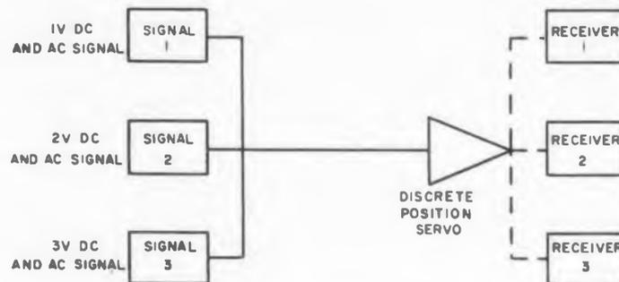
Fig. 10. An inexpensive multiplexer for communications equipment.
