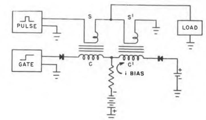
Fig. 9 (left). Balanced gating circuit for reducing blocked signal. Compound method, Fig. 10 (right).
