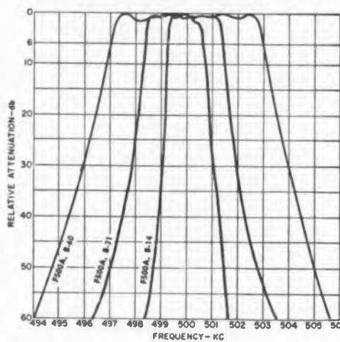
**F500** Mechanical Filters for AM, CW, RTTY signals at 500 kc. Bandwidths of 1.4, 3.1 and 6.0 kc at 6 db attenuation. Nominal transmission loss, 23 db.
