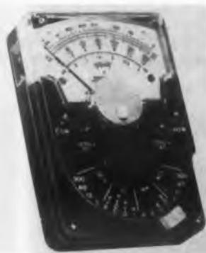
The Model 310 is a miniature VOM which can be carried in the pocket. It has a wide variety of a-c and d-c voltage, d-c ma and  $\mu$ amp, and ohms and megohms ranges. It provides 20,000 ohms/v d-c and 5000 ohms/v a-c. Size of the unit is only 2-3/4" x 4-1/4" x 1-3/16". The
