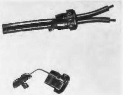
All popular-size "Heyco" strain relief bushings made by this firm are now of one-piece construction. The two component parts of the former units now are joined by an integral web of thin, tough nylon. This joining web is completely flexible, yet strong and will not crack or weaken with handling. When the bushing is assembled, the web in no way interferes with the cord.
