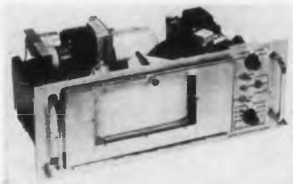
These one and two - channel direct-writing oscillographs are available with 8 or 16 recording speeds. The chart drive is electrically - controlled, permitting
