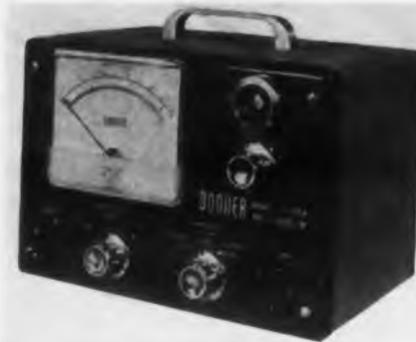
This portable Wow and Flutter Meter is expressly designed to meet the recently adopted IRE-SMPTE-ASA standards on sound recording and reproducing methods for determining flutter content.
