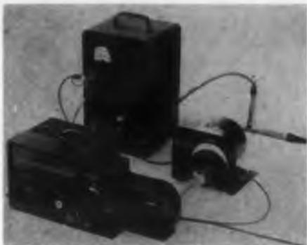
This sweep drive for oscillators replaces point-by-point frequency analyses by using a mechanical hand which turns an oscillator dial back and forth. Known as the
