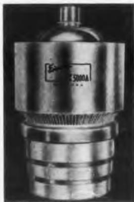
The 4X5000A, a radial-beam power tetrode, is constructed entirely of ceramic and metal, thereby offering greater electron-tube reliability and increased immunity to damage from thermal and physical shock. With a plate dissipation rating of 5000w and a power output of 16kw in Class C telegraphy service through 30Mc, the unit fills a power gap in the tetrode field. Especially
