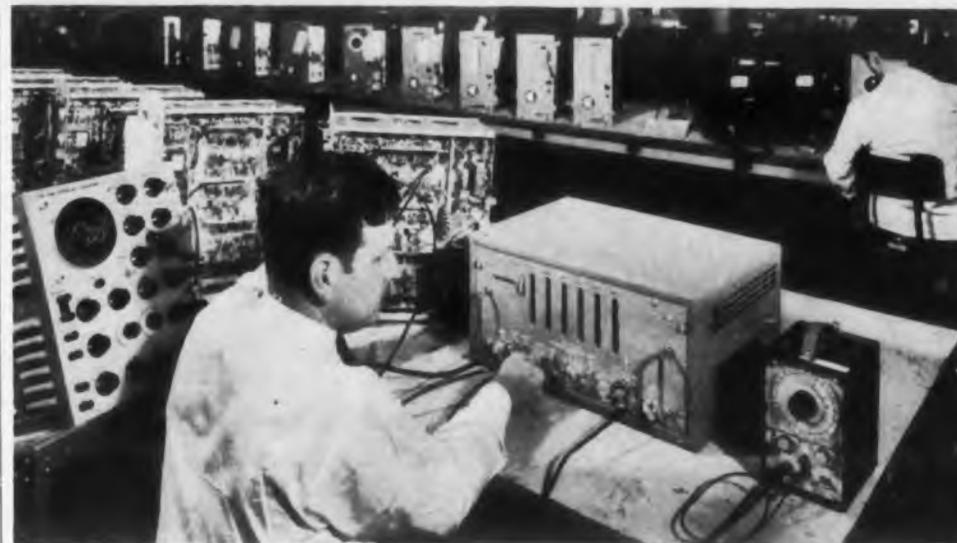
Typical digital phase-shift measurement set-up employing a BERKELEY Model 5510 Universal Counter & Timer, with a Shasta oscillator as reference frequency source and an oscilloscope to provide visual check.
