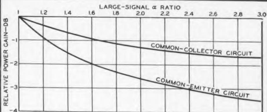
Fig. 5. Characteristics of class B amplifier pairs having mismatched  $\alpha$  and matched  $R_{in}$ .
