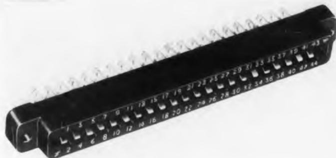
To meet the requirements of equipment using printed-circuit construction, five new connectors have been made available in 10, 18, 22, 28, and 44 contacts. These fittings are made of Dupont "Zytel" molded insulation, with gold-plated phosphor-bronze or beryllium-copper contacts. Flashovers are 2000 and 2500v 60cy a-c (rms), with a current rating of 5amp.
