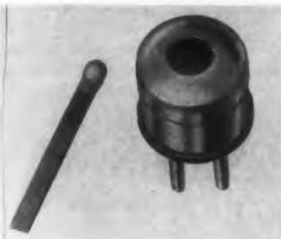
The 1317 is a low-cost, remote detector of far infrared energy designed specifically for use in commercial applications of "non-contact" heat detection measurement, and control systems. This ther-
