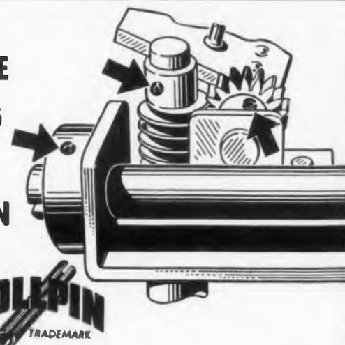
Rollpin speeds production alignment of close tolerance shafts. The slotted, hollow steel spring pin, with chamfered ends, is simply pressed or driven into holes drilled to normal production tolerances. It compresses as driven, is self-locking and vibration-proof. Rollpin is light, easily removable, reusable and has a shear strength greater than a solid pin of the same diameter. Diameters from 1/16" to 1/2".
