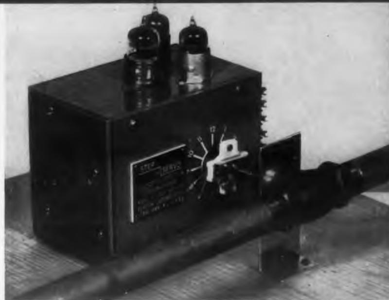
The discrete-position servo can control a fuel line, as illustrated, in addition to many other liquid flow systems. Fig 7 is the block diagram.
