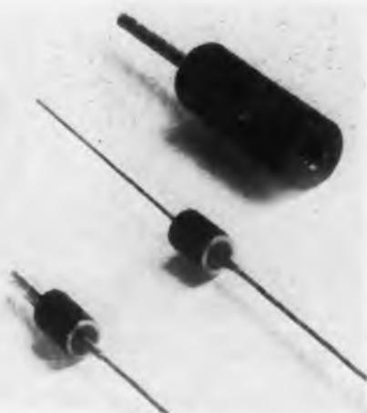
The type BD series of SiR Silicon Area Rectifiers have an average rectified forward current of 25amp for an inverse working voltage as high as 1000v. These rectifiers make it practical to design high power d-c generators and motors without commutators or brushes. The largest units are only 0.5"OD by 1" long.
