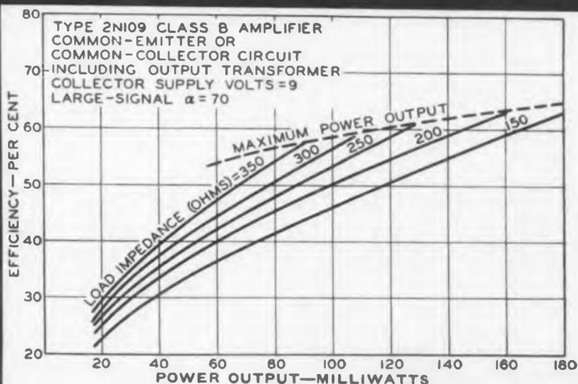
Fig. 6. Efficiency decreases as power level is reduced.
