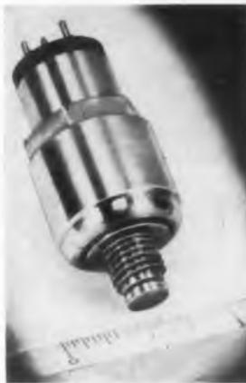
For maximum convenience in the measurement of pressures up to 7000psi, this group of high-performance pressure pickups features pressure-sensitive diaphragms only 1/4" in diameter. A pickup can be mounted in a 5/16-24 threaded hole. They are particularly suitable for studies in high-pressure hydraulic and pneumatic systems.
