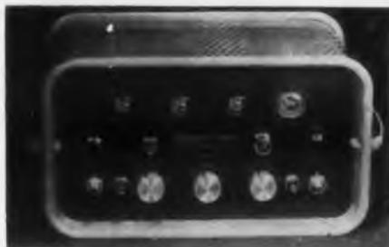
The WE-210 is a small, lightweight, inexpensive, yet highly accurate time interval meter and frequency standard using glow-transfer tubes in the counter unit and a crystal-controlled oscillator as the time base. Time is displayed directly to the nearest 0.0001sec by four easily read decades. Two ranges of 1sec and 10sec are provided; longer intervals are easily noted by watching the thousands decades, or by use of an auxiliary electro-mechanical register.
