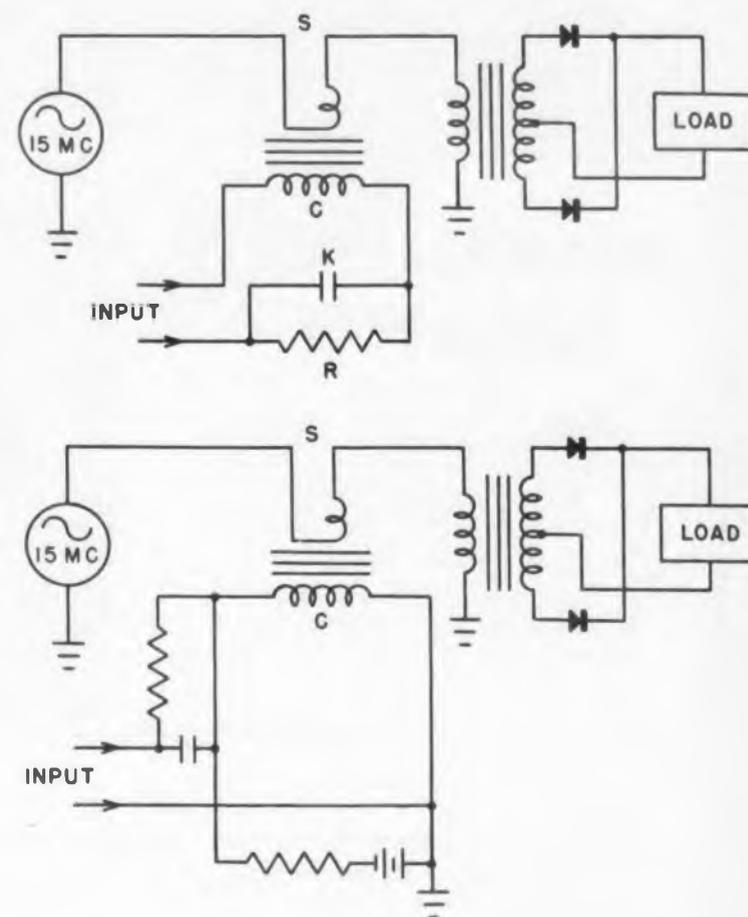
Fig. 11 (top). General Magnistor amplifier circuit. Typical audio amplifier, Fig. 13, (lower).
