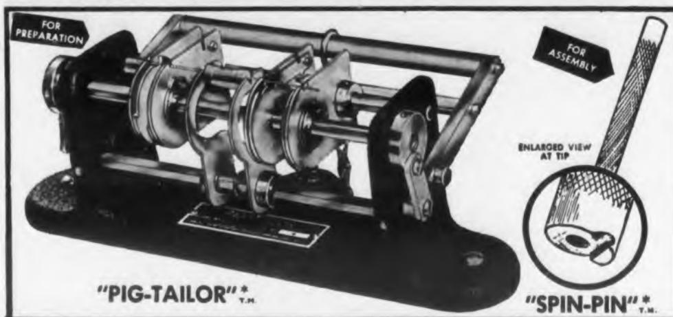
The "PIG-TAILOR" plus "SPIN-PIN" — Accurately Measures, Cuts, Bends, Ejects and Assembles both leads simultaneously to individual lengths and shapes — 3 minute set-up — No accessories — Foot operated — 1 hour training time.
