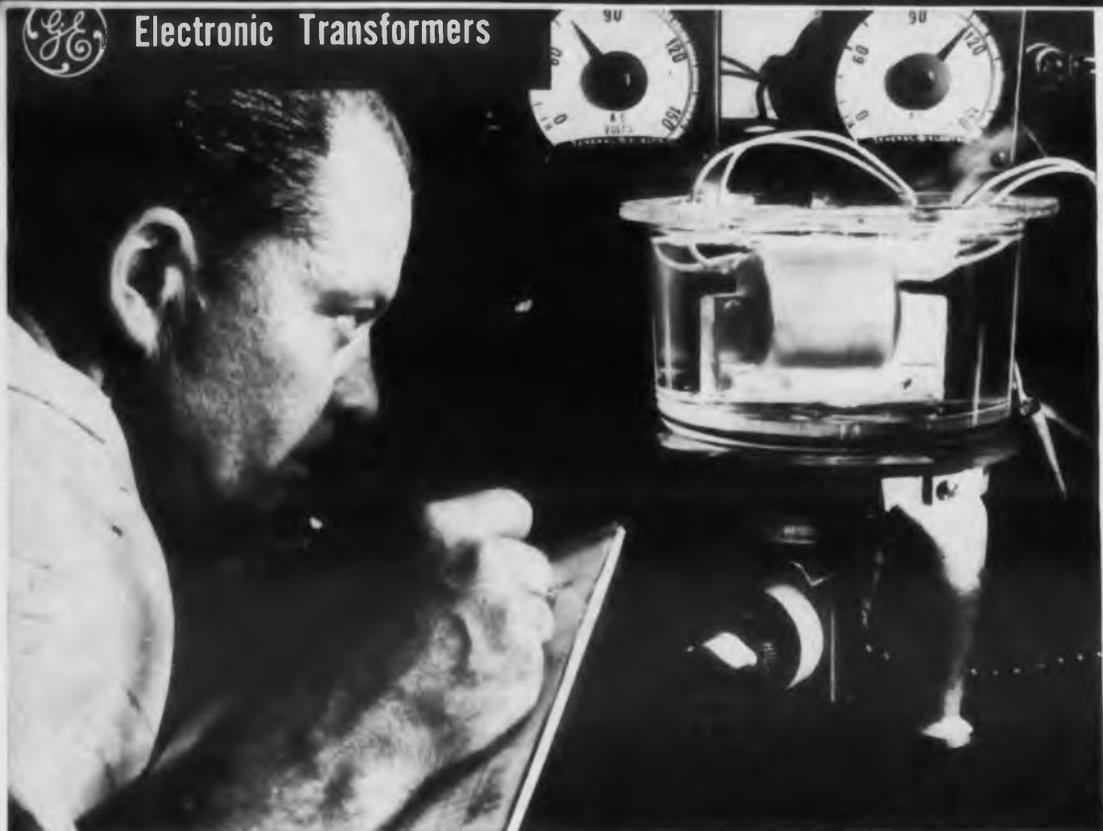
TO PROVE THE MOISTURE-RESISTANT QUALITIES of G-E high temperature encapsulated transformers, our engineers operated one in boiling water. Your application probably won't ever require this much protection, but it proves that G.E.'s encapsulated transformers can take it!
