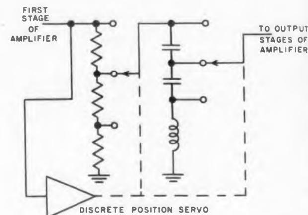
Fig. 6. In this a-g-c circuit, capacitive phase-shift is provided to a certain limit, with inductive phase-shift beyond.
