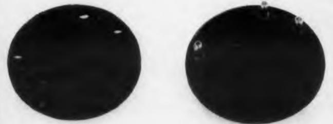
An electronic component made with the material. At the left is the "preform" before the metal inserts are molded in.
