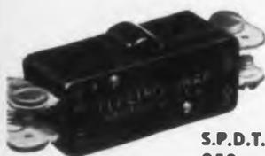
S.P.D.T., 2 circuit; 10 amps, 125/250 v. AC/ 30 v. DC. Ind. Screw or solder terminals on ends or one side of switch. Also available with reset button at bottom of switch or in Type S-100 Make-Before-Break Series where switch completes a new circuit before interrupting old one.
