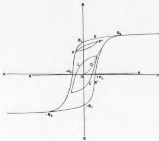
Fig. 2. Ferromagnetic B-H curve.
