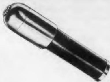
The Model CS-100 "Radimax" is a collimated scintillation counter with heavy shielding for maximum directionality. The unit is supplied with a 1" x 1" sodium iodide crystal, and other sizes
