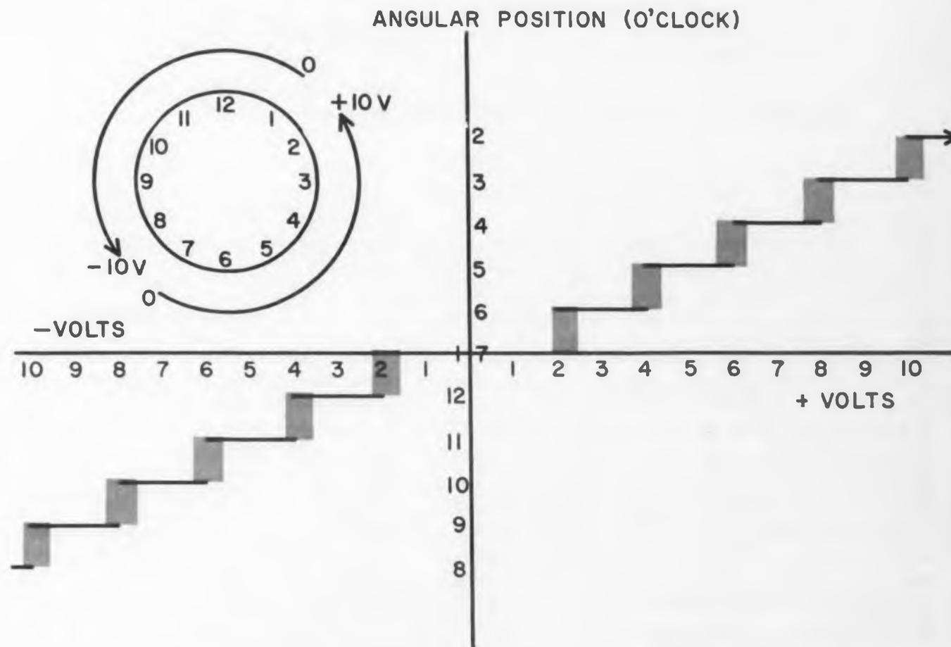
Fig. 5. Voltage input plotted against angular position for a commercially available form of the discrete-position servo. The step does not occur at an exact point, as indicated by the color.
