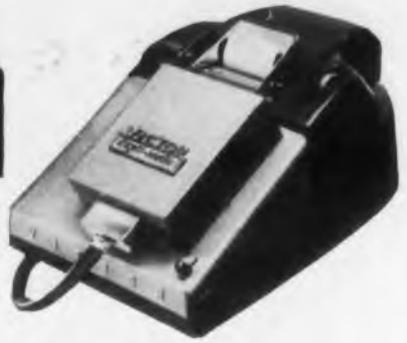
The Digit-Matic accepts numerical information electrically from all types of digital output devices, performs required calculations and records entries and results.
