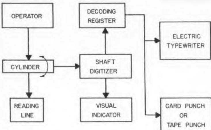
Shaft digitizer is set as reading line is adjusted. Decoding register (and storage) is located below typewriter in illustration above.
