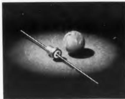
This miniature "cup" electrolytic capacitor is the fifth design to be added to the "Tantalex" line. Designated Type 104D, these units are valuable for low-voltage applications, where they provide values of capacitance up to 30 mfd in volumes less than 1/10 cu in. The use of tantalum, the most stable of all anodic film-forming materials, gives them unusual stability of performance. They exhibit no shelf aging under long periods of test, and have extremely low leakage current.
