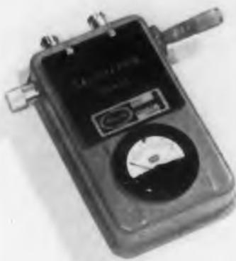
The "C&D" S-band wavemeter is an inexpensive unit for the frequency range from 1800 to 3800Mc. It features highly sensitive indication of resonance, with a control for setting the sensitivity of the instrument. Its micrometer extends outside the instrument, providing easy reading.
