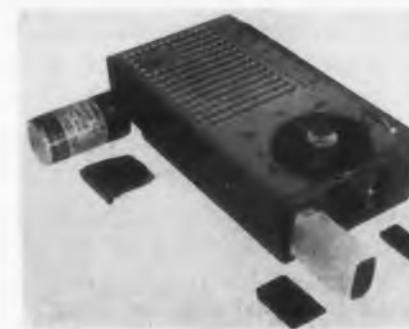
The tube-transistor radio showing how the batteries are replaced without removing the chassis. The hole near the dial is for a final trimmer adjustment after assembly.
