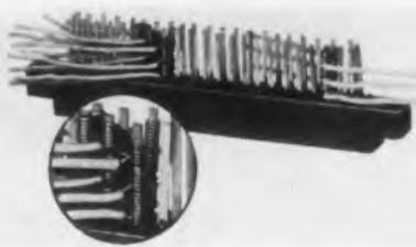
The PCW-22, a printed-circuit "Continental" connector, was developed originally for computer applications. It can handle 132 solderless connections with 24 gage wire. The illustration shows three wires wrapped around each of 44 contacts (two rows of 22 contacts each).
