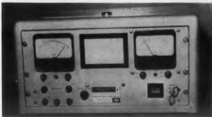
This meter furnishes accurate information on the noise figure of a transistor in a single reading simply by inserting the transistor into a socket. Valuable as a laboratory tool, it also is useful for large scale users of transistors. Its high speed of operation makes 100% inspection possible.
