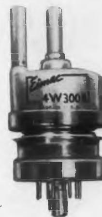
The "Eimac" 4W300B radial-beam power tetrode may be used as an amplifier, oscillator, or frequency multiplier into u-h-f. It is a water and air-cooled version of the "Eimac" 4X150A. Rated at 300w plate dissipation, this powerful little tube delivers 140w of useful power output at 500Mc in a coaxial-cavity amplifier circuit. The tube is especially suitable for applications requiring higher plate dissipation capabilities than the air-cooled 4X150A.
