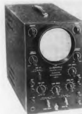
This unit is an inexpensive oscilloscope having many laboratory-quality features. It is recommended for industrial applications where square-wave and pulse type signals must be observed, and for field service use. Vertical amplifier response is flat from 10cy to 4.5Mc ( $\pm 3db$ ). The four-step frequency-compensated vertical
