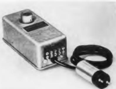
The "Delta Unit", converts changes in capacitance to changes in voltage. It may be applied to the measurement of any physical phenomena which can be resolved into
