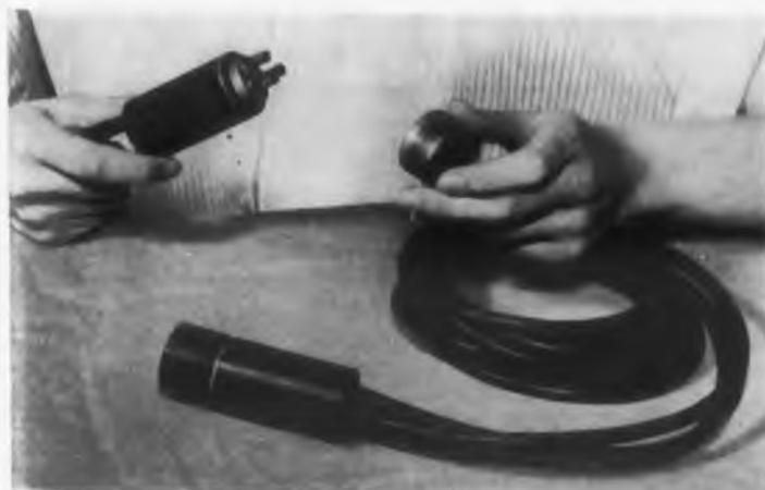
Incorporating three transistors, this adapter pre-amplifier for plane intercoms weighs only 6 oz.
