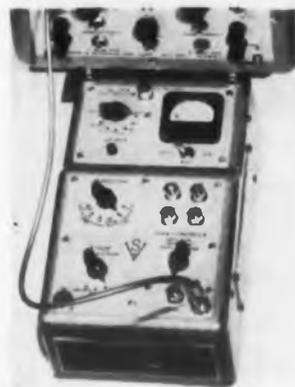
The Type VS-61 "ultra-low-noise scope preamplifier" has less than 0.5 $\mu$ v rms noise over its entire frequency range of 2cy to 60ke. Its design is based on the discovery that transistor noise can be reduced substantially below the noise level of vacuum tubes if suitable low-noise operating parameters are selected.
