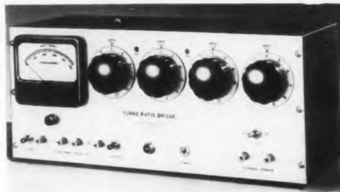
The Model MC-127 Turns Ratio Bridge is fed by an RC type audio generator and an amplifier. It has two unknown transformer windings in two legs. The ratio division resistors are in the third leg, and the balancing decade resistor is in the fourth leg.
