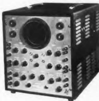
The Model K-26 Dual-Channel Oscilloscope is for viewing or photographing virtually any two simultaneous phenomena. It is designed for low cost plus wide applicability. The scope employs two completely separate and independent channels with
