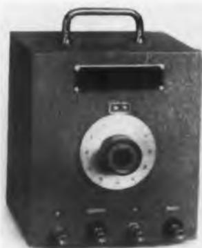
This delay line consists of 60 sections of LC m-derived networks and one 60-position rotary switch. The networks are especially designed for fast rise time and negligible overshoot. The switch is used to change the amount of time delay between the input and output by connecting the output terminal to any one of the 60 sections of LC networks. The accuracy of time delay can be as high as  $\pm 0.5\%$  of the time delay at any point.
