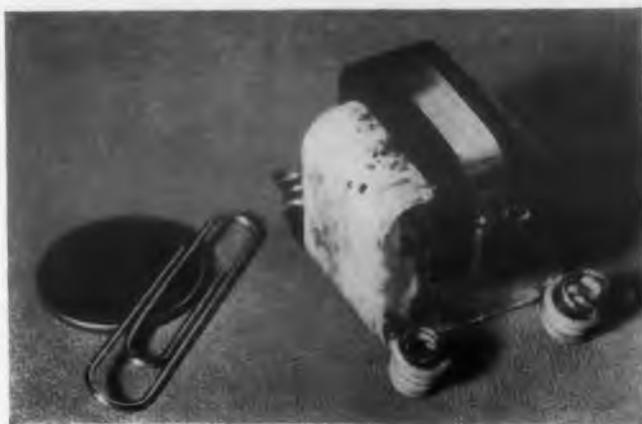
With a volume of less than one inch cubed, this transformer has a weight-to-power ratio of 0.007 lb/w. Output is 12.6w.
