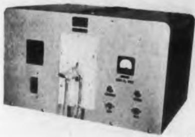
Induction Heating Unit Model IH-3 has a conservatively rated output of 3kw (per NEMA standards). It features simplicity of design and rugged construction.
