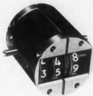
The Model 1502 Angle Counter features a reduced number of moving parts. It indicates angular changes from 0 to 359° and back to 0, in 1° divisions. One revolution of the input shaft is equal to one revolution of the unit drum.
