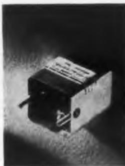
Style B Type 1 Variable Inductors are carbonyl-iron cup-core units completely embedded in epoxy resin. They are provided in 16 standard values from 56μh to 18mh. Their construction makes them resistant to the effects of large amplitude vibration and shock, as well as moisture and chemical attack.
