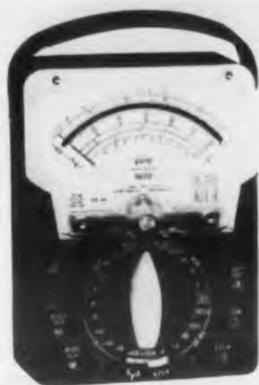
The Model 630-NA "Volt-Ohm-Mil-Ammeter" features meter protection against overloads; 70 ranges, nearly double those of conventional testers; and frequency compensation up to 20kc, providing for accurate readings over the entire audio range. In addition, it has high accuracy on the same scale for a-c and d-c: 1-1/2% d-c to 1200v, and 3% a-c to 1200v.
