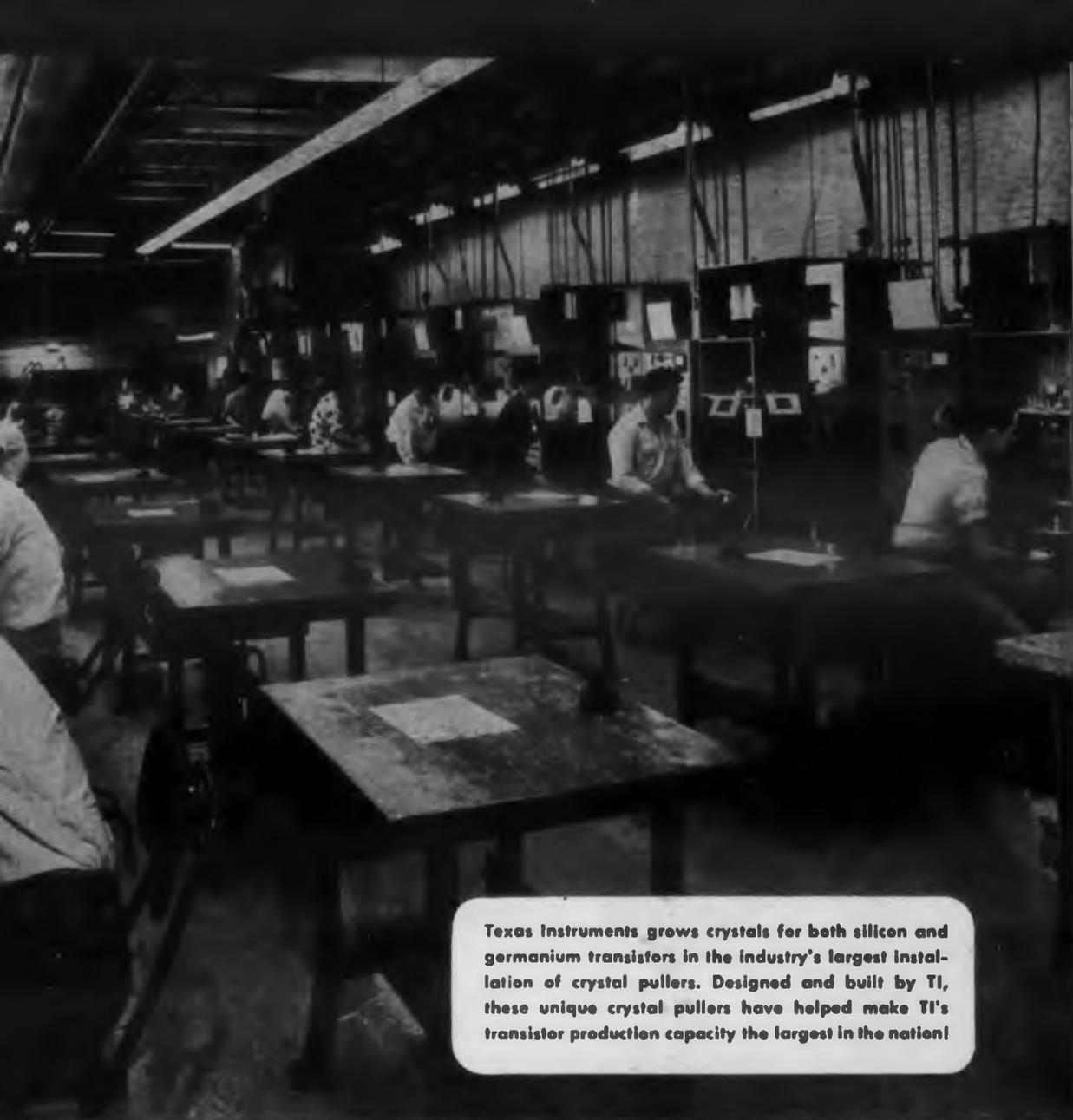
Texas Instruments grows crystals for both silicon and germanium transistors in the industry's largest installation of crystal pullers. Designed and built by TI, these unique crystal pullers have helped make TI's transistor production capacity the largest in the nation!
