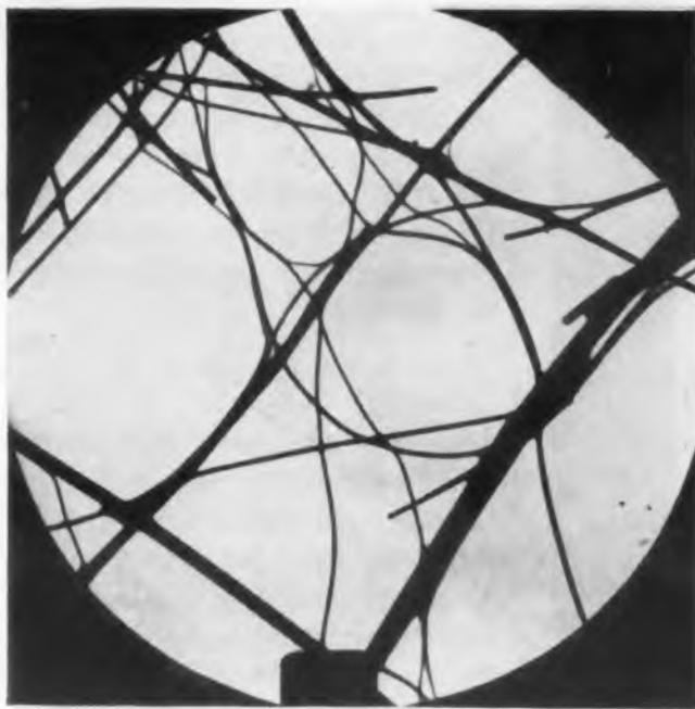
Microphoto of the newly improved glass-fiber paper showing the formation of a binder at the intersections of the fibers.
