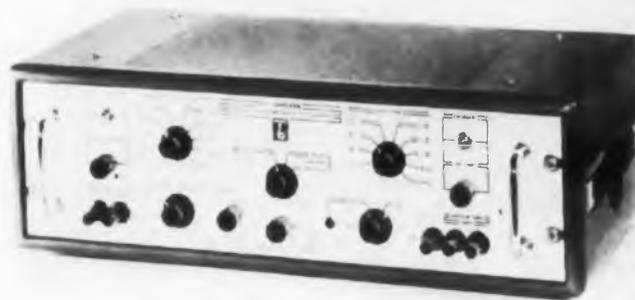
The Model BL-550 is a high-sensitivity d-c recording amplifier with a gain of 10,000. It is a sturdy, direct-coupled amplifier employing a chopper stabilized feedback circuit that eliminates the need for matched tubes. This circuit permits extended frequency response. When used with Brush direct-writing oscillographs, the frequency response is d-c to 100cy. In its application to photographic equipment, the frequency range can be extended to 5000cy.
