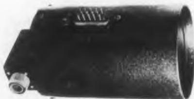
The Type NU-DVI-3 is a high-brightness, daylight-viewing 5" oscillograph presentation unit that uses both electrostatic focusing and magnetic deflection.
