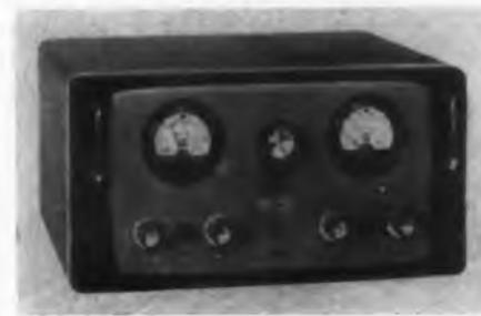
The Model UHR-240 Regulated Power Supply provides up to 1/2-amp of d-c at 0-500v with 0.001% regulation and less than 100 $\mu$ v of ripple. The stabiliza-
