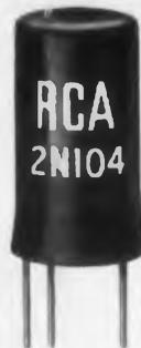
The **2N104** is a germanium alloy-junction transistor of the p-n-p type for low-power audio applications. It has been carefully designed and manufactured for extreme stability, very low leakage currents, and excellent uniformity of characteristics throughout its life.
