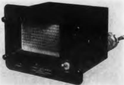
The Model 20 Dynamic Visual Monitor combines 24 moving-spot, light-beam galvanometers in one package, 8-1/2" x 8-1/2" x 6", weighing less than 13.5 lb, to
