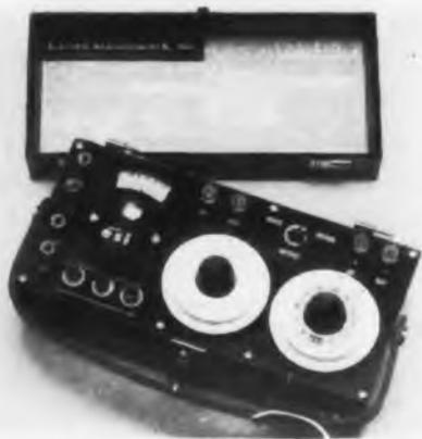
This Wheatstone and "Fault Locating Bridge" is engineered for rough use in the field, yet offers excellent readability with high accuracy and reliability. It is supplied in a strong, lightweight, weatherproofed
