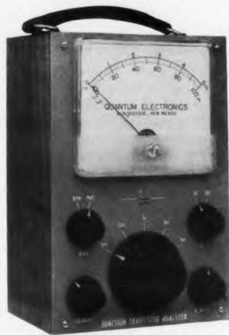
**C**OMpletely portable, this compact, three-pound junction transistor analyzer uses transistorized circuitry. It is powered by three flashlight batteries. The analyzer measures  $h_{21}(\beta)$ , the short circuit current gain, and  $I_{co}$ , collector cut-off current. True small signal parameter,  $h_{21}$ , is measurable for various values of emitter bias. Unlike transistors can be compared for identical operating biases.
