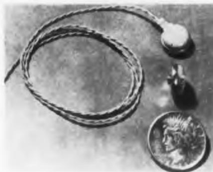
Wide bandwidth and ultra-thin size are features of this magnetic transistor receiver developed for use in portable amplifiers, hearing aids, earphones, and other electro-acoustical devices.
