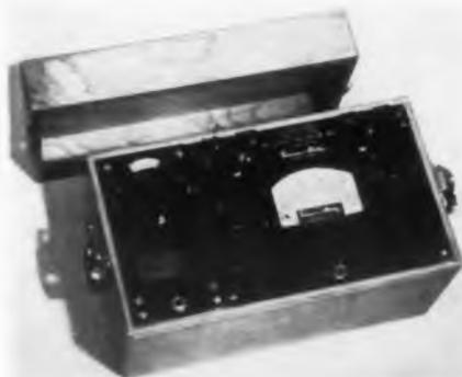
Seven ranges, covering values from 0.25 to 25mv are provided in this portable indicating instrument. Laboratory precision is combined with ruggedness, permitting field use. Specific uses
