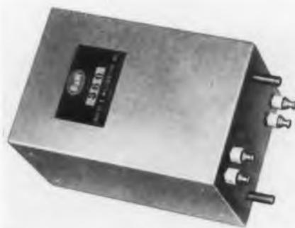
This filter is designed specifically for single sideband. Its construction includes use of eight stabilized toroidal inductances and precision silver mica capacitors in an LC type filter designed to pass
