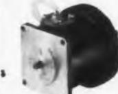
**MODEL 430 AIRCRAFT DRIVE MOTOR** — 1/12 h.p. 11,000 r.p.m. Teflon insulation. -65° F. to +160° F. Completely qualified to MIL 7969 specs.
