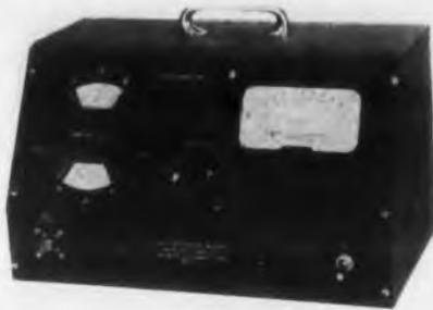
This R-F Distortion Meter is designed to measure the total harmonic distortion present in r-f sources from 1 to 100 Mc. In principle, the meter completely suppresses the funda-
