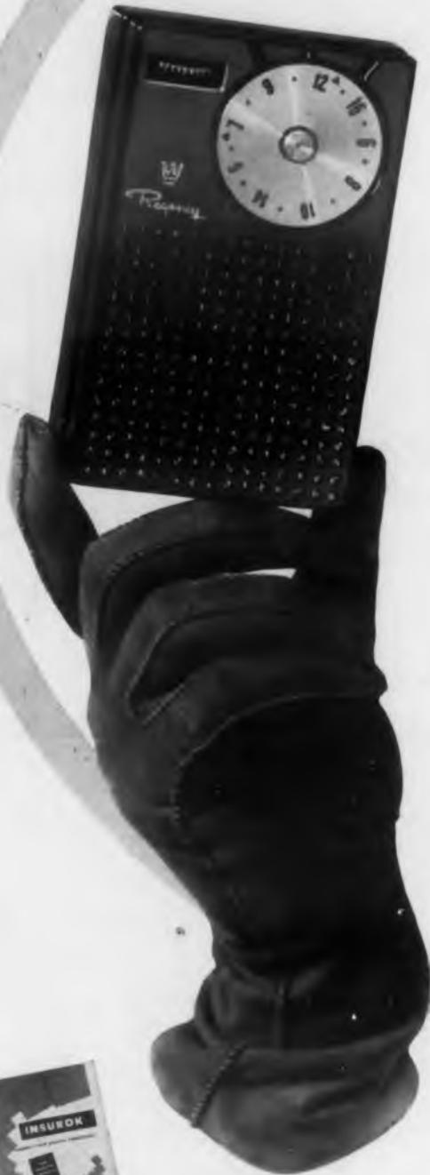
Here's a remarkable example of miniaturization . . . made possible mainly through the use of printed circuits and transistors. This diminutive radio weighs a scant 12 ounces, complete with battery. Yet, it has good tone, is selective, and delivers plenty of volume.
