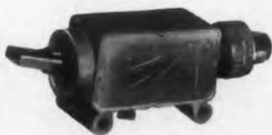
This unit combines rotary actuation plus a hermetically sealed basic switch. The sturdy roller actuator arm has optional settings throughout 360° with operating travel of 90°. The long over-travel of 81° protects the basic hermetic switch and also permits flexibility of application.
