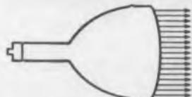
**MAGIC-MIRROR ALUMINIZED TUBE**—Aluminized reflector allows electron beam through. Blocks wasted light from backing up into tube. Reflects *all* the light into picture.
