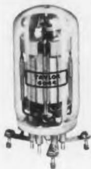
The 6011 is an inert-gas grid-controlled rectifier featuring the use of a high-shock multiform glass wafer stem. It is designed especially for motor control circuits where short deionization time is required. The tube will also serve on applications requiring high peak-current-carrying capacity, such as timing control.
