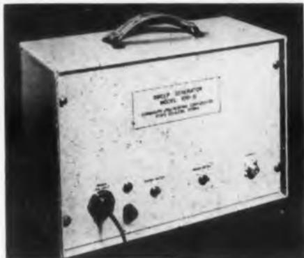
A line of wide-band sweep generators, announced by this firm, is for use in work with TV antenna and cable systems, or similar applications. Frequency ranges of the three models are
