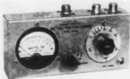
The Type 28 is a compact, r-f wattmeter bridge measuring only 2" x 4" x 8". It performs three r-f measurements. As a wattmeter, impedance
