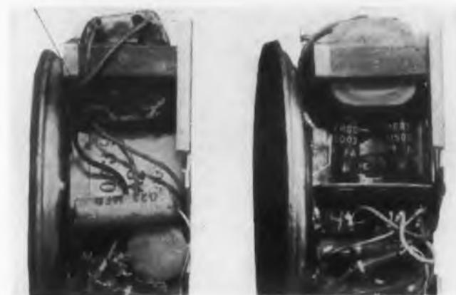
The transistors are mounted in a previously empty space behind the speaker.
