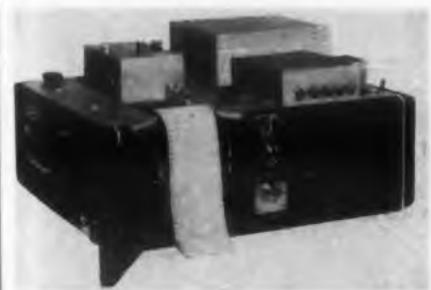
For electro-acoustical measurements, this recorder is based on the electro-dynamic principle and utilizes a "sliding coil" for the operation of the writing mechanism.
