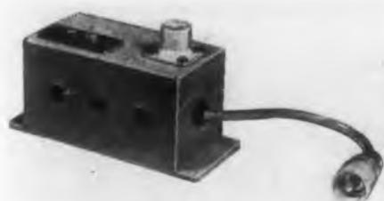
This compact automatic electronic transmit-receive switch is suitable for amateur and commercial radio transmitters with up
