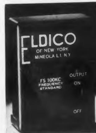
Self-contained unit is crystal controlled. No external connections are required.
