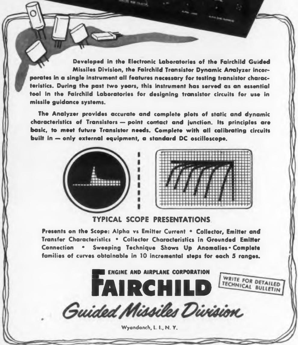
Developed in the Electronic Laboratories of the Fairchild Guided Missiles Division, the Fairchild Transistor Dynamic Analyzer incorporates in a single instrument all features necessary for testing transistor characteristics. During the past two years, this instrument has served as an essential tool in the Fairchild Laboratories for designing transistor circuits for use in missile guidance systems.
