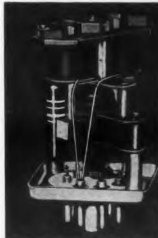
Frahm Resonant Reed Relay is an electro mechanical device which responds to an alternating signal having frequency and amplitude values that lie within specified bands. A number of control signals over a single circuit is possible with all types of communication circuits, including radio. A signal is transmitted either on a wire line, or as a modulated carrier to some remote location
