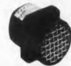
**MODEL 102DA AXIAL FAN MOTOR** — Totally enclosed, panel mount, screened intake, high temp. operation 20 CFM N.A.F.M. at free air. O.D. 1.45", 115 V., single phase, 400 cycle, or variable frequency models.
