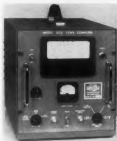
Model 621B VSWR Computer is designed to provide expanded utility and operator convenience in automatic development and production tests of microwave components and systems. Four linear scales, each covering a 10:1 range, are provided for voltage reflection coefficient percentages from 0.5
