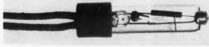
This switch is offered single pole normally open, and single pole normally closed. It is much more rugged, with a larger mercury pool, and smaller in size than previous models manufactured by this firm. The weight of armature and movable contacts is supported by an electrically conductive bearing, resulting in an exceptionally sturdy unit. The spring is used for return purposes only. There are no leads to flex and break.
