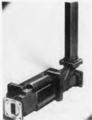
The high-power ferrite circulator is a broad-band, high-performance, lightweight, non-reciprocal ferrite component capable of handling full magnetron power without external cooling. The circulator has dual application as a load isolator or a combination isolator-duplexer package. It is used to stabilize high-power magnetrons that are
