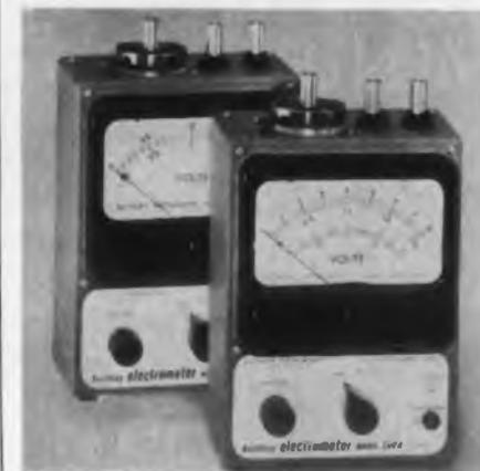
Models 200 and 200A Electrometers, battery-operated d-c vacuum tube voltmeters with input impedances exceeding  $10^{14}$  ohms, and available in an improved version. These are now fitted with output terminals, providing
