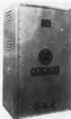
The Model 1420-B Variable Frequency Electronic Generator is a versatile power source for use in the development or testing of equipment operating over a range of power supply frequencies. The frequency range of its internal oscillator is 50-6000cy with an external oscillator of 25cy-20kc.
