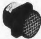
**MODEL 182DA AXIAL FAN MOTOR** — Totally enclosed, panel mount, screened intake, high temp. operation, 20 CFM N.A.F.M. at free air. O.D. 1.45", 115 V., single phase, 400 cycle, or variable frequency models.
