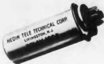
Engineered for d-c applications, the 100-C Relay is available either hermetically sealed or with dust cover in contact combinations from spst to dpdt. It incorporates the unique feature of thorough wiping action yet with a sensitivity of 10mw. This wiping effect has the advantage of eliminating the bounce and chatter at normal operating voltage.
