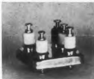
This terminal is composed of Steatite insulators which compress a silicone rubber grommet against an extruded hole in the header, forming a leak-proof oil seal capable of withstanding extremely high internal pressure. D-c metallic migration is prevented, and operating temperatures range from  $-60^{\circ}$  to  $+500^{\circ}$ F. Standard voltage rating is 2000v to 7000v.
