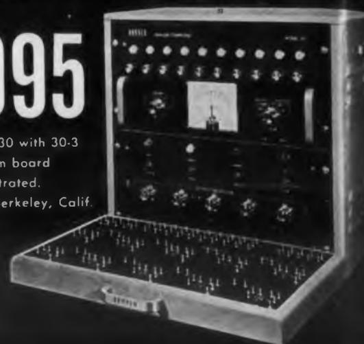
This versatile and compact Donner Model 30 is the first electronic computer specifically designed as a personal tool of the engineer, mathematician and scientist. It offers the speed and accuracy of electronic computation with slide rule operating simplicity wherever differential equations are used.
