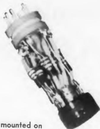
Components are mounted on a turret socket prior to the encapsulation process.
