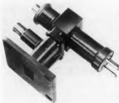
flex klystron, the VA-203 is for airborne X-band radar receiver and beacon local oscillator service. It has a brazed-on external tuning cavity to assure exceptional frequency stability. This klystron can withstand shocks of 50G to 100G without malfunction or damage.
