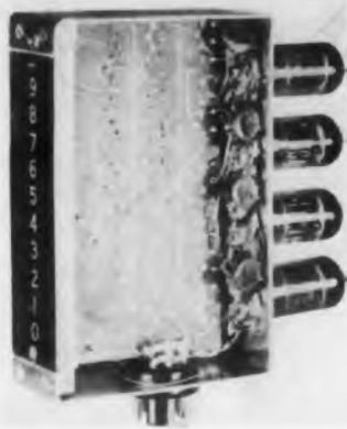
Two Digital Decade Counters, each available in three variations, are for use wherever high-speed electronic counting is required. Both types employ the printed circuit principle, thereby permitting maximum ventilation, low operating temperature and longer life.
