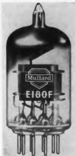
The Mullard *E180F* is a new miniature pentode with a high mutual conductance of 16.5ma. This, together with its low interelectrode capacitances, makes the tube ideal for all wide-band amplifier applications, such as radar i-f amplifiers, high definition television cameras and transmission equipment, and carrier telephone equipment, especially that used with coaxial telephone cables.
