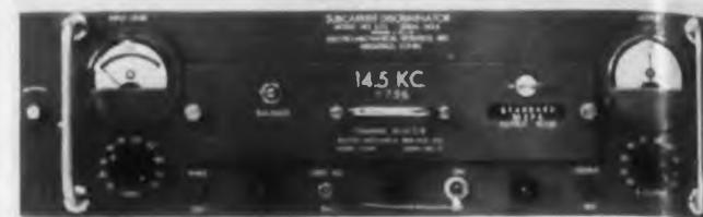
The Model 67 Precision Subcarrier Discriminator is for use in f-m telemetry and data recording systems. The discriminator contains its bandpass input filter, frequency determining network, and interchangeable output filter in a single front-panel plug-in unit. Three outputs are provided, one of which will drive most pen motors to full deflection. Each discriminator contains its own electronically regulated power supply.
