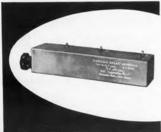
A new series of Variable Delay Networks, designed for laboratory use to facilitate design and development of advanced computer and radar systems is now available. Compactly designed for front panel mounting (gussets provided as specified), these delay networks offer a variation of delay from 0 to .75  $\mu\text{sec}$  in 10 turns of a Vernier control shaft.
