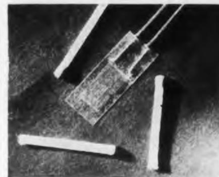
The "RdF Stikon" line of resistance-thermometer elements has been broadened by the addition of the SN-1, a new type for higher temperature applications.
