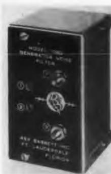
For amateur, marine, aviation, police, utility, civil defense, military, and similar uses, the Model 1080 is a completely shielded generator filter designed to materially reduce commutation "hash" and "whine" throughout the high-frequency amateur bands. These filters are supplied complete with a 4-way mounting bracket for quick, easy installation on one end of the vehicle generator.
