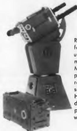
Remote Control TV Camera; for broadcast and industrial use. Pre-set control permits memory of 6 different shots. Mounted on servo-operated pedestal, provides complete remote control of lens selection, iris, pan and tilt. Highly useful for observing dangerous phenomena; permits broadcasting without use of camera man.
