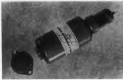
A basic building block for doing complicated switching operations at speeds up to 200kc, the "Logiblock" contains four cores, three diodes, and a buffer amplifier tube.
