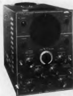
Precise measurements and analyses of phenomena which take place at extremely high rates of speed may be made with the Type 336 Cathode-ray Oscilloscope. The instrument is expected to have applications in nuclear studies, development and maintenance of high-speed electronic computers, design
