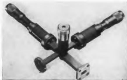
The DB-350 Crystal Multiplier enables experimentation in the "Ultramicrowave" region up to 90,000-Mc. It is designed to operate with this company's new ul-
