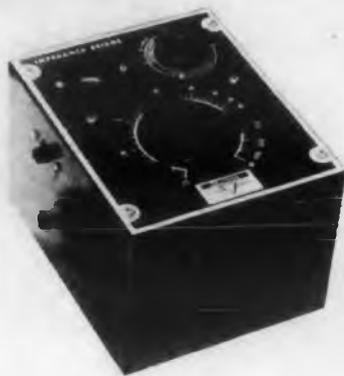
This "R.C." low-cost, completely self-contained, portable resistance-capacitance bridge is designed to increase the speed and accuracy of making measurements on capacitors from 10mmfd to 50mmfd, and resistors from 10 ohms to 50 megohms. It can also be used for making
