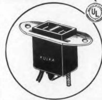
No. 221 (above) with solder terminals and steel bracket with #6 clearance mounting holes. Also No. 222 with 6-32 tapped mounting holes. No. 223 with 8" #14 or #16 plastic leads and steel bracket with #6 clearance mounting holes. No. 224 with 6-32 tapped mounting holes.
