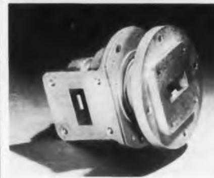
This compact rotary joint, for waveguides in the  $K_u$ , X, and S bands, is available for both 90° and 180° orientation of input and output waveguide sections, and provides 360° continuous rotations at high speeds with broadband operation and very high power handling capabilities. At the same time, vswr is extremely low (less than 1.10 over the entire frequency range of  $f_0 \pm 0.06 f_0$ ).
