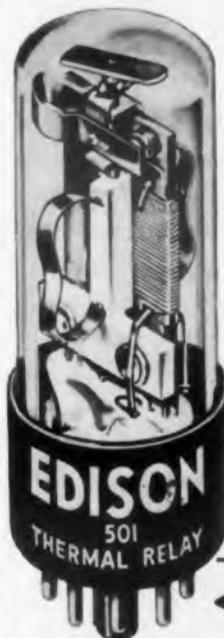
A preloaded Inconel spring fulfills one of the most important requirements in this Edison Time Delay Relay. It maintains steady contact pressure.
