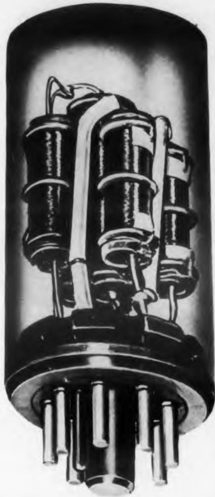
Five precision resistors attached to octal tube socket.
