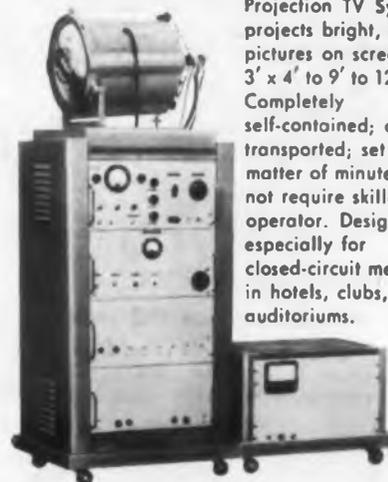
Projection TV System; projects bright, clear pictures on screens from 3' x 4' to 9' to 12'. Completely self-contained; easily transported; set up in matter of minutes; does not require skilled operator. Designed especially for closed-circuit meetings in hotels, clubs, auditoriums.
