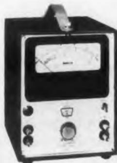
The Model 202A voltmeter is designed for the accurate measurement of a-c voltages from 0.001v to 300v full scale in the frequency ranges from 20cy to 2Mc. The input impedance of 10 megohms and 25-mmfd minimizes errors due to loading of the circuit under test. Separate terminals are brought out from the
