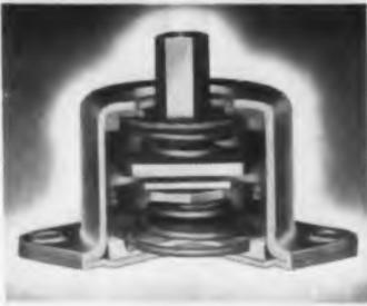
The ALL-ANGL mount above has a standard one-inch cup to mount on 1-13/32" centers, and is interchangeable with other miniature BARRYMOUNT® isolators. Weighing less than one ounce, it handles loads up to 3 pounds.
