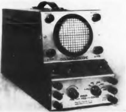
This D-C "Mid-getscope", Model No. 534, combines linear sweep with a d-c amplifier for color TV restorer circuits and for complex waveforms. Other features include provisions for a-c coupling; full
