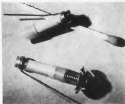
Only 3/4" in overall length, this midget glass rotary trimmer capacitor features a very low minimum capacitance and smooth trimmer adjustment. It is suitable for application in any commercial
