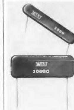
The units shown are the test additions to this fine line of resistors. Employing a unique method for attaching the leads to the body of the resistor, the construction is designed to provide desirable in mechanical and electrical connections. Wound on ceramic cores and covered with an extremely hard ceramic based coating, they are available in 4w to 25w, 5 ohms to 18,000 ohms resistance.
