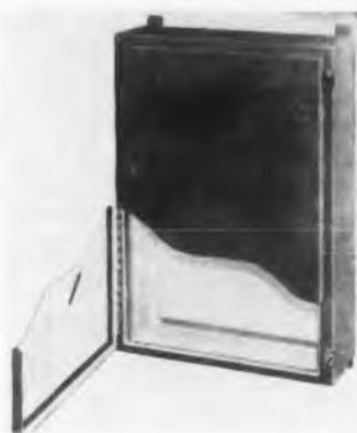
Fifteen standard sizes of NEMA "12" sheet metal panel enclosures (16" x 12" x 6" to 60" x 36" x 8") are available from this firm to supplement its line of oil-tight "JC" electrical pull boxes and troughs. These enclosures are constructed to be completely liquid tight. All seams are welded, and there are no
