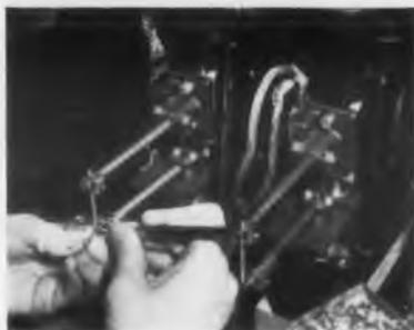
**Standardized Work Place Setups** for each material combination and geometric configuration to be welded, including specification of welder head, electrode material and design, welding current, time and pressure insures optimum welding conditions at all times.
