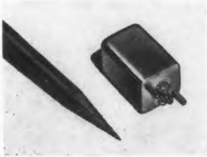
The dimensions of this standard series of subminiature bandpass filters are  $23/32'' \times 23/32'' \times 1\text{-}1/16''$  high. The units have a 0.55 cu in displacement and exhibit excellent
