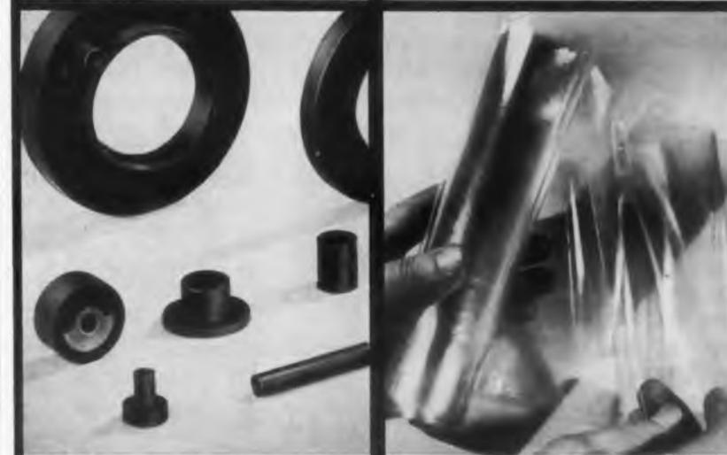
Superior dielectric properties of BAKELITE Fluorothene at elevated temperatures make it an ideal material for these insulators and other parts used in high-frequency radio circuits. Excellent molding properties make it possible to produce these variously shaped parts to close tolerances.
