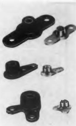
This all-metal self-locking miniature nut is designed to use only one-half the space of comparable standard anchor nuts and to be only one-fifth the weight, thus effecting weight savings of 80%. It retains the full tensile strength of the original "Kaylock" self-locking standard anchor nut.
