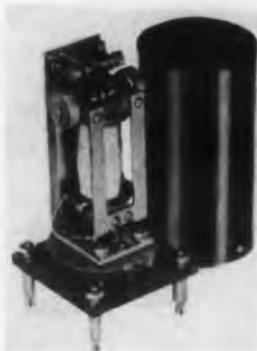
The P255A Polarized Relay utilizes a reed-type, Permaloy armature with anti-chatter contacts. The armature is equipped with extra-heavy (3/32" diam) palladium-copper contacts. The contact screws have 1/16" diam tungsten contacts rated at 2amp 110v d-c.
