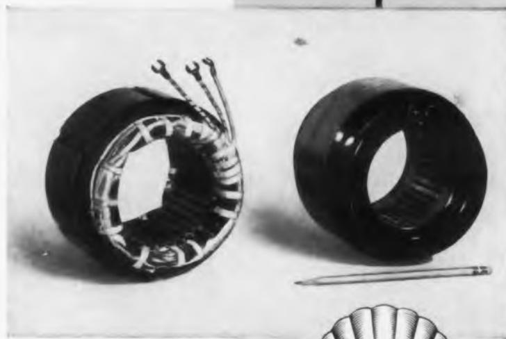
Why not combine the pump and the motor? Put a gear pump *inside* the motor stator, encase the stator in plastic, and you can build an entire motor-compressor in the space occupied by a conventional motor alone!
