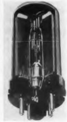
Two mercury-wetter contact relays, the Type HG and HGP, are capable of over a billion operations without maintenance, and are designed for use in high-speed switching machines and devices. These relays will operate at up to 60 operations/sec; have high current-carrying capacity (up to 5amp) and high voltage-handling capacity (up to 500v); are bounce-and-chatter-free; and keep a uniformity of operation to within 1.5milli-sec under constant drive conditions.
