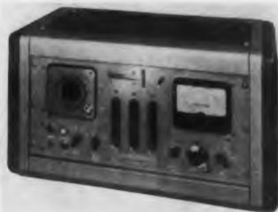
The Model 200 Scaler utilizes decimal or binary units which are directly interchangeable; it may be changed from one to the other in a matter of seconds.
