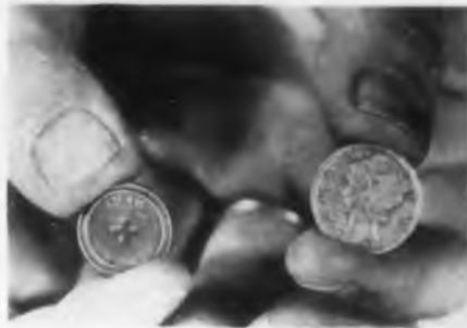
This miniature mercury battery, with an unusually high rating for constant current, power, and service life, is for use in electronic equipment. Called the "General 625", it
