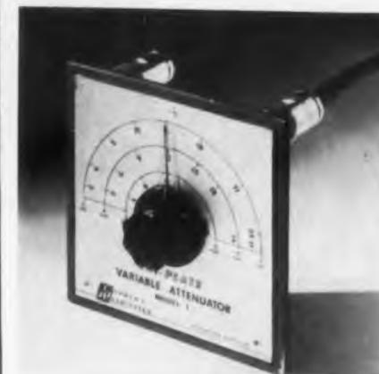
This "Tri-Plate" Variable Attenuator is for use in coaxial lines. The "Tri-Plate" construction makes use of a movable resistive card sandwiched within a new type of printed circuit transmission line.
