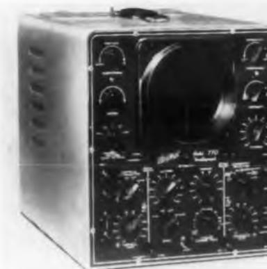
The Model 7500 a 5" wide-range high-sensitivity oscilloscope, has been engineered for maximum dependability. The unit provides a frequency range from d-c to 2.5Mc, with band width switch in narrow position; and d-c to 5Mc, with band width switch in wide position.
