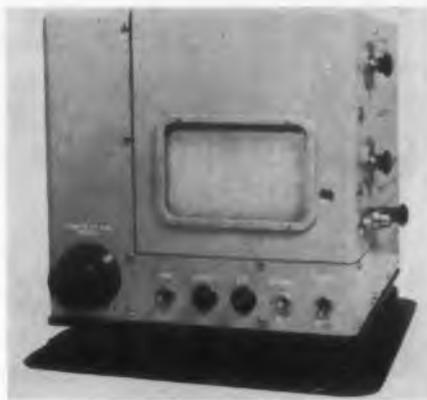
The R-1021-D Recorder is a 210-channel fixed-stylus recorder, writing on a 5" width electrosensitive chart. It is a light, compact unit, designed for use on airborne as well as ground applications. It operates
