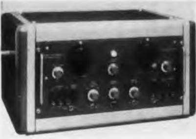
The Audiosweep Generator is an instrument designed to eliminate time-consuming point-by-point plotting of frequency response curves. It presents a frequency response
