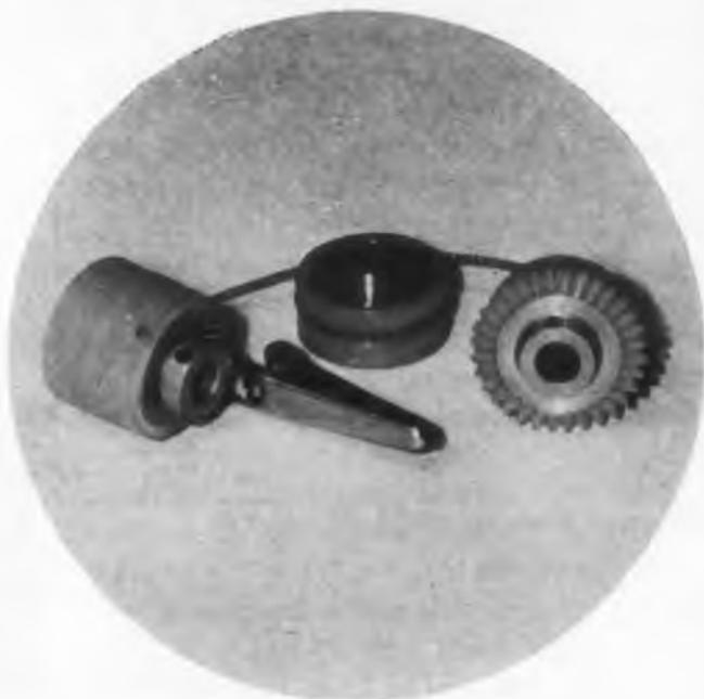
Direct in-line, cable, and gear types use identical clutch bodies. Size is indicated by alligator clip.
