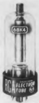
The 6BK4 is a low-current beam triode of the sharp-cutoff type designed specifically for voltage regulation of high-voltage, low-current, d-c power supplies in color TV receivers. It has a maximum d-c plate-voltage rating of 25,000v, a maximum d-c plate-current rating of 1.5ma, and a maximum plate dissipation rating of 25w.
