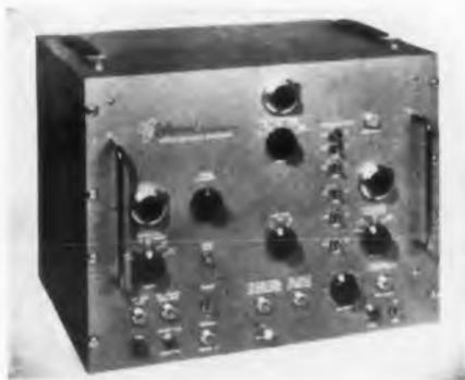
The Model B-2A Pulse Generator is a general-purpose instrument giving repetition rates from 10cy to 100-ke, widths from 0.1μsec and delays from 0 to 10,000-μsec, with an output pulse of 40v
