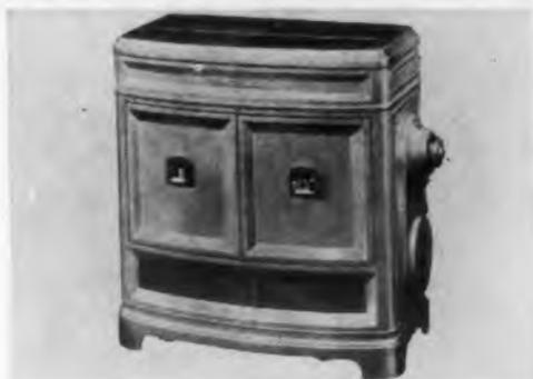
Formulated by Glidden Company, the platinum finish is more durable than any organic finish. It easily passes Duo-Therm's life test of 500 consecutive hours at a surface temperature of at least 450 F. Under the same test conditions, light colored high temperature coatings based on organic resins discolor, crack and flake. The modified silicone coating shows no deterioration.
