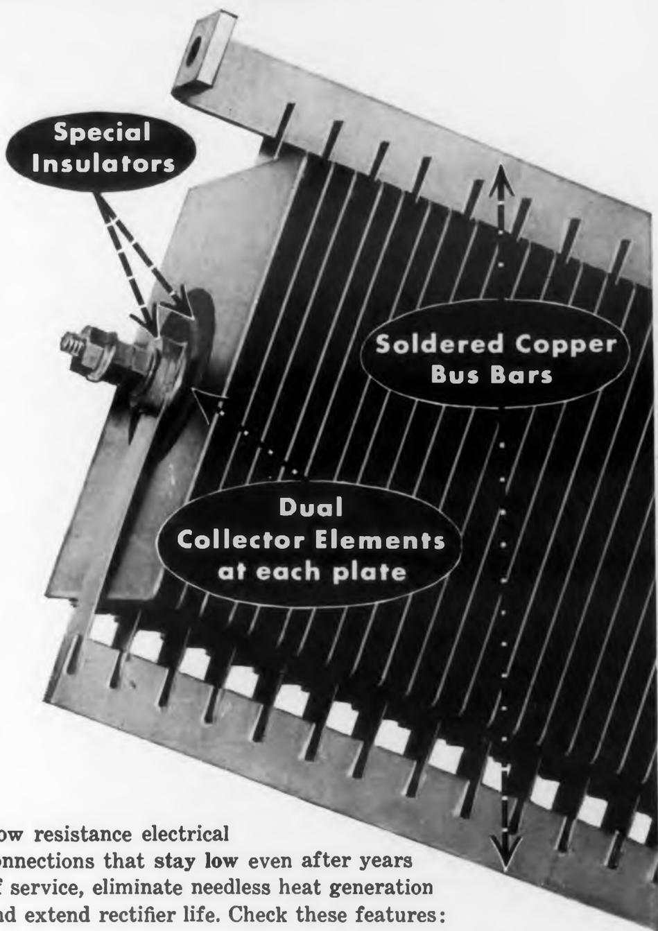
Low resistance electrical connections that stay low even after years of service, eliminate needless heat generation and extend rectifier life. Check these features:
