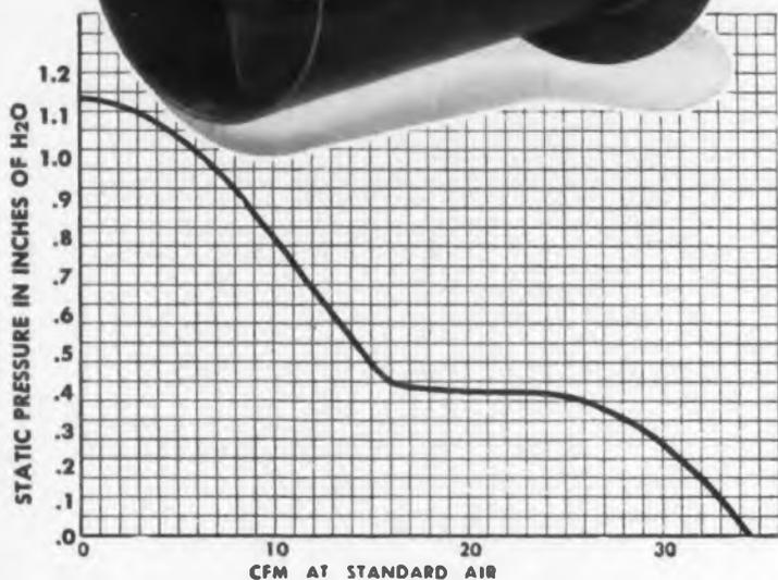
For efficient, spot cooling of electronic equipment, for air change in small equipment-filled boxes, it's EAD's miniature tube axial blowers, driven by EAD's new one-inch diameter motor. These light weight, long life units have no brushes . . . no arcing . . . no radio interference. They meet applicable MIL specifications for aircraft use.
