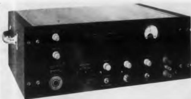
The Model D-1 Direct-Coupled Amplifier can be used for many applications formerly requiring specialized instruments. Maximum useful overall gain is 80,000, while frequency response flat from zero to more than 100kc is available at gain settings up to 10,000.
