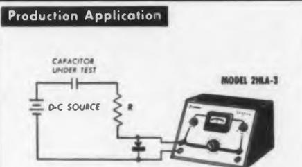
Measuring the dielectric leakage current of capacitors.
