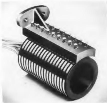
"Eldec" standard slip ring and spring loaded brush contact assemblies are available in 10 combinations of either 2, 4, 6, 8, 10, 12, 14, 16, 18, or 20 silver rings, 4μinch finish, with 1, 2, 3, or 4 silver graphite brush contacts
