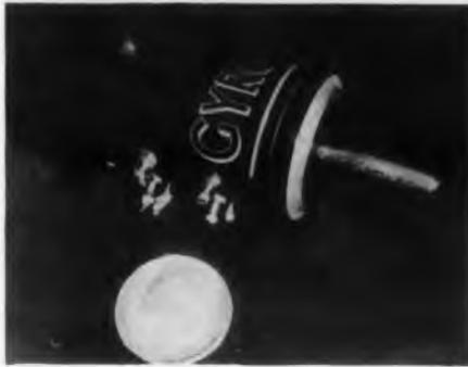
The Model 36000 miniature low torque precision potentiometer is less than 1" in diameter, yet is as accurate as standard pots up to several times that size. It is designed for either linear or non-linear output functions, with accuracies of  $\pm 0.1\%$  for linear and  $\pm 0.25\%$  for sine or similar functions. Initial length is 0.8" max, with an increase of 0.35" per extra section.
