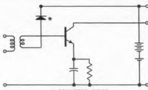
Fig. 4. Diode stabilization with steady power supply.
