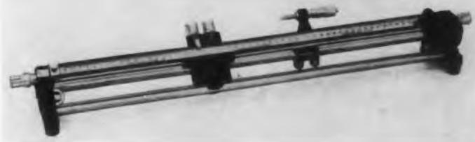
Operating over the frequency range from below 300Mc to 5000Mc, the Type 874-LBA Slotted Line is a convenient and accurate instrument for measurements of impedance, standing-wave ratio, and attenuation. Measurements on dielectric materials, lumped components, coaxial elements, and networks, and antennas in the u-h-f range can be made.
