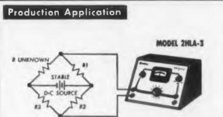
Production testing of precision resistors or potentiometers in a balanced bridge circuit.
