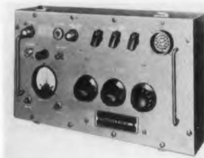
The Model 592 Standard Voltage Ratio Comparator is used for setting accurate voltage ratios, both a-c and d-c, by means of an accurately calibrated voltage divider network
