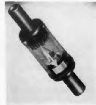
The Type 1N263 is a hermetically sealed germanium crystal diode specifically designed for exceptionally low noise performance in the X-band. This crystal is capable of superior performance at any frequency below 12,000Mc. It may be used for wide-band mixer appli-
