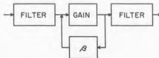
Fig. 17. Stabilization of lumped elements by feedback.
