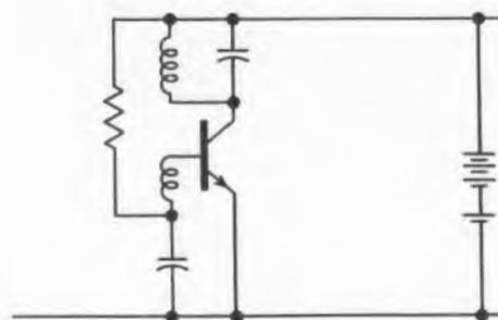
Fig. 18. Fixed base current insures oscillator starting.
