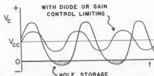
Fig. 20. Effect of carrier storage on oscillator frequency.
