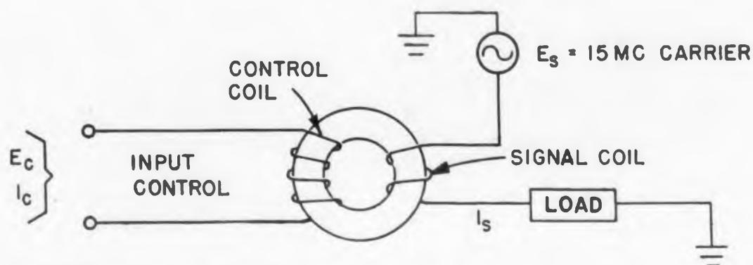
Typical Magnistor gate circuit connections showing control and signal coils.
