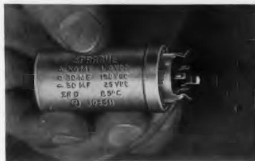
"Push-Lok" 28D dry electrolytic capacitors have a mounting design which makes assembly-line connection in printed wiring boards easier, faster, and fool-proof. They are mounted merely by inserting their connecting lugs into the slots. Strong spring action of the lugs can hold relatively heavy capacitors in place securely until the chassis is ready for dip soldering, even when the board is carried sideways or upside-down on a conveyor.
