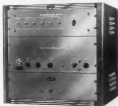
The CPA-1 Color Phase Analyzer is designed to analyze the chrominance components of composite color video signals. The unit compares the phase of chrominance components with respect
