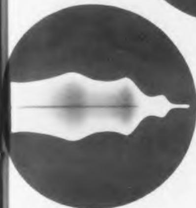
Three typical readings as seen on the Wobbulator's oscilloscope. The top photo concerns a double-tuned input circuit of a cascode amplifier. The second photo shows the image response of a 54Mc receiver with a 21Mc i-f of 2Mc bandwidth. The bottom photo indicates an improper coaxial line output termination on a v-h-f distributed amplifier.
