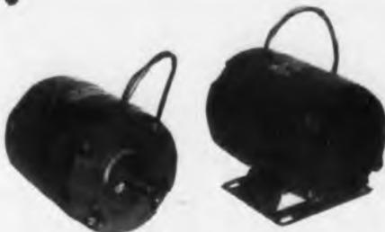
Beefed-up design and built-in "air conditioner" give low temperature rise with ratings up to 1/6 hp in a frame only 4 1/2" OD x 5 1/2" long—Frames and End Brackets, heat-treated aluminum—Ball Bearings shielded, type ABEC-1—Rotor Shaft precision-ground special-analysis carbon steel—Stator insulated silicon-steel laminations, hydraulically riveted, accurately ground; heavy formvar-type magnet-wire windings, double vacuum-impregnated—Rotors:
