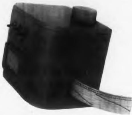
This recorder is designed for accurately recording temperature, pressure, humidity, torques, and other electrical and physical properties. It is particularly adaptable for recording of the analog computers outputs and production process information.
