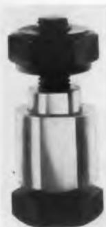
This "D" shaped radio chassis punch is designed to facilitate the punching of holes for mounting miniature sockets having a flat on their shanks. Sockets mounted in this manner cannot twist in the chassis and may be located in any convenient position.
