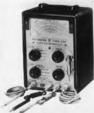
The "302 Polymer" is a vacuum tube voltmeter that offers a subminiature vacuum tube r-f probe, a peak-to-peak scale, a new 7" meter movement, a lighted scale, a patented linearity circuit, an input impedance of 17 megohms, shielded a-c and r-f leads, and screw-on connectors. The brushed aluminum
