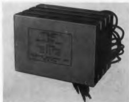
This Encapsulated High Voltage Power Supply is designed for aircraft installations meeting the requirements of MIL-E-5400. It operates from a 115v 400cy source, and delivers
