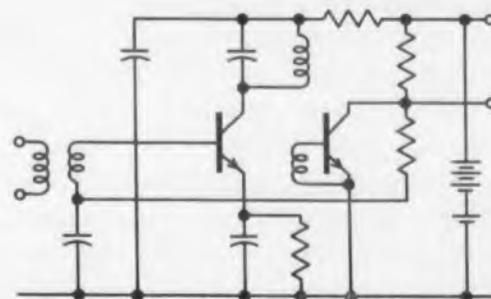
Fig. 12. Combining  $I_e$  and  $V_c$  for avc action.
