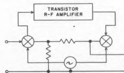
Fig. 25. D-c amplification by carrier techniques.
