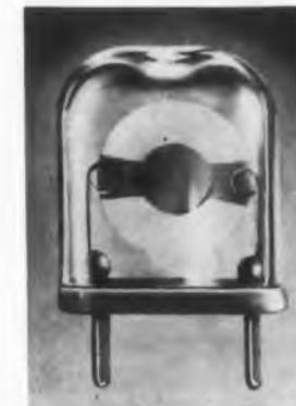
The "Cryst-O-glas" quartz crystal unit features an all-glass case and holder, providing a perfectly hermetically sealed container. Because heat alone is used in the bonding operation, the crystal itself is never subjected to the chemical fumes given off by conventional sealing compounds. This absence of contamination re-
