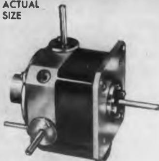
An extremely compact unit measuring only  $1\frac{15}{16}$ " high,  $1\frac{3}{4}$ " wide and  $2\frac{1}{8}$ " long. It combines the functions of a ball and disc integrator and a spherical resolver. Will integrate the sine and cosine functions of an angle or resolve a vector displacement into its horizontal and vertical components.
