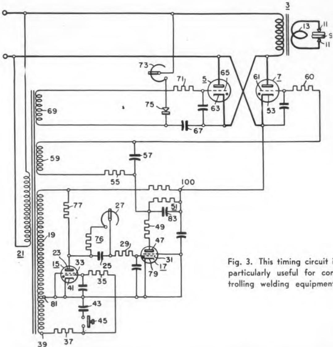
Fig. 3. This timing circuit is particularly useful for controlling welding equipment.
