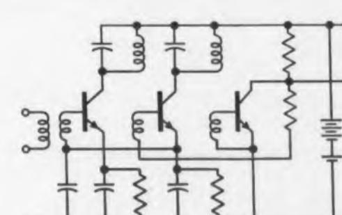
Fig. 13. Gain-controlled i-f stage as current amplifier.
