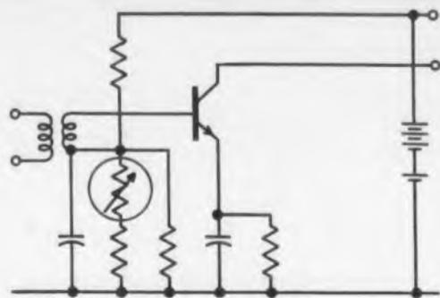
Fig. 6. Thermistor absorbs excess cut-off  $I_e$ .
