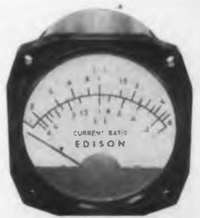
This panel meter has the capacity to handle 50ma in either coil, and will accurately indicate a ratio on an input of 2ma minimum. Scale tolerances are based on an angular tolerance of 1°.
