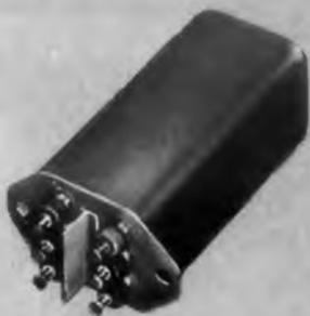
Modulation of DC voltages is achieved by the illumination at line frequency of the photo-conductive element in a voltage divider.
