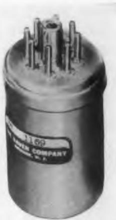
These hermetically sealed wire-wound resistance and resistance-capacitance networks can be supplied with resistance values to  $\pm 0.02\%$  and temperature coefficients matched to within  $\pm 3$  parts per million per degree centigrade. The networks are encased in "Sealed-Ohm" cases with plug-in or solder terminals.
