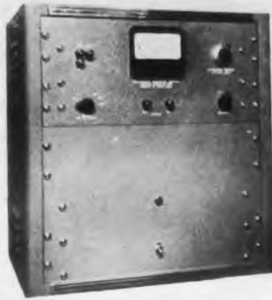
The PS-171 Power Supply was developed expressly for use in high accuracy transistor measurements. The regulated output current of 1-amp max is high enough to accommodate power transistors; in addition, its regulating characteristics and wide range make it useful in many other applications where constant current or voltage source is needed. It has seven regulated current ranges from 1ma to 1amp and four regulated voltage ranges from 10v to 100v.
