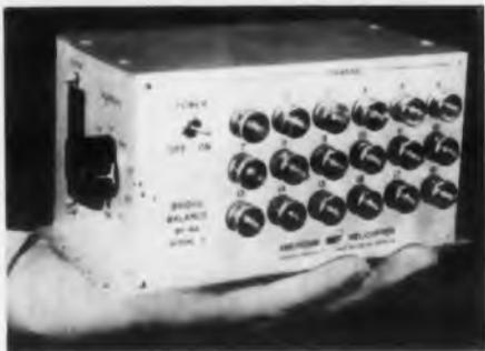
The Model BP-18A Eighteen Channel Bridge Balance has provisions for controlling the electrical balance, sensitivity, and calibration of resistance bridge sensing devices,
