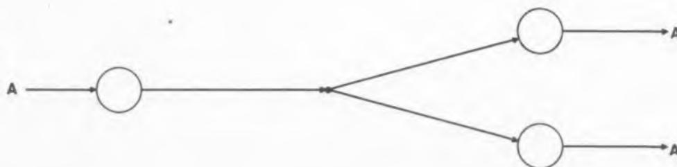
Fig. 5. A magnetic-core branching circuit for a high-speed logic.
