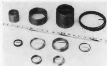
These wire thread inserts of extra-large pitch diameter and wire size provide strong, permanent threads in soft materials such as aluminum, magnesium, plastics, and wood, as well as in iron and steel. Inserts in standard stock sizes run from 4-40 up to 1-1/2-12, serving most applications. Special inserts have been formed up to 6-11/16" diam with 12 threads per inch.
