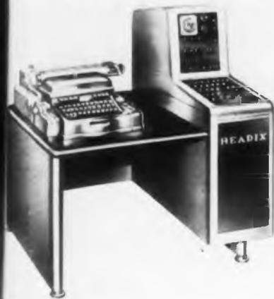
The "Readix" is a decimal, serial, single-address machine with a magnetic storage capacity of 4000 words. Each word consists of 10 decimal digits with sign, or two commands, complete with addresses. Use of the decimal system
