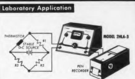
The fast thermal response of highly sensitive thermistors can be accurately measured and recorded.
