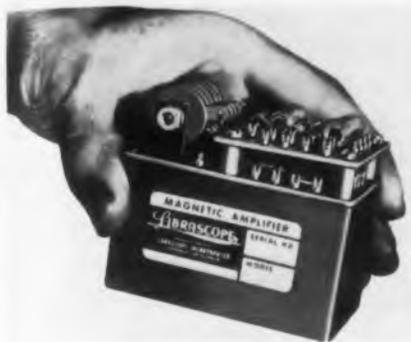
The "Constrained Bridge" Magnetic Amplifier features high power efficiency, low quiescent power consumption, and freedom from zero drift due to change in rectifier characteristics. The unit
