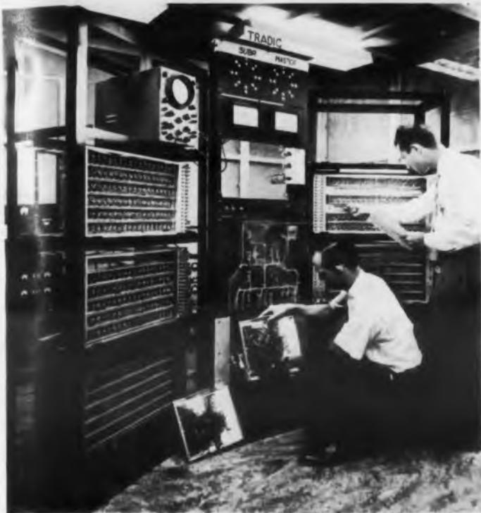
J. H. Felker is inserting instructions in this laboratory version of "Tradic" by means of a problem patch board while J. R. Harris places numbers into the machine by flipping switches.
