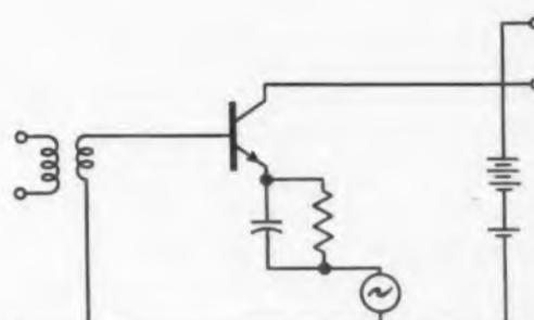
Fig. 9. Converter bias obtained from "emitter bias".
