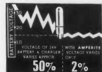
Amperite Regulators are the simplest, most effective method for obtaining automatic regulation of current or voltage. Hermetically sealed, they are not affected by changes in altitude, ambient temperature ( $-55^{\circ}$  to  $+90^{\circ}$ C), or humidity. Rugged; no moving parts; changed as easily as a radio tube.
