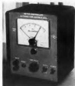
Almost any electrical indicating or recording instrument can be quickly converted into an automatic controller or monitor using the Model 360 Meter Controller. Such quantities as radiation, pH, pressure, flow, strain, vibration, and voltage can be caused to actuate alarms, counters, or complete closed-loop control systems upon approaching or deviating from preset limits.
