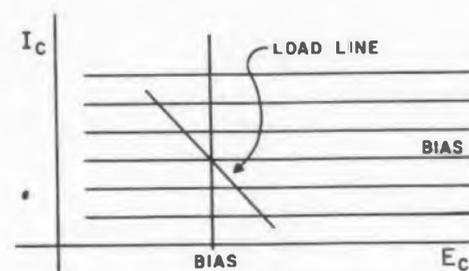
Fig. 23. Very linear characteristics for small signals.
