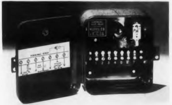
The Model EB Electronic Pilot Relay is able to control large values of current and power with a current flow of 2μamp. It permits delicate mechanisms with extremely light contact pressures to control larger electrical currents. Its unusual cold cathode triode tube design and construction gives instantaneous action, unlimited lead lengths, and a current amplification up to 2.5 x 10<sup>6</sup>.
