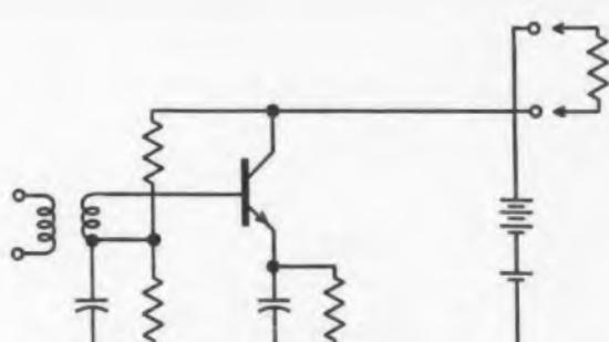
Fig. 8. D-c voltage feedback to stabilize  $I_e$ .
