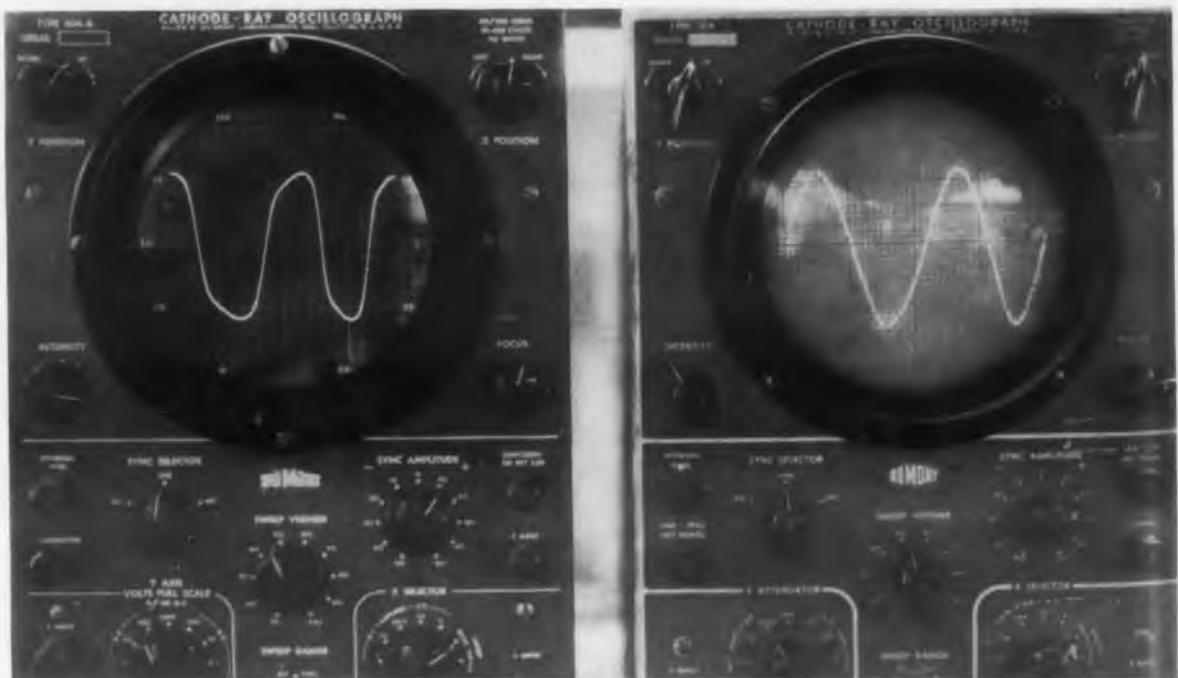
Before and after waveforms show effect of Harmonic Eliminator.
