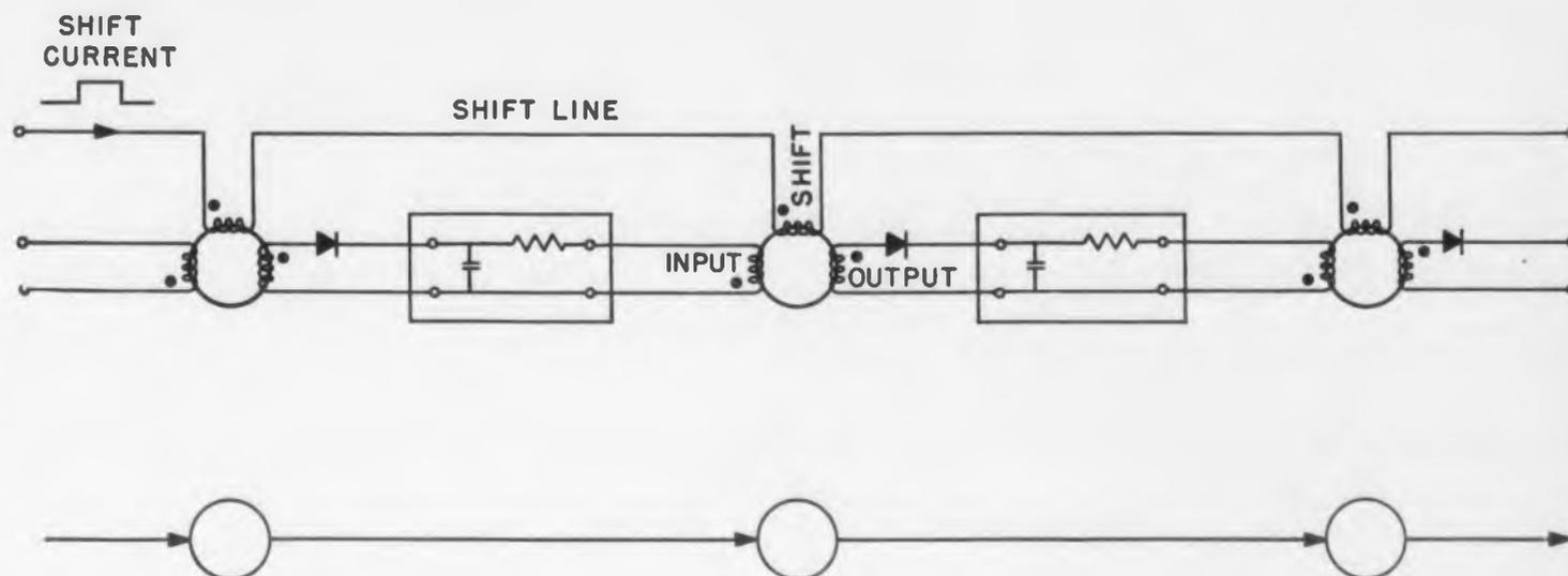
Fig. 3. The "Single-Line" shift register and its symbolic representation.
