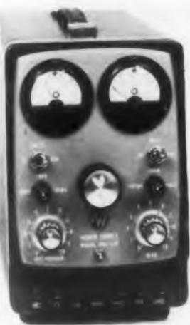
The Model UHR-220 is a compact (7-1/2" wide x 10" high) power supply for applications requiring ultra-high regulation, extremely low ripple, and unusual stabilization under severe input line voltage transients. The regulation of 0.001% applies over the entire operating range.
