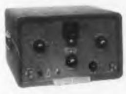
**-hp- 202A Low Frequency Function Generator.** Convenient, highly stable, multi-purpose source of transient-free test voltages from 0.008 cps to 1,200 cps. 5 bands, distortion less than 1%, provides sine, square or triangular waveforms. 30 volts peak output, frequency response flat within 0.2 db. \$465.00 $\Delta$ .
