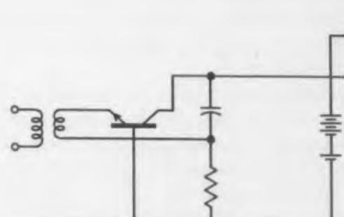
Fig. 15. Stabilization from a bridge-type connection.
