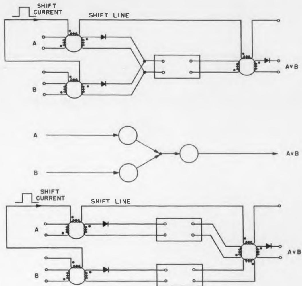
Fig. 6. High-speed logic mixing or buffer circuits utilizing magnetic cores.
