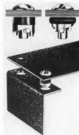
Expanding rubber provides a sturdy, locking mechanism for the multi-function "Vibrex" Fastener. The use of rubber results in a combination quick-action fastener and vibration isolator. Floating the assembly in live rubber, the fastener effectively suppresses noise, rattles, and vibration.
