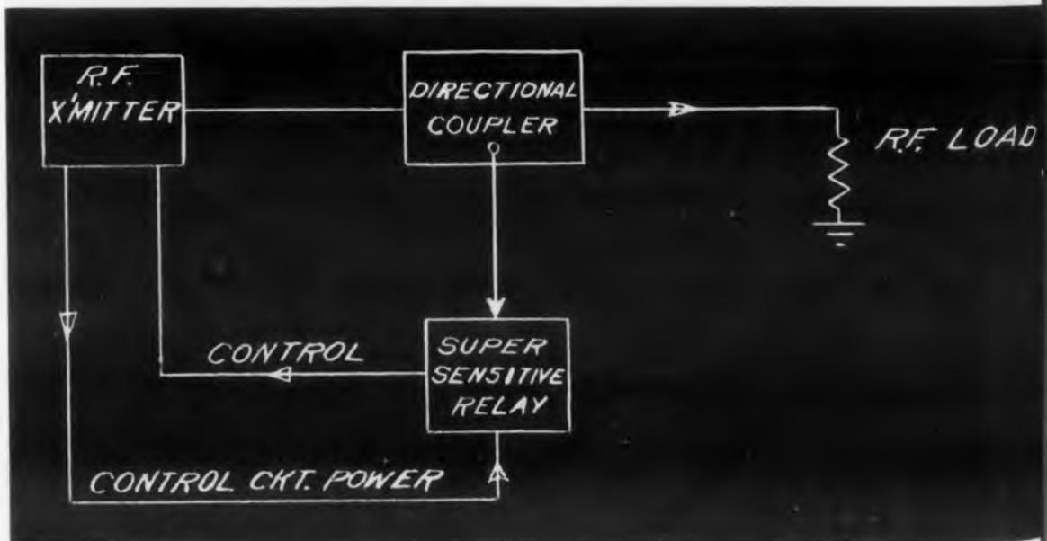
The relay shuts off the transmitter if load mismatch rises above a set level.
