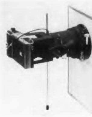
Some applications include sonic analysis, TV signal certification, and TV transmission quality control, in addition to conventional uses. The camera is designed to mount on any scope type electronic device having a 5" tube and a bezel measuring 5-5/8" OD. It offers a single image per print of a high quality due largely to the special f/1.9 oscillo-anastigmat lens.
