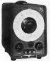
**-hp- 200CD, 5 cps to 600 kc.** Probably America's fastest selling precision audio oscillator. Offers highest stability, constant output, year after year dependability. 5 ranges, frequency response  $\pm 1$  db, distortion less than 0.5%. Compact, weighs only 22 lbs. 300° logarithmic dial, 60" effective scale length. \$150.00.
