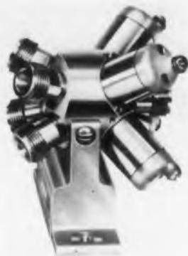
This miniature broad-band r-f coaxial switch permits switching of four circuits by remote control. Only 12 oz in weight, it occupies only 3" x 3-1/2" x 2-1/2" space, thus providing designers wide latitude. Performance is excellent for frequencies up through the X-band.
