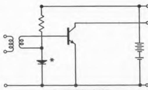
Fig. 5. Junction diode for temperature compensation.
