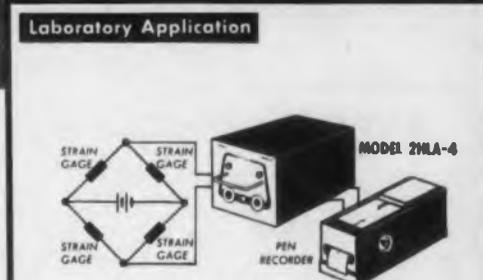
Dynamic stress measurements made with linear response up to 20 cps.
