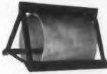
coils virtual "standards" for industrial and broadcast use. Essentially airwound, with slotted, glass bonded mica supports, their open construction provides exceptional current carrying capacity for their size. Extremely compact due to edgewise copper windings—they're economical, easy to mount and offer a choice of inductances from 8 to 320 uh. Nominal 10, 15, 20 amp. ratings.
