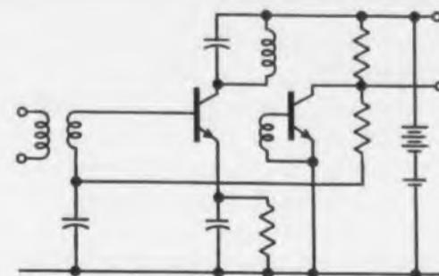
Fig. 11. Variable input voltage to base for avc.
