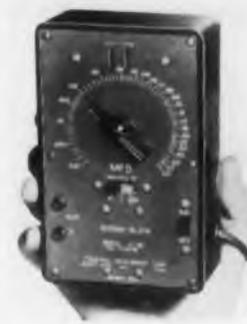
Capacitance Bridge Model C-10 has been added to the line of "Signa-Glow" instruments. It incorporates a newly designed visual null indicator consisting of a pair of glow lamps which indicate both the degree and direction of unbalance at a glance.
