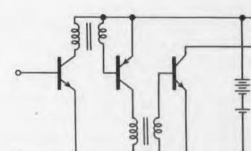
Fig. 14. Compensation for alpha change with temperature.
