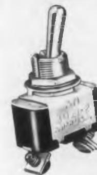
Originally designed to meet the requirements of Air Force—Navy Aeronautical Standard AN-3021, in conformity with specifications MIL-S-6745, these aircraft toggle switches are available in 2- and 3-position models. They are 1-1/8" long x 5/8" wide x 1-3/64" high. Arrow-Hart & Hegeman Electric Co., Dept. ED, 103 Hawthorn St., Hartford 6, Conn.
