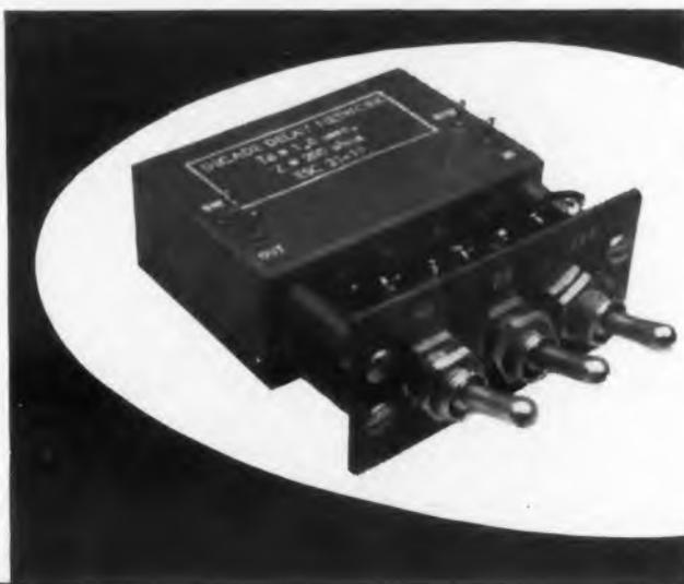
\* Custom-made to precise specifications, this new, compact decade pulse forming network (Model #21-19) provides pulse formations from .25 usec. to 2.0 usec. in width by means of three miniature toggle switches. Embedded in epoxy resin and hermetically sealed, the entire assembly comes in a dust-proof case and is finished in accordance with MIL-T-945A Salt Spray & Humidity Conditions.
