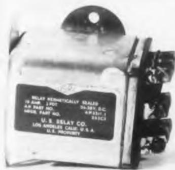
An AN-approved 3311-1 relay for military use, this unit is a dpdt, hermetically sealed device with eight screw terminals. Nominal coil voltage is 24-28v d-c. Rated load (contacts) at 29v d-c is 10amp resistive; at
