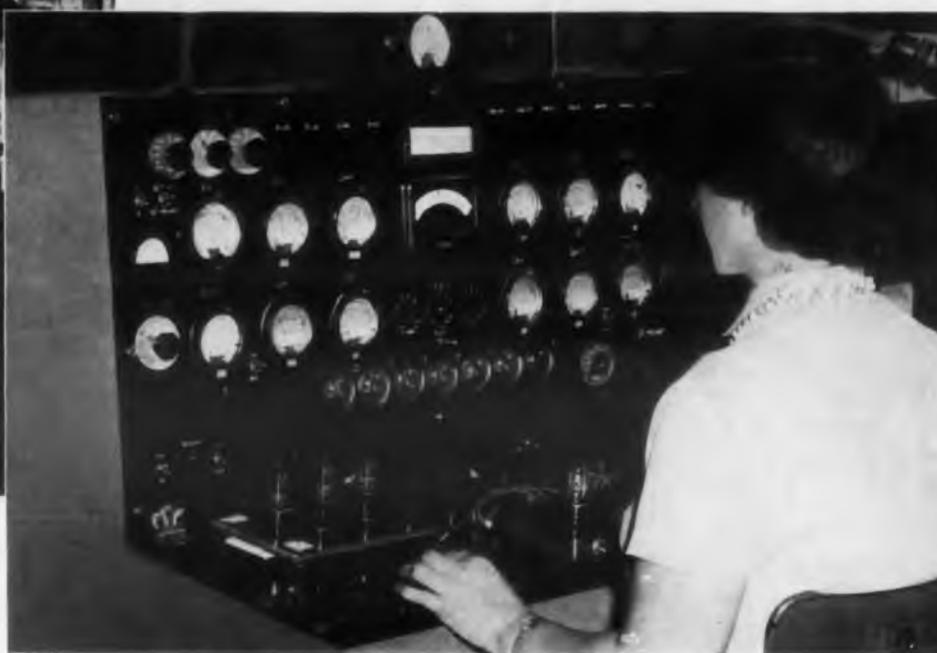
RIGHT: extensive instrumentation is used to test tube electrical qualities that closely affect operation in computer circuits. Zero-bias plate current; cut-off performance; any difference in cut-off between twin-triode sections—these are three of many characteristics checked. ▶
