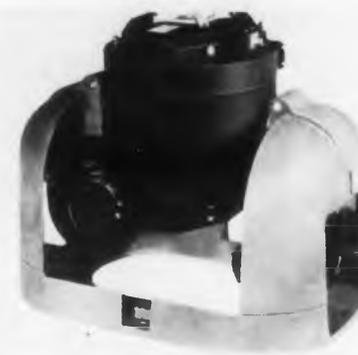
The "68" Electrodynamic Shaker-System, for vibration - testing assemblies and components, is capable of developing 100 lb peak force output over the 40cy to 3000cy range, and dis-
