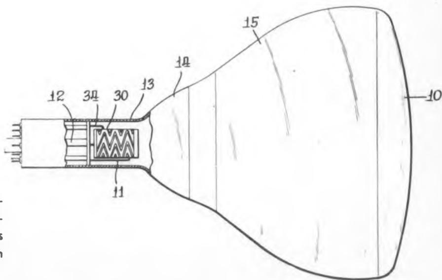
Fig. 2. This cathode-ray tube has electrostatic deflection fields at right angles to each other.
