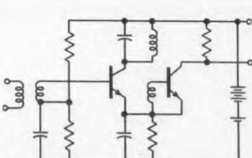
Fig. 10.  $I_e$  varied by detector current for avc.
