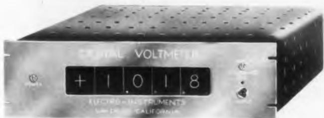
These "Automatic Digital Voltmeters" are designed for reliability, flexibility, and precision. Standard models are available ranging from two to five in-line digits, in voltage ranges from 1mw to 1000v, with automatic ranging indicated by a moving decimal point. Input impedance is 1000 megohms, accuracy is 1 digit, and average time for reading is less than 1sec. Models may be specified to operate printers, electric typewriters, or IBM punches.
