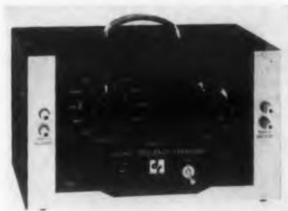
This compact signal generator, the Model F5-1, acts as a secondary frequency standard with a short-time accuracy of one part per million. Generating twelve selected standard
