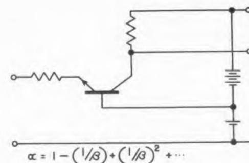
Fig. 24. Criteria for a very stable amplifier.
