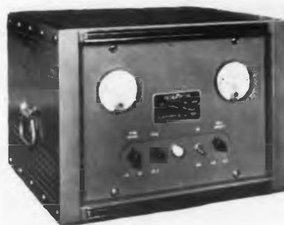
The "Nobatron" Model MA 640 tubeless, regulated d-c supply uses magnetic amplifier principles. Its tubeless circuit makes it highly valuable where accuracy and high capacity
