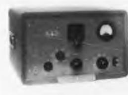
**-hp- 650A Test Oscillator.** Provides fast, accurate tests from 10 cps to 10 MC. Extreme stability; output flat within 1 db full range. Voltage range 0.00003 volts to 3 volts. Output impedance 600 ohms. No zero set, no adjustment during operation. Output voltage attenuator, self-contained VTVM. \$490.00 $\Delta$ .
