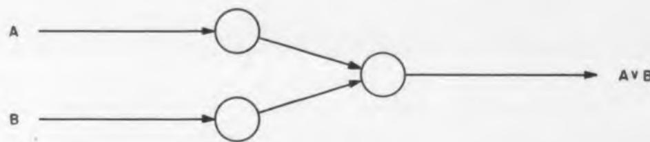
Fig. 7. The "exclusive or" function is readily performed by magnetic core circuits as shown.
