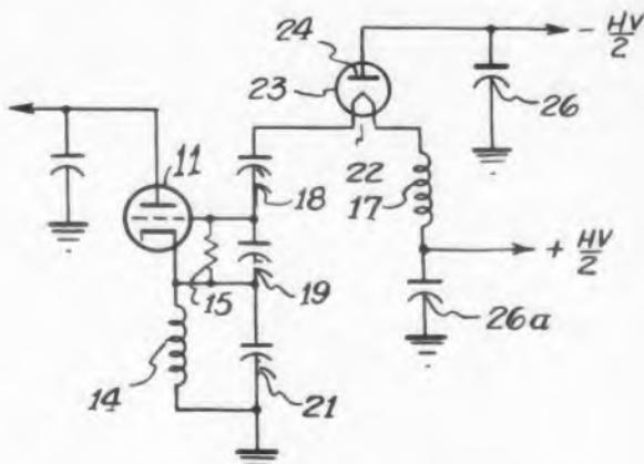
Fig. 4. This high-voltage supply does not require a high-frequency transformer.
