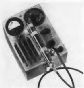
The "Countmaster" is a portable lightweight Geiger counter that permits field assay of radioactive substance and gives an accurate timed count. The unit weighs 7-1/4 lb, including probe and shield.
