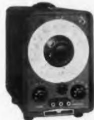
**-hp- 200CD, 5 cps to 600 kc.** Probably America's fastest selling precision audio oscillator. Offers highest stability, constant output, year after year dependability. 5 ranges, frequency response  $\pm 1$  db, distortion less than 0.5%. Compact, weighs only 22 lbs. 300° logarithmic dial, 60" effective scale length. \$150.00.
