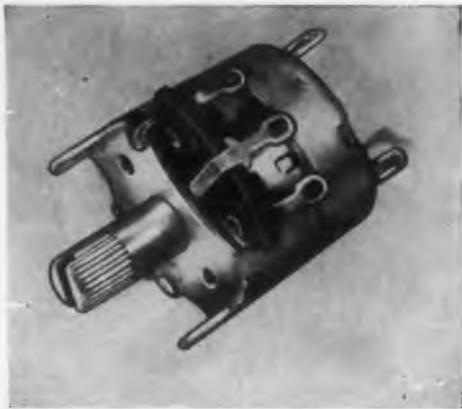
Series 47 controls are designed for twist-ed-tab mounting, resulting in time, labor, and money savings. Materials saving is accomplished by the elimination of such items as bush-
