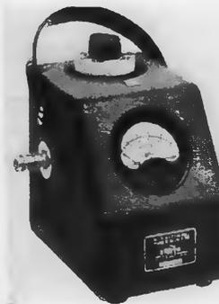
This bi-directional power monitor, Model 164, is designed to simplify measurement of incident or reflected power and to speed matching of loads to line. A twist of the wrist selects incident or reflected power, or any power range, without requiring removal of power. No exchange of plug-in units is necessary
