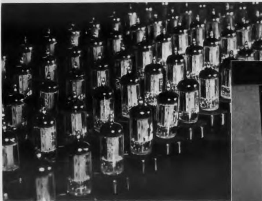
◀ LEFT: G-E computer tubes undergo a cut-off life test. The tubes are operated for long intervals with their grids biased to cut-off. Periodically the tubes are given a cathode interface check, to make sure no "sleeping sickness", or failure to respond to changed grid voltage, has developed during inactivity.
