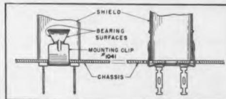
An outstanding mechanical advantage is the clip mounting method, which greatly reduces assembly time. This
