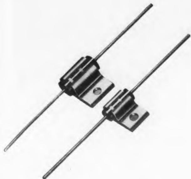
**C**OPPER clamps encircling a standard composition resistor increase its heat transfer capabilities. These copper clad resistors are considerably smaller than wire-wound units of comparable rating and are relatively non-inductive. All standard values and tolerances for composition resistors are available starting at 2.7 ohms in one instance and extending to 22 megohms.
