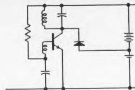
Fig. 21. Diode used for oscillator amplitude limiting.
