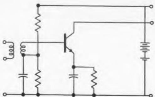
Fig. 2. Bias stabilization from potential divider.
