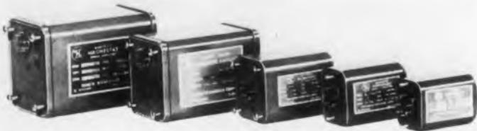
These magnetic servo amplifiers are designed for operation at high temperatures and use no rectifiers. Output power ratings of 3, 6, 10, 15, 18 and 40w at 400cy, delivering voltages of 0-26v, 0-38v, 0-115v, and 0-220v, are available from stock. In addition, 60cy amplifiers are available in similar power ratings.
