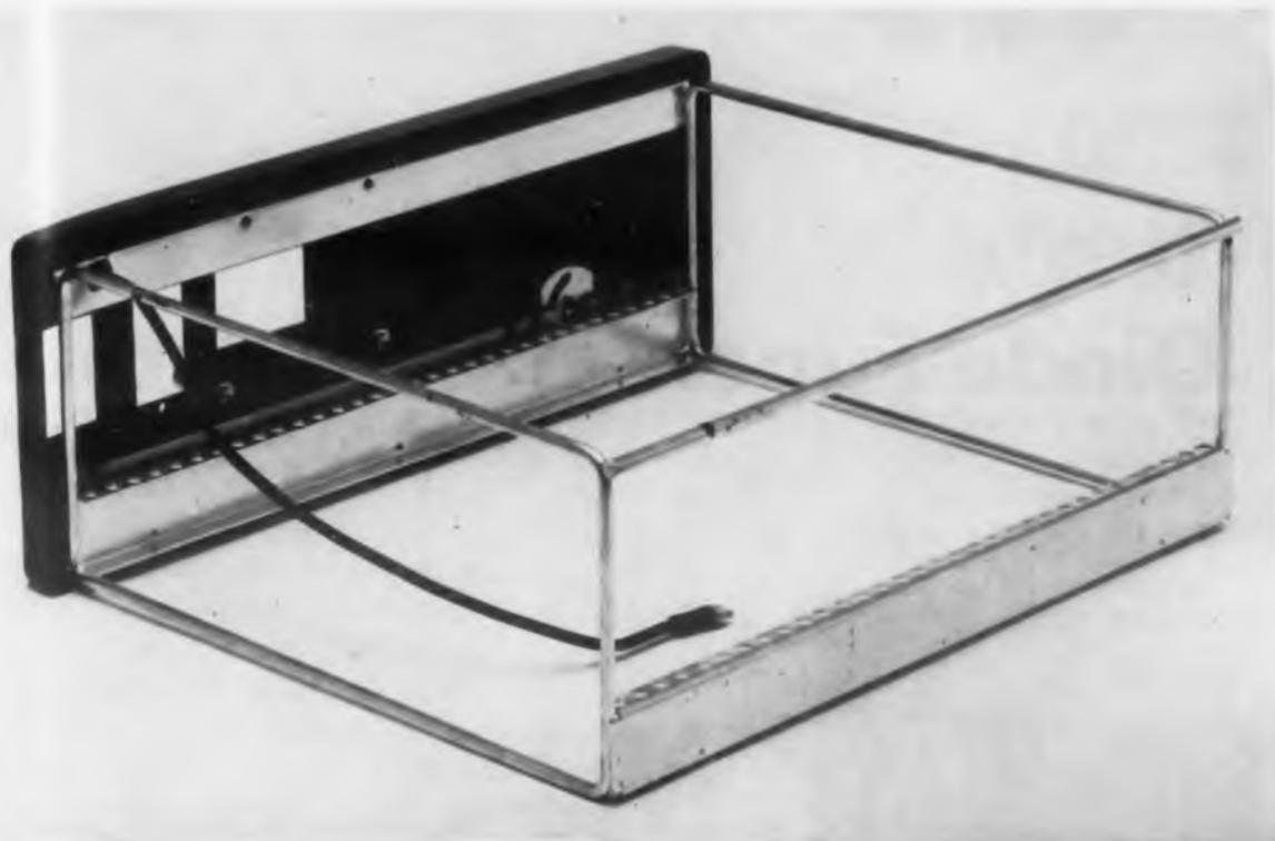
The chassis are mounted in a type of universal relay rack inside the enclosure for greater rigidity.
