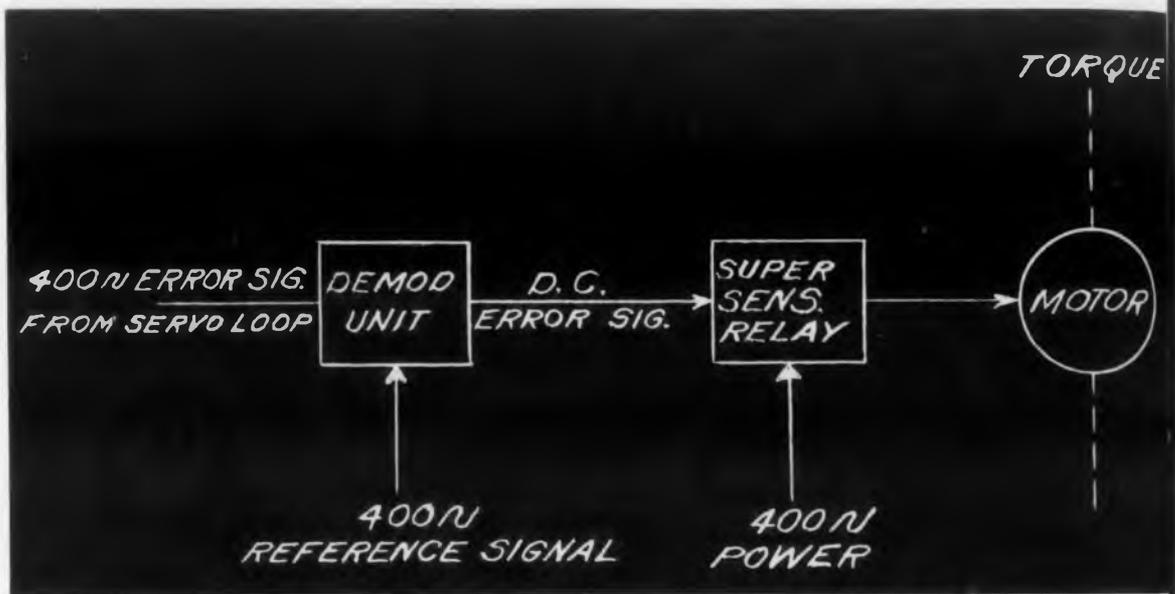
The relay controlling a high-powered motor in a non-proportional servo system.
