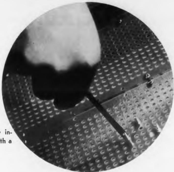
The terminals are easily inserted into the panels with a screwdriver.
