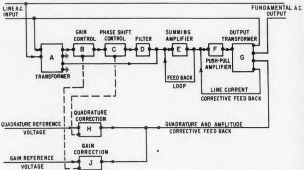
At a 525-w rating this equipment can reduce 10% rms distortion to 0.3% by cancelling line irregularities.
