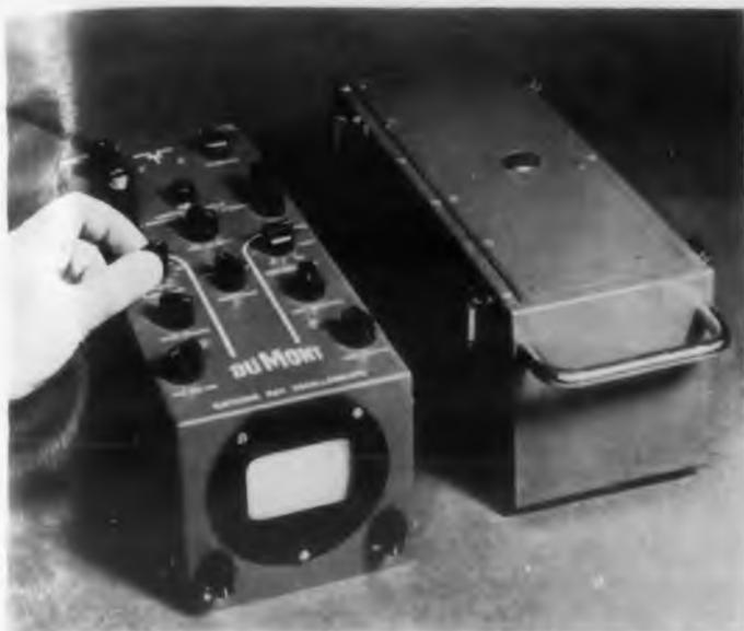
The Du Mont experimental portable oscilloscope and its battery case, which is just as large as the instrument. The entire unit consumes about 5w.
