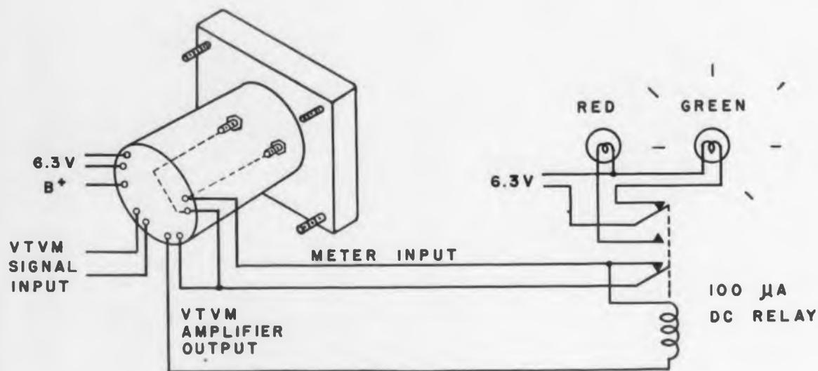
Amplifier section is used for go—no-go indication. Meter switches in automatically indicating exact deviation of rejects.
