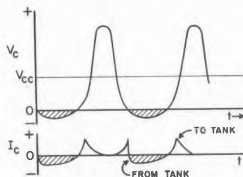
Fig. 19. Clipping by the collector diode.
