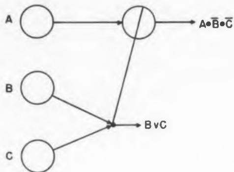
Fig. 4. A magnetic-core inhibit circuit, its symbolic representation, and two other symbolic inhibit circuits are used for high-speed logic in computers.
