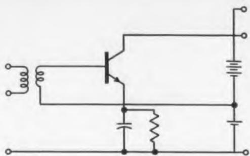
Fig. 1. Split battery current stabilization.
