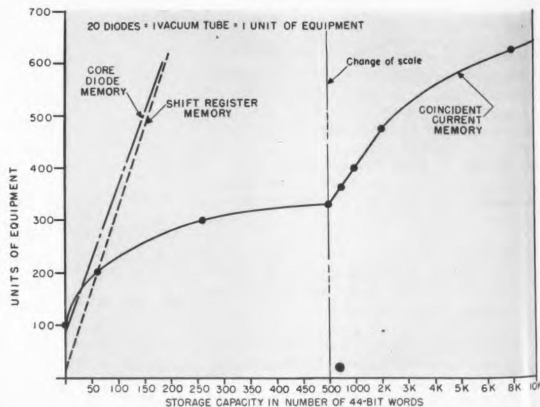
Fig. 1. This chart indicates which type of memory requires the least equipment for a specific size memory.
