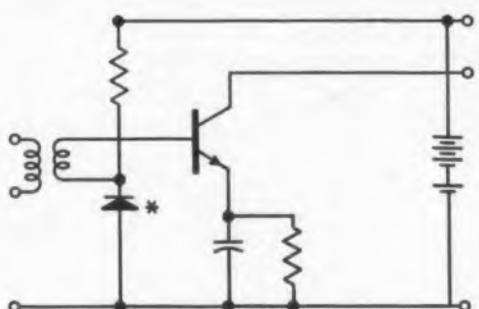
Fig. 3. Townsend diode provides bias stabilization.
