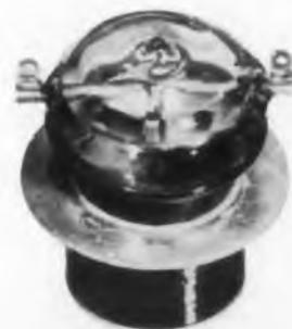
This firm's smallest high-voltage vacuum relay, the Type R5-E, is designed for pulse network, antenna transfer, and guided missile applications. Size is only 3" long x 2" diam, including a 12v or 24v d-c actuating solenoid located in the base.
