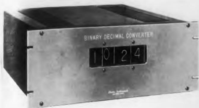
The Binary-Decimal Converter is an electronic instrument which converts binary numbers to decimal numbers. It provides an in-line visual display, as well as control for machine storage of the decimal numbers.
