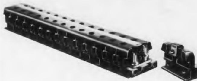
"Pres-SURE-blocks" allow any number of circuit sections to be securely assembled into a compact 70amp, 750v sectional terminal block. One-piece ruggedness of assembled circuit sections is achieved through three integrally molded serrated pins which locate and secure each circuit section by a mating with corresponding holes in the adjoining circuit section. The pins permit limitless circuit sections to be assembled without accessory fastening hardware or loose-fitting sections.
