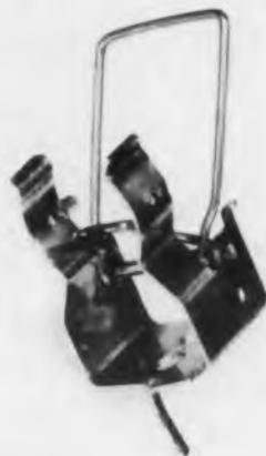
A wide selection of Navy type fuse and resistor clips, that provide positive locking for extreme conditions of shock and vibration, is available. Consisting of silver-plated, phosphor-bronze clasps and passivated, stainless-steel springs, they have an ejector feature which makes resistor and fuse changing an easy matter.
