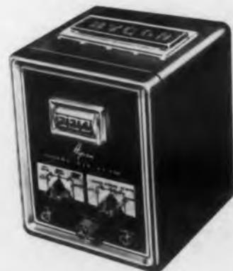
Sensitivity ranges for the Model 615 are from one millivolt to 1,000v and from 1000 ohms to ten megohm, with an accuracy rating of 1% (on d-c and ohms, 2% on a-c). Hycan Mfg. Co., Dept. ED, 2961 East Colorado St., Pasadena 8, Calif. *This product will be on display at the Radio Engineering Show, Booth 735.*
