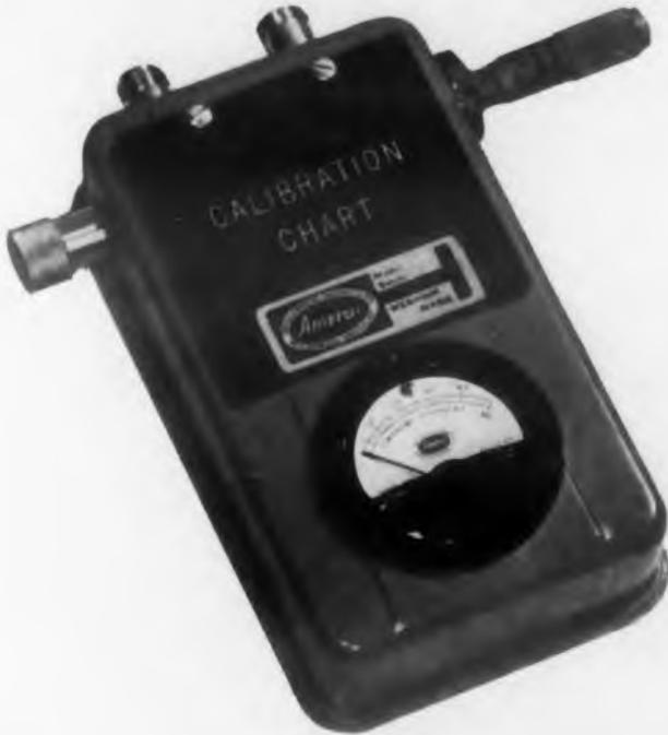
Amerac has now produced a new, inexpensive "S" Band Wavemeter. The model C&D covers the frequency range from 1800 MC to 3800 MC.
