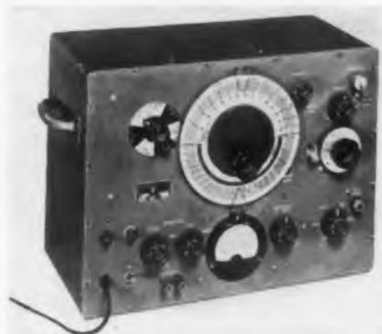
The Model 552 Standard R-F Signal Generator covers the frequency range from 32kc to 70Mc in seven ranges. Signals from less than 1mv to the high voltage requirements of bridge
