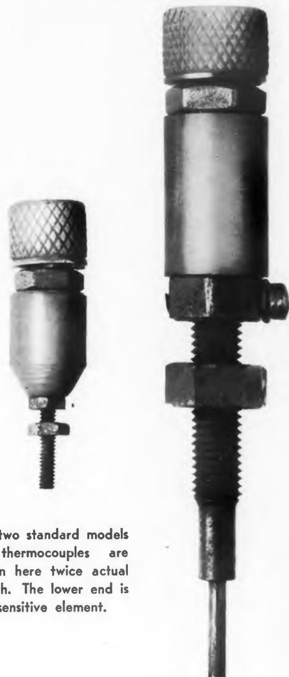
The two standard models of thermocouples are shown here twice actual length. The lower end is the sensitive element.
