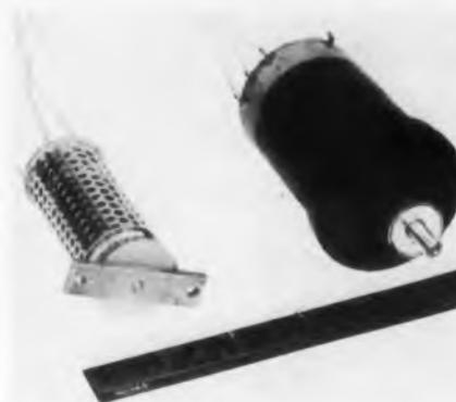
This High Precision Rate Generator is designed to supply a voltage output that is proportional to the speed at which it is driven. Having a linearity of 0.05% up to 4000rpm, the unit may be used
