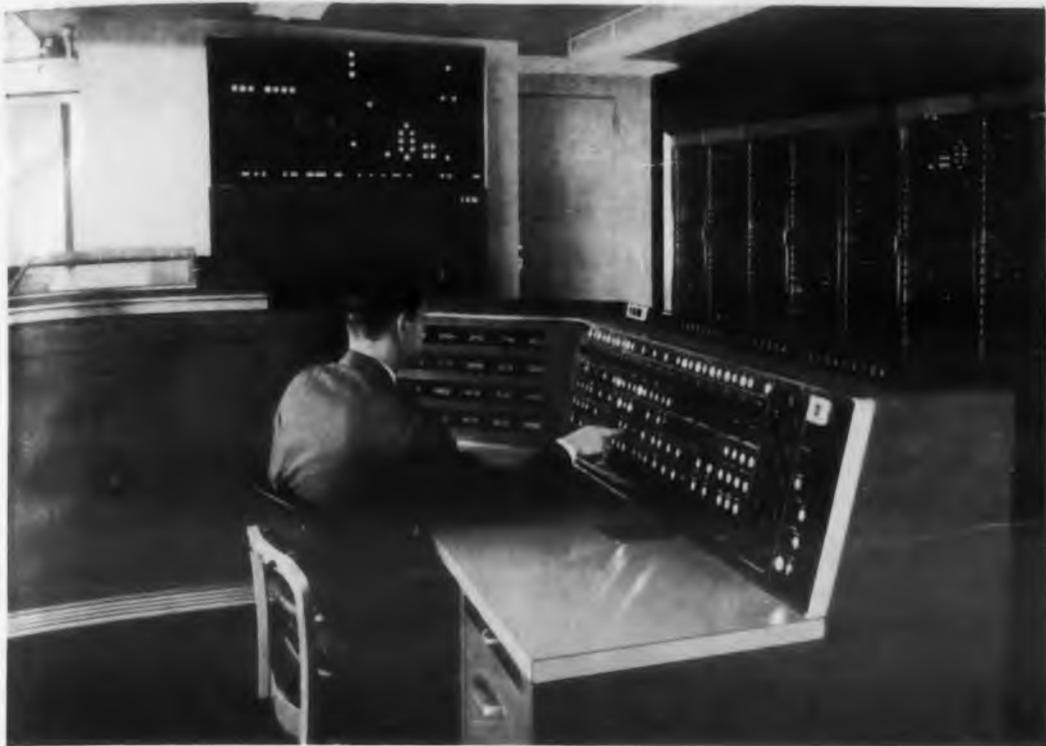
The control area. One of the intermediate-result printers is at the left. The other one is to the right of the console out of camera range. The operator is checking by means of the console's cathode-ray tube display. Some of the calculation circuits are at the right.
