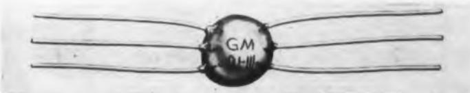
The GM Series toroidal steel core pulse transformers produce rectangular pulses with durations, when operated in this firm's standard blocking oscillator circuit, of 0.05, 0.1, 0.2, 0.5, 1 and 2  $\mu$ sec. Available with two or three windings, they are epoxy resin impregnated and encapsulated, and they are impervious to moisture.
