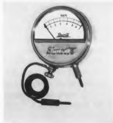
This small pocket type voltmeter is suitable for testing batteries used in transistor type devices such as hearing aids, etc. The instrument is supplied with a nickel plated case, one positive stationary test prod and a negative flexible lead with probe attached. The current drain is in the order of 11-12ma at 7v. Shurite Meters, Dept. ED, 61 Hamilton Street, New Haven 8, Conn. *This item will be on display at the Radio Engineering Show, Booth 205.*
