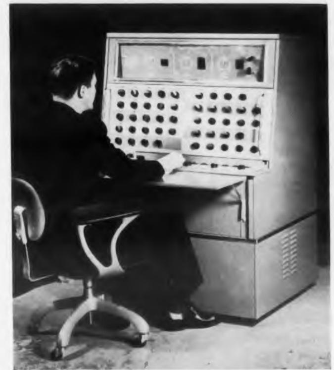
Aeronautical engineers can solve their design problems on this Aerolog analog computer without special training in programming.
