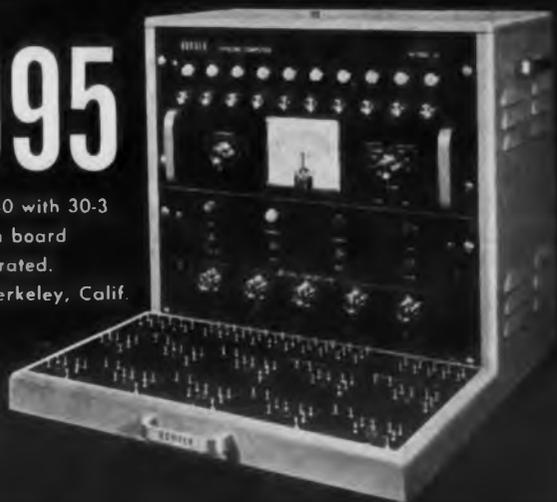
This versatile and compact Donner Model 30 is the first electronic computer specifically designed as a personal tool of the engineer, mathematician and scientist. It offers the speed and accuracy of electronic computation with slide rule operating simplicity wherever differential equations are used.
