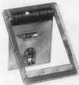
Designated Type H84 and H85, this hinge design permits attachment of any small access cover or door to the exterior skin of aircraft. A major feature is that skin cutout is not required for installation. The unit requires only 0.450" maximum depth dimension below the skin surface for
