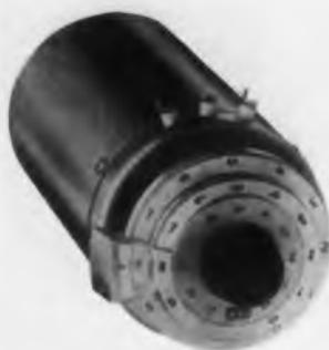
Model 250-DA is an accurate wide-range impedance bridge designed for the measurement of resistance, capacitance, inductance, dissipation factors, and storage factors. It operates directly from an a-c power line. A carefully stabilized capacitance standard unit is included that is adjusted to better than  $\pm 0.15\%$  of its nominal value.
