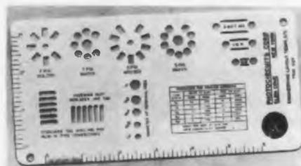
This plastic template facilitates drafting of components for printed circuitry. It is pocket-sized, measuring 4" x 8", and is satin-
