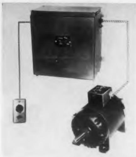
These drives use a tachometer feedback signal to hold speed within desired setting, eliminating critical phasing circuits or adjustments, and at the same time providing close speed-load regulation. Both 1/4hp and 1/2hp Models are available from stock with a choice of either 1800rpm or 3600rpm as the base motor speed. Both motors supply constant torque over a 30:1 speed range.
