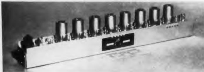
The Series M-200 I-F Amplifier now includes four standard models, with band centers of 30, 23.5, 30, and 60Mc, and bandwidths of 2Mc (3db), 2Mc (3db), 10Mc (3db), and 10Mc (1db), respectively. Maximum gain is greater than 100db on the first two units, and 90db on the second two.
