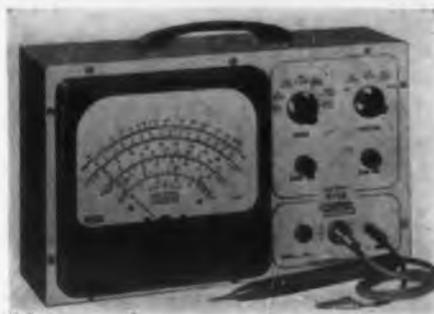
The Model 249 Peak-to-Peak VT-VM is offered either in kit or factory-wired form, and is supplied with the dual-purpose a-c/d-c "Uni-Probe".
