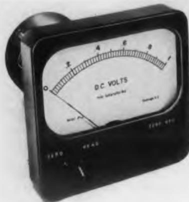
The Model F D-C Vacuum Tube Voltmeter is a miniaturized panel - mounting version of a laboratory instrument. It consists of a standard 4" x 4-1/4" rectangular meter, with a small housing that extends approximately 3"
