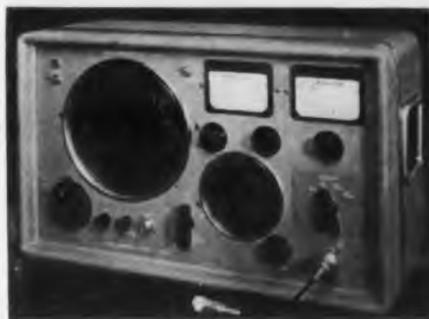
The TF.801B Signal Generator, with a frequency range of 10Mc to 500Mc, has an output range of 0.1 $\mu$ v to 2v and incorporates a piston attenuator.
