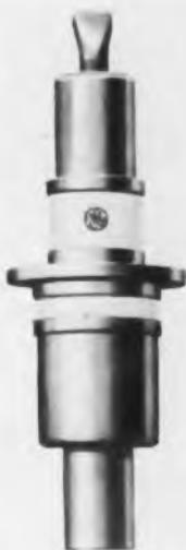
This miniaturized lighthouse tube, the GL-6442, is a 2-5/8" long metal-and-ceramic tube of new design that permits pulsed power applications up to 4000Mc. Peak power output at 3500Mc is 2.0kw.
