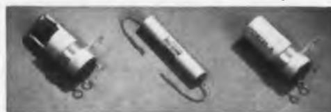
The Tru-Ohm Division of the Model Engineering and Manufacturing Co., of Chicago, has improved its line of wire-wound resistors by using a silicone-based cement that is much more resistant to moisture than the silicate-type cements previously used.
