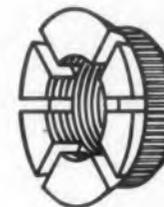
This locknut is a single solid metal piece, with a slotted cone shape on one end and a splined cylinder on the other. It is designed to be inserted in a countersunk hole: the nut is partially or completely seated in material and is held in position by force-fitted splines. After a bolt is inserted, locking action is effected by the pressure of the sector threads forced against the bolt by the interference of the countersinks. Locking action is unaffected by high temperatures.
