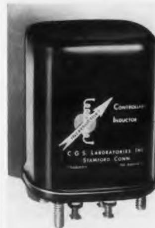
These "Increductor" controllable inductors, designated as the LP series, operate on the principle of saturable reactors but use a direct current to control the inductance of a signal winding suitable for use in high frequency circuits. The series has been developed in response to the increasing demand for more uniform performance characteristics in the supersonic frequency range. A
