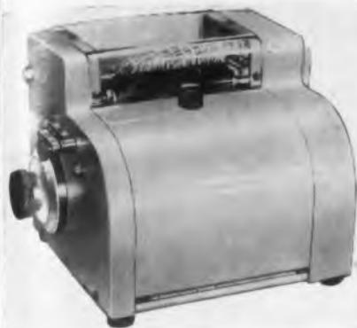
The R-1021-1 Miniature Fixed Stylus Recorder provides 210 channels of On-Off information recorded on a 5" wide "Teledeltos" chart. It is particularly adaptable to events or sequence recording requirements, and can be used as a high-speed digital recording system. A direct-writing instrument, it offers continuously variable chart speeds.
