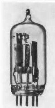
The commercial type "G" series snap-action thermal time-delay relay is provided in a 9-pin miniature glass envelope. These relays feature snap-action spdt contacts, time delays preset from 5sec up, and ambient temperature operation from -60° to +80°C. They are available in 6.3v, 26.5v and 115v a-c or d-c heater ratings.
