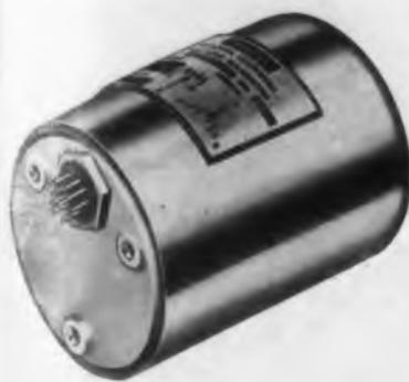
Model 36128 is a high-performance, small-sized Rate Gyro, suitable for use in aircraft and missile control, or telemetering. A rugged, fluid-damped instrument, it is enclosed in a hermetically
