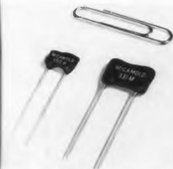
"Micap" capacitors are encapsulated and hermetically sealed by a dip-coating method rather than the usual compression-molding procedure. They are smaller in size than molded types, and are generally
