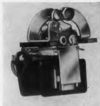
The Series 23 Relay is equipped with a flexible armature and adjustable contacts. The first feature makes the relay ideal for a-c as well as d-c use; the second provides for an easy readjustment after the unit has been placed in service.
