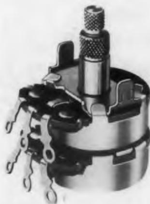
This complete line of variable resistors for all color TV applications includes 3/4" diam "dime size" to 2-1/2" diam controls with wattages from 0.2w to 4w. Control types are carbon and wire-wound, with and without attached switch. Mountings are conventional bushing, twist ear, and snap-in bracket for printed circuits.
