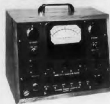
The Model TT-11A Transistor Tester checks NPN, PNP, junction, and point contact transistors, diodes, and other semiconductor devices on a direct-reading "Go, No-Go" basis, and is not obso-
