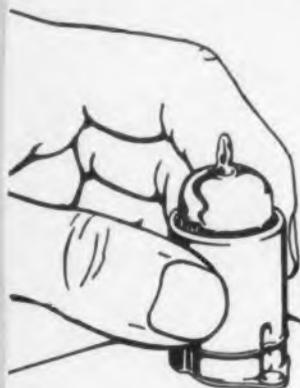
... For easy tube replacement, top half of shield telescopes, exposing tube. Shield is quickly locked back in place.
