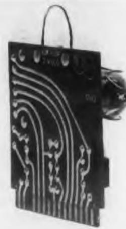
The Z-91000 is a medium-speed bistable multivibrator circuit designed for use in counting frequency division, switching, and time selection applications. Making use of etched circuitry, the unit was designed to provide a low-cost, light-weight, plug-in device. The output of one Z-91000 may be directly coupled into another without the use of amplifiers. The unit is wired so it can be used
