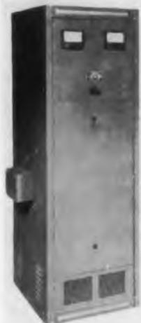
The Model No. MR2432-200 tubeless magnetic-amplifier-regulated power supply is rated 24-32v at 200amp continuous. The unit has a regulation accuracy of 1% (a) from 0-200amp, (b) for the d-c voltage range of 24-32, (c) for a-c input voltage range of 208/230/-460v  $\pm 10\%$ . The ripple is 1% rms maximum; response time is 0.2sec; and the unit is designed for 3-phase, 60cy a-c input.
