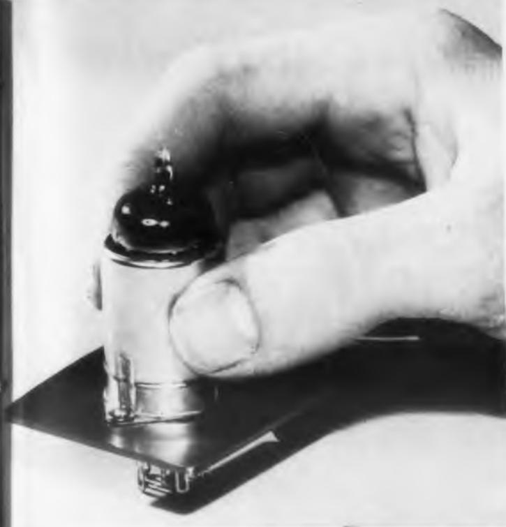
Shield is collapsed over base for tube removal.
