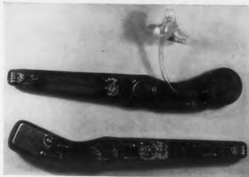
The battery and sound reproducer are mounted in the upper temple, while the microphone, switches, and amplifier are in the lower one.
