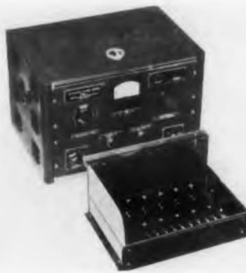
This instrument automatically tests, in sequence, the dielectric strength between any ten conductors and indicates the location of breakdown when it occurs. The test interval can be accurately controlled up to 120 seconds,
