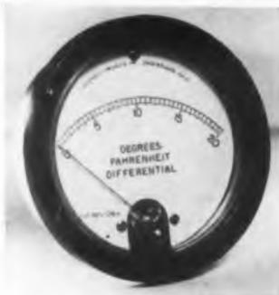
The Model 455 is a ruggedized and sealed 4-1/2" outside diam panel mounting meter conforming to mounting specifications of MIL-M-6A. It is designed to withstand shock, vibration, and other environmental requirements of MIL-M-10304 (Sig C).
