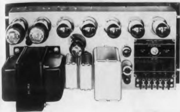
Model 323 is a highly compact 200-325v, 300ma, regulated d-c power supply. Panel height is 8-3/4", and depth behind panel is 9-1/4". Stability is better than 0.1% for line or load variations, ripple less than 1.0mv, and transient response less than 150 $\mu$ sec.
