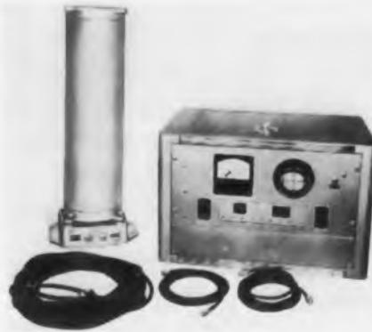
The Model 3 Corona Test Set is designed to facilitate non-destructive testing of the insulation on electrical equipment. This is accomplished by the detection of electric discharges that may result when
