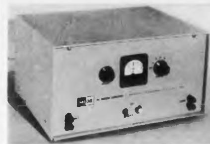
The D-C Decade Amplifier contains a high-gain, wide-band, direct-coupled amplifier operated with negative feedback and frequency corrective networks to
