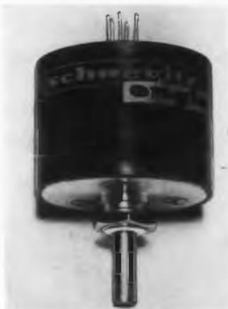
The unit is similar to a linear variable differential transformer, but has a suitably-shaped ferromagnetic cam as its core. This cam is affixed to the shaft, which is ball-bearing mounted, and varies the relative coupling between the primary and the two halves of the secondary as the shaft is rotated.
