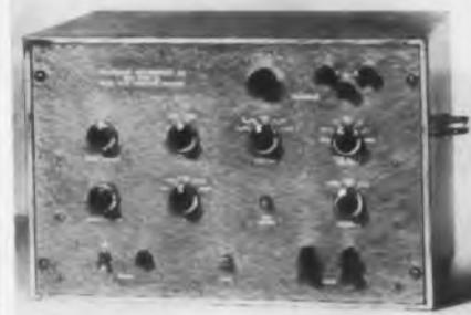
The Model TA-3A Transistor Analyzer, a transistor family curve tracer, displays on an oscilloscope the  $R_{12}$ ,  $R_{22}$ , and  $I_{12}$  families in the grounded base connection, and the
