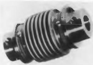
Type No. T1 Precision Bellows Coupling is designed to join shafts of the same or different diameters. It is used where only low torque operation is required. The stainless-steel
