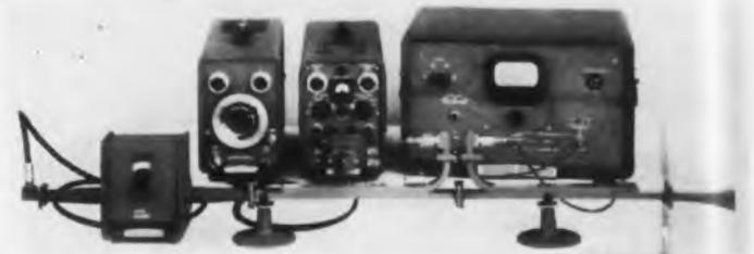
This reflectometer system, when measuring small reflections, has an accuracy that is comparable to that obtained with slotted section techniques, and may be used with sufficient speed to allow investigation of reflection coefficients over a wide frequency range in a few seconds' time. The equipment is now available to form reflectometer systems for the 8.2kMc to 10.0kMc range.
