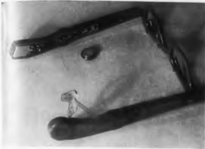
The two "temples" containing the circuitry are connected by three wires running through the frame.
