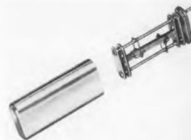
Crystal CR-38/U has a frequency range of 16-100kc; load capacity of 20mmfd; frequency tolerance of  $\pm 0.012\%$ ; and a temperature range of  $-40^{\circ}$  to  $+70^{\circ}$ C. The holder is IIC-13/U. Recommended drive level is 0.1mw.
