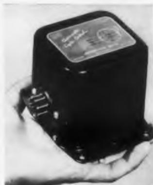
This automatic timer and cycle control sensing device provides a compact, dependable, and inexpensive unit with wide application: (1) for timed quantity measurements in production processing of liquids or solids; (2) for coin-operated vending machines; and (3) for sequential production operation.
