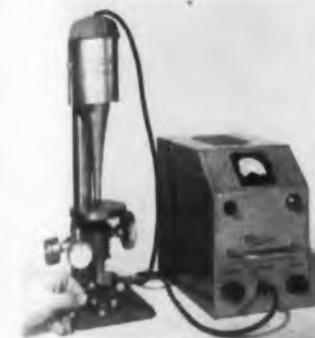
The Model U 600 ultrasonic drill is valuable for such operations as cutting, shaping, grinding, and finishing. It is particularly useful for drilling hard materials as glass, tungsten carbide, sapphire, ceramic, and hardened steel within a tolerance of 0.0005".
