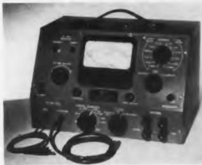
The Megohm-meter and High Potential Test Set measures breakdown voltage and resistance without damage to the component being tested. When a short occurs, current is automatically re-
