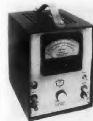
The Model 207A VTVM utilizes a logarithmic meter movement which provides the user with a logarithmic voltage scale and a linear db scale. The accuracy of the log scale therefore is not affected by the position of the pointer, as is the case with instruments which state accuracies as a "percent of full scale".
