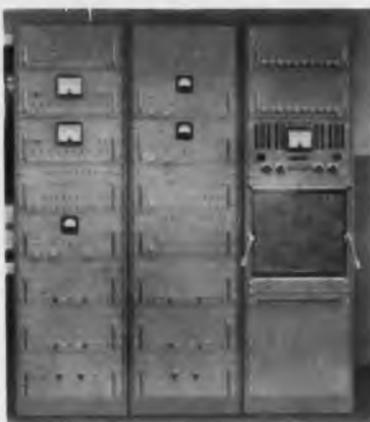
"EASE" (Electric Analog Simulation Equipment) can be used for: systems design, providing fast problem set-up and computer operation; systems development, by simulating part or all of a system for performance prediction; and for system control, providing amplifiers,
