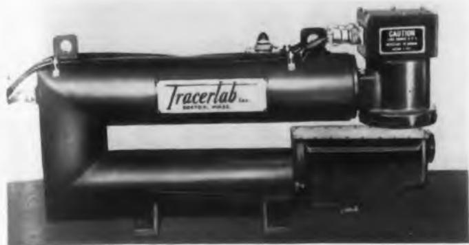
The Light Materials Beta Gage uses a Cesium-137 source, the first gage to utilize this radioactive material. It has lower energy beta rays and a half-life of 33 years, much longer than the approximately two-year source used in older gages. Because low energy beta rays are emitted by the source, much thinner materials can be successfully gaged. The electronic circuitry in the detector head and console incorporates many new features.
