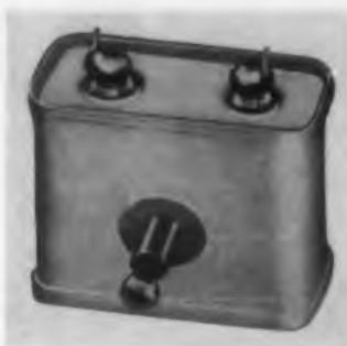
This series of polystyrene and "Teflon" dielectric capacitors may be adjusted to values from 1% below to 1% above nominal. Once set, the capacitance will remain constant indefinitely.
