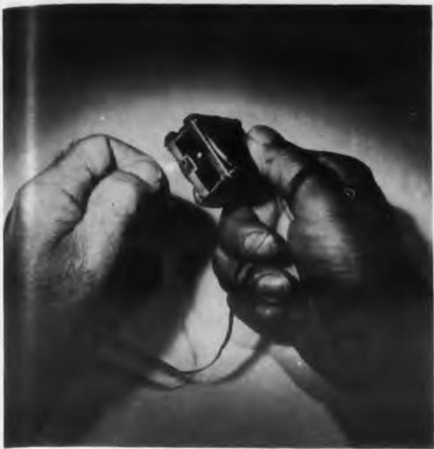
The inductance of this assembly is being adjusted by moving the ferrite-coated trimmer strip.
