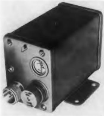
These time delay relays provide all the features of hermetically-sealed units and also permit adjustment of the time delay period. This feature is accomplished by coupling the standard adjustable type unit to a hermetic rotary seal. The timer is thus totally enclosed in
