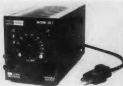
The Model DK-1 low distortion fixed-frequency power oscillator produces essentially pure, highly-stabilized sine wave power at 10v, 2w, and 0.03 ohm
