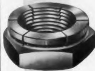
Regular FLEXLOCs are one-piece, all-metal, standard height nuts that lock securely, even under extreme vibration. Thin nuts have the same one-piece, all-metal construction and the same positive locking principle, but these nuts are approximately 30% thinner. Your FLEXLOC industrial distributor stocks both types: regular FLEXLOCs in sizes from #4 to 2"; thin FLEXLOCs in sizes from #6 to 1 1/2". Ask him for catalog information and samples. Or write STANDARD PRESSED STEEL Co., Jenkintown 12, Pa.
