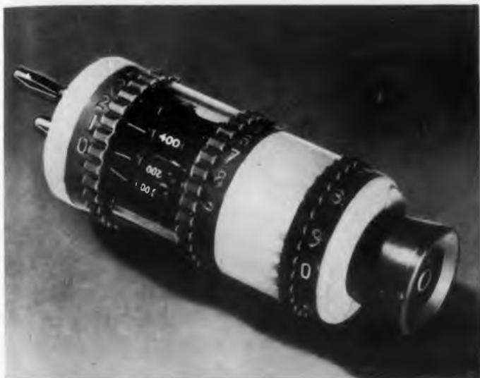
The compact Telex plug-in decade resistor is easily adjusted by its three control wheels.
