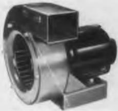
631 x 1—115 Volt, 60 cycle, 3450 RPM 100 CFM @ 2 1/2" water gauge. Fits in space 9 1/2" long, 8 3/4" wide, 7 3/4" high.
