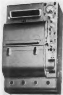
The 700C oscillograph for dynamic data recording is available in two models; one which records up to 36 channels on 8" wide recording media, and another which provides up to 60 channels using 12" wide paper. Record speeds as high as 114ips or as low as 0.030ips are made readily available through
