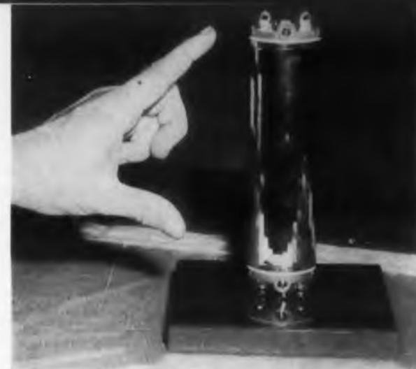
**Electrostatic Speaker . . .** Another phonograph incorporating an electrostatic speaker (*ED, September, 1954, p. 9*) has been placed on the market. Illustrated above, the speaker has a frequency reproduction range from 7000 to 20,000cy. It consists of 16 slender units arranged as facets on a half-cylinder. This arrangement radiates the sound uniformly throughout the room.
