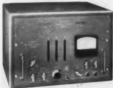
"Decimatic" Scalers are designed to measure all types of radioactivity precisely and easily. One of the main features of the design is the use of "modular" construction where-
