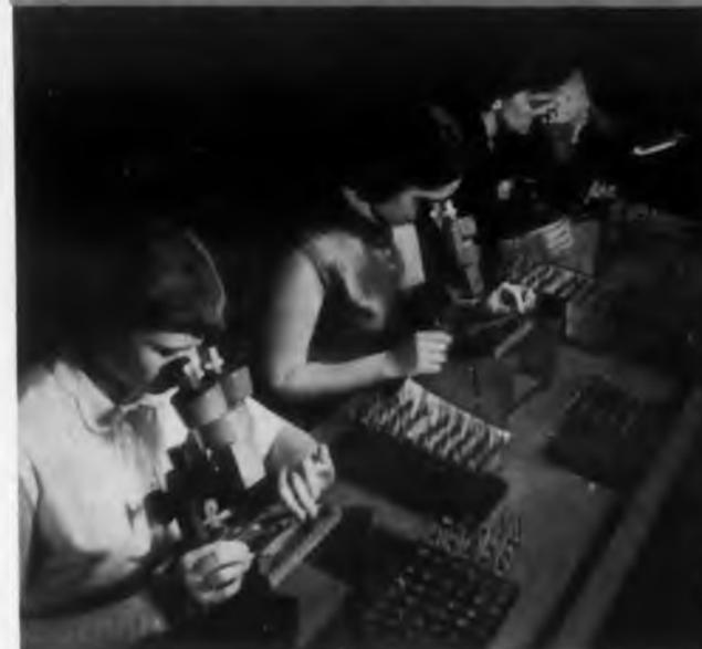
All these Raytheon Reliable Subminiature Tubes must pass microscopic inspection
