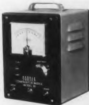
secondary standard for calibration of laboratory instruments.
