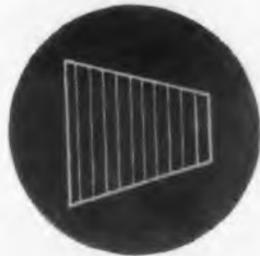
No sweep oscillator is necessary with this circuit to produce the modulation checking display shown above.
