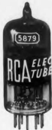
**RCA-5879**—is a sharp-cutoff pentode of the 9-pin miniature type intended for use as an audio amplifier in applications requiring reduced microphonics, leakage, noise, and hum. It is especially well-suited for input stages of medium-gain public address systems, home sound recorders, and general-purpose audio systems.
