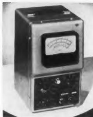
A series of electronic D-C Millivolt Meters have voltage ranges extending from 100 microvolts, for the most sensitive to 1kv for the highest range models. Input impedance on the low ranges is 6 megohms and 60 megohms on all ranges above 1v full scale. They contain an accurately tuned 120cy d-c, modulator which is driven from its own highly stable 60cy, R/C-tuned oscillator.
