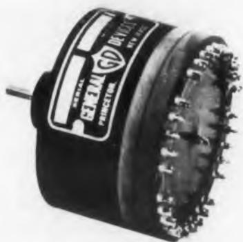
Typical specifications of this switch are 60 contacts, 30 channels, one pole, and sampling rates up to 60rps. Multiple stacked pole designs, as well as variations in the number and arrangement of con-
