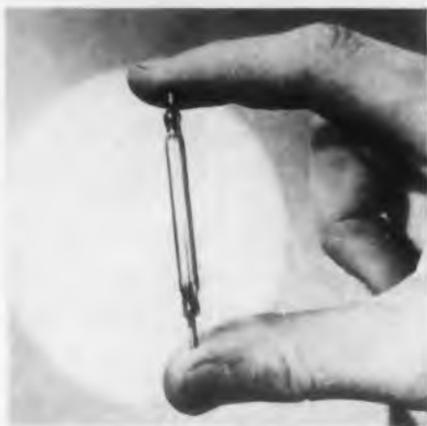
Contacts, which are closed when an external magnetic field is applied, are rhodium plated. They operate in an inert atmosphere hermetically sealed in a glass tube, permitting safe operation in explosive atmospheres. Contacts are rated at 0.5amp resistive or inductive at 28v d-c, or 10w 1amp load at 115v a-c. Revere Corp. of America, Dept. ED, 1000 N. Colony Rd., Wallingford, Conn.
