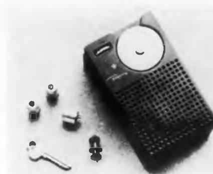
"Vo-Tron" sub-miniature if transformers and oscillator coils, originally designed for the new Regency all-transistor pocket-radio, are now in volume production by this firm.
