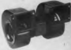
A15AD3—Axial blower unit for operation on 115 Volt 60 cycle single phase supply at 3300 RPM delivering 35 CFM at 0.2 S.P. This unit has special mounting bracket.
