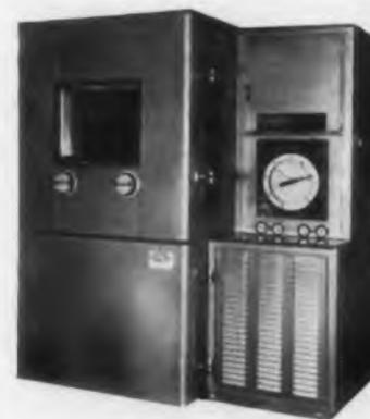
This climatic test chamber is for rapid, exact temperature tests, under varying conditions or cycles, of wire and cable. It is equipped with mandrils from 1/16" to 18" in size, with externally mounted turning devices and reduction gears for easy and exact control.
