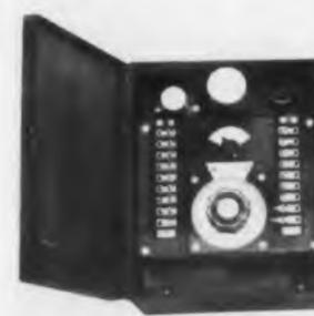
The Model T2, a precision general purpose electronic timer, is designed for interval timing, timed delay, repeat cycling, programming, or pulsing. Because of its special circuit design, the timer maintains 1% accuracy over line voltage variations of 90-135v. Thus, it is particularly suitable for industrial application where such variations may be present and would normally impair accurate timing.
