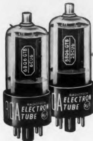
**NEW—RCA-6BQ6-GTB/6CU6, 12BQ6-GTB/12CU6, and 25BQ6-GTB/25CU6** are directly interchangeable with similar types in the 6BQ6 family. In comparison with previous versions, these types retain the same desirable characteristics, but feature a modified mount design to provide higher perveance and to permit higher ratings.
