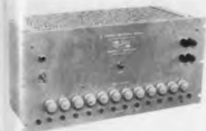
The Model 19 12-channel Electronic Switch provides a convenient, economical method for displaying 12 separate signals on a conventional single-gun cathode
