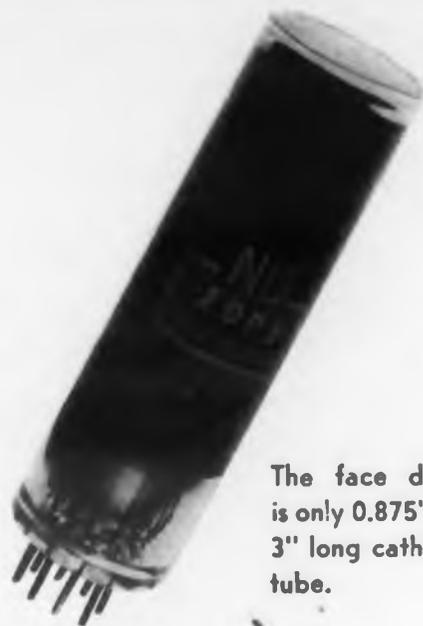
The face diameter is only 0.875" on this 3" long cathode-ray tube.
