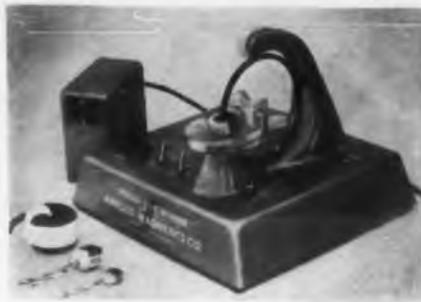
This simple toroidal coil winder is a useful device for the design laboratory. It handles AWG No. 26 to No. 44 wire. Minimum finished hole size is 0.18", with maximum OD of
