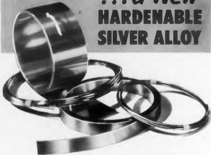
SILVER-MAG-NICKEL is its name. As you receive it, it is soft and ductile, like fine silver. Fabricate your most intricate parts, then oxidation harden them and this new alloy will hold its temper permanently. This hardness is not disturbed even when subsequent elevated temperatures are encountered.
