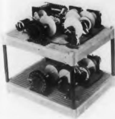
A rapid and economical method for designing, testing, and evaluating an infinite variety of experimental instrumentation setups is provided by the "grid plate" system and its associated "Erector Set" components. Light
