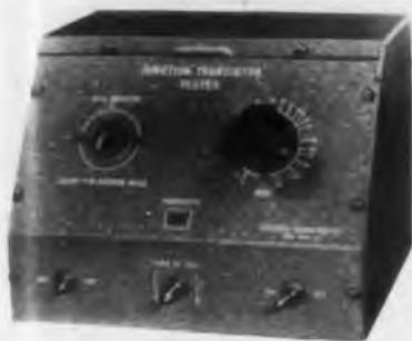
This low-cost tester provides a rapid, positive means of testing the current gain of any NPN or PNP junction transistor. A front panel selector switch allows rapid
