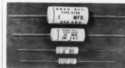
"Seramelite" capacitors are designed as reliable and economical units that have high humidity resistance and will operate continuously over a temperature range of  $-50^{\circ}$  to  $+100^{\circ}\text{C}$ . They are available with either paper or "Mylar" dielectric and are encased in ceramic tubes. They are sealed with a new thermosetting plastic.
