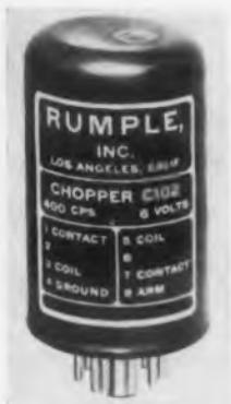
The C102 Precision Chopper has a temperature range of  $-85^{\circ}$  to  $+85^{\circ}\text{C}$ . It withstands 10g at 10-55cy, 30g of shock, and has a breakdown of 280v d-c. It is designed for 6.3v drive at 380-420cy. Contacts are spdt, rated at 0.002-amp, 100v. Dwell time is  $135^{\circ}$  ( $\pm 20^{\circ}$ ) and phase lag is  $65^{\circ}$  ( $+15^{\circ}$ ). Noise is less than 3mv peak-to-peak at 1 megohm.
