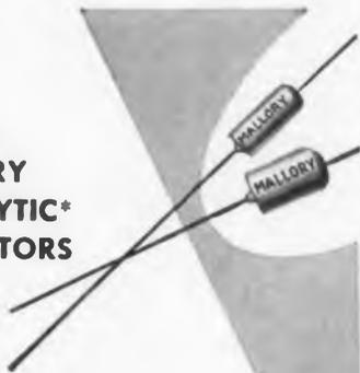
Capacitances up to 30 mfd. at 6 volts are compressed into sub-miniature case only  $\frac{7}{32}$ " in diameter by  $\frac{3}{8}$ " long, with temperature range from  $-55^{\circ}\text{C.}$  to  $+85^{\circ}\text{C.}$  Ultra-miniature Type TAW, rated 1 and 6 mfd. at 4 volts is only 0.145" in diameter by  $\frac{3}{8}$ " long.
