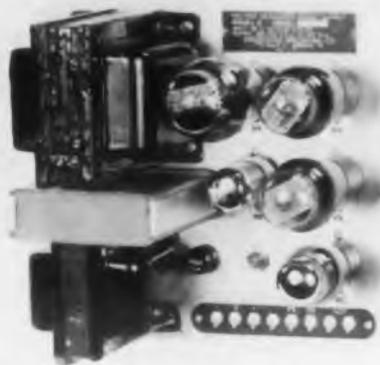
This sub-chassis mounting type regulated power supply can be mounted on a chassis along with other components to save space. The unit, known as Model 2, is an electronically regulated d-c power supply. Input is 105-125v a-c 50-60cy. Output is continuously variable from 200v to 325v d-c for load currents of 0 to 100ma. Regulation is better than 1%.
