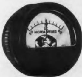
The Model 150 is a high precision 1-1/2" sealed panel meter designed for easy one-hole mounting without conventional mounting screws and related hardware. A Neoprene O-ring panel gasket provides a positive watertight juncture between the meter and panel. Terminal studs are similarly sealed. A knurled locknut with slots for wrench-tightening secures the instrument to the panel at the rear. Damage to the scale window will not destroy the watertight seal to the panel.
