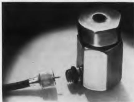
The Model 2101 Dynamic Force Gage has an extended frequency range and large output, permitting more thorough dynamic tests of servo systems, vibration-
