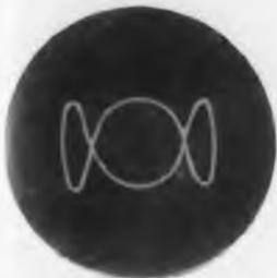
The frequency comparison circuit at the left requires no sweep oscillator. A typical display in which  $f_1/f_2 = 3/1$  is shown above.
