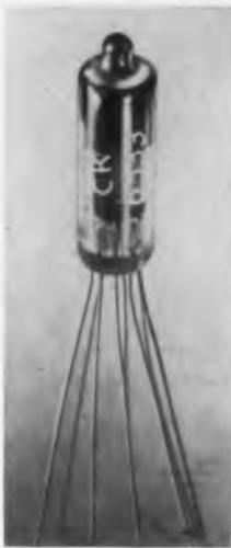
Type *CK6533* is an improved low noise subminiature triode with 6.3v, 200ma heater, amplification factor of 53, and mutual conductance of 1750 micromhos. At the standard test condition of 40 cy, 15g vibration, noise output across 10,000 ohms in the plate circuit is a maximum of 1mv, with typical tubes usually reading between 100-mv and 200mv.
