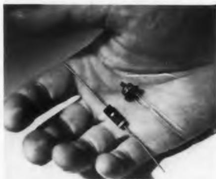
The 2N76 is a low-cost fused junction transistor having high reliability. It covers a broad specification range so that designers interested in developing and experimenting
