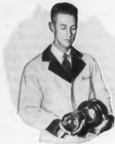
**New Compressor** (left) takes only 27% of the space of a conventional unit (right). It has only 10% as many parts, weighs 58% less, and will cost much less to produce.
