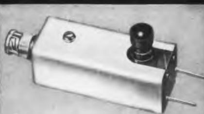
**RCA WG-298A UHF DEMODULATOR**—connects between the output of the WR-86A sweep generator and a 300-ohm termination for use in measuring the approximate standing-wave ratio of a 300-ohm-transmission line throughout the UHF range of 300-950 Mc. The WG-298A may also be used with other instruments such as the WR-40A, WR-41B or any UHF sweep generators using a 50-ohm BNC type output connector.
