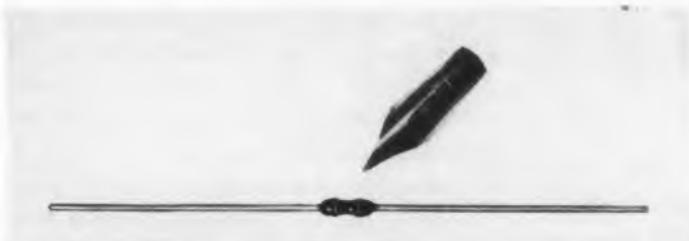
The Type C-5 miniature carbon deposited resistor is for transistor and hearing aid circuits. It has a diameter of 0.032", and is just 9/32" long. It is rated at 1/8w, with a minimum resistance of 5 ohms and a maximum resistance of 500,000 ohms.
