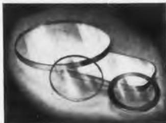
**METALLIZED GLASS INSTRUMENT WINDOWS** are made of both tempered and untempered glass with metallized bands on the edges. They can be easily soldered into a bezel to form a hermetic seal. Available in sizes and shapes to meet your needs.
