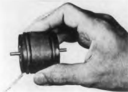
The motor presently is offered in 2-phase, 2-pole, 60cy units with ratings of 1w and 5w. Locked torque is 1.5oz-in and 5.5oz-in, respectively, and theoretical acceleration is 9650rad/sec<sup>2</sup> and 19,000rad/sec<sup>2</sup> respectively. Control phase is 50v and 115v, while reference phase is 115v for both units.
