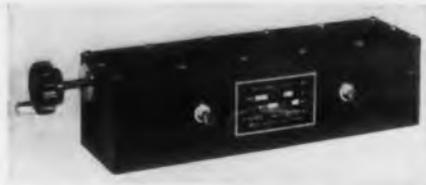
In this delay line, continuous variation of delay time is effected by rotary motion of a shaft. Variation
