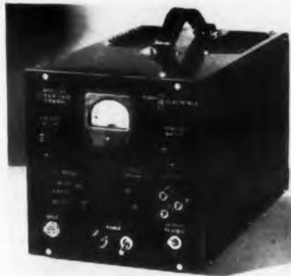
The Model 125 Strain-Gage Terminal is designed for use with this firm's Model 220 Wide-Band D-C Amplifier or other instruments with differential input. It contains a metered voltage source to energize
