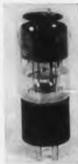
This single end thyratron, the NL-716, is rated at lamp d-c and 8amp peak current. It is designed especially for motor speed control and low current regulated voltage supplies.
