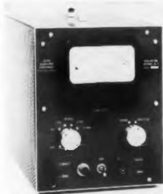
The Model D-1 "Reg-meter" provides direct measurement of power supply internal resistances without a complex laboratory setup. It measures from 0.02 ohms to 1,000 ohms in voltage sources with outputs ranging from 0 to 500v. The instrument may also be used as an accurate, stable a-c voltmeter
