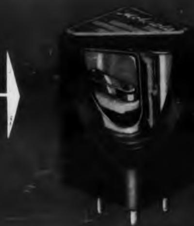
If your product requires a high degree of temperature stability . . . if compactness is a must—specify Stevens Type C\* thermostats. Since contacts open only when bimetal overcomes spring pressure and friction of bimetal against spring surface, electrically independent bimetal responds only to heat from controlled device—for a clean, positive break.
