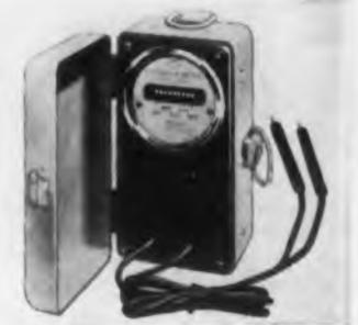
Insulated test probes are provided for shunting a portion of the voltage in the tested line across the 10,000-ohm internal resistance of the meter. An electromagnetic coil-armature combination applies mechanical energy at the frequency to be measured to the entire row of reeds. Only the reed having a natural frequency corresponding to line frequency will undergo vibrational response.
