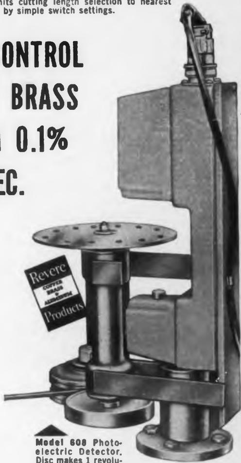
Model 608 Photoelectric Detector. Disc makes 1 revolution per foot of tube travel. 12 holes provide counting in inches. Resolution of measurement can be increased if desired.
