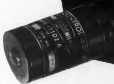
Servomechanisms, Inc. Type 17ID, for use with the amplifier, is a damped-control motor whose control winding is the output load for the amplifier.
