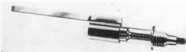
The Model VC-13G variable trimmer piston capacitor employs an expansion piston with a traverse motion, free from mechanical backlash, giving smooth capacitance tracking over the complete range. There is a rigid grip at all times between the piston and inner wall of the dielectric tube. Consequently, the capacitor is relatively free from effects of vibration and shock. The positive wipe, due to the constant spring tension of the moving parts, assures good r-f contact and low noise ratio.
