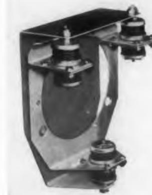
This mounting system, Model 1102, incorporates three all-metal double-acting mounting units. Located in the vertical plane of the center-of-gravity of the instrument, the mounting units combine to give a natural frequency of approximately 15cy. Effectively isolating vibration and shock forces, the system provides multi-directional protection to instruments installed on bulkheads or airframe structures. It meets requirements of MIL-E-5272B, Procedure 1.
