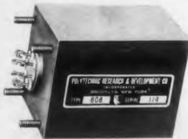
The PRD Type 808 is a phase sensitive demodulator producing a full wave, reversible polarity, d-c voltage output from a reversible phase, a-c voltage input. It will also
