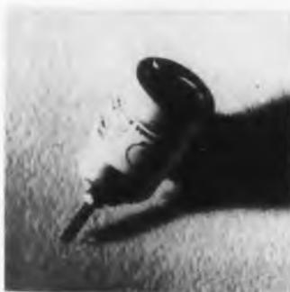
Available both shielded and unshielded, Style A Type 1 Variable Inductors are supplied in 10 standard values from 56μh to 1.8mh, and up to a maximum of 25mh in special units. They feature an inductance variation range of 2:1; Q's of approxi-
