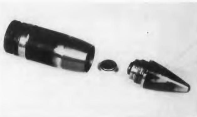
Only 1" long, this plastic encapsulated transmitter has an even smaller mercury battery beside it. The transmitter and 200hr cell fit into the nose of the illustrated projectile.
