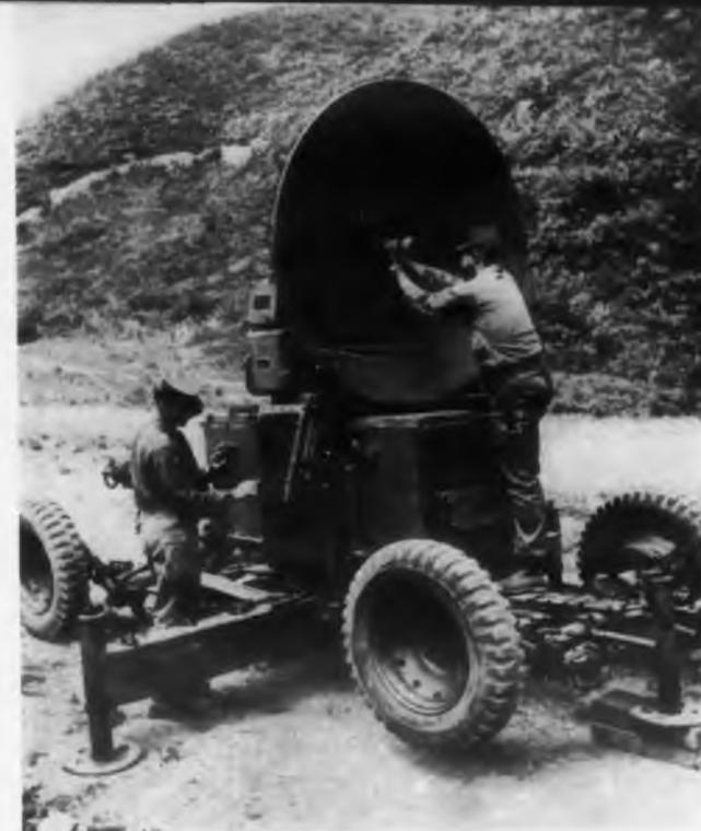
**Mortar-Detecting Radar . . .** The development of a mortar-detecting radar, already battle proven during the Korean war, has been announced by the U. S. Army. Within a short time after an enemy mortar commences firing, the detector system relays its position to an artillery fire direction center. Artillery fire is then pin-pointed on the mortar.
