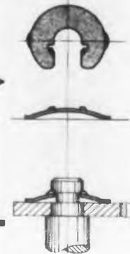
The "Series 5139" is a radially-applied retaining ring which can be locked positively in its groove and used as a shoulder against rotating parts, replacing expensive nuts and bolts and eliminating the need for springs, washers, and other accessory fastening devices. It is made of spring steel and is shaped like a bowed horseshoe. When fastened to a shaft, it is locked in its groove by two prongs extending from the inner circumference of the open end (illustrated at the top).
