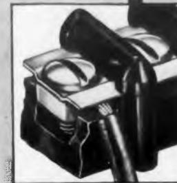
Without a doubt, the simplest space, labor and cost saving Terminal Block made. Stripped wire is inserted between clamping members without looping or other preparation and the screw tightened — it's there to stay unless the wire itself breaks. Screws nest in blind holes in the solid molded base, eliminating danger of shorting. The type "E" is factory produced in any number of terminals from 1 to 22.
