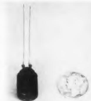
The cell is available with a flat glass or small collecting lens. The spectral response peaks in the visible range at about 0.5 microns, and falls off rapidly in both the infrared and ultraviolet ranges. Selected units can be applied directly to the 110v a-c line. Maximum internal power dissipation is about 50mw.
