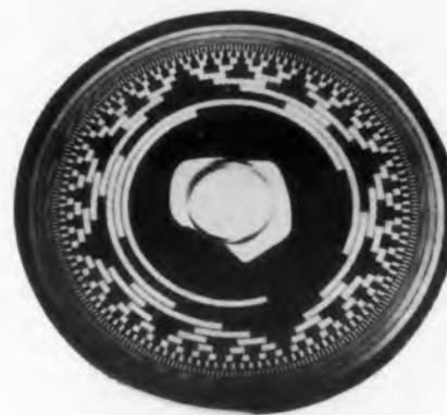
A Gurley Code Wheel. Base material is polished glass for use with photoelectric as well as magnetic or contact pick-ups.
