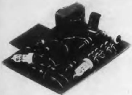
Fig. 2. Transistorized amplifier mounted on phenolic printed circuit board.
