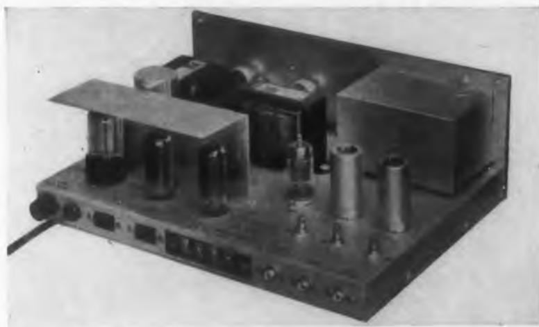
The Harman-Kardon "C-100 Melody" ("3-1/4" high x 12-1/2" wide x 7-1/4" deep) matches this firm's "Theme" am-fm tuner. Most of the wiring of the amplifier is exposed for easy repair by removing a few screws. The tubes are hidden by the grate.
