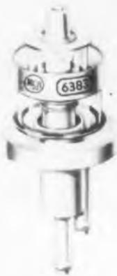
The 6383 is a compact, liquid- and-forced-air-cooled u-h-f power triode. It is designed primarily for applications where transmitter design factors of compactness, light-weight, and high power output are prime considerations. It has a maximum plate dissipation of 600w and can be operated with full plate voltage and plate input at frequencies up to 2000Mc.
