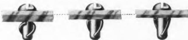
Spring-Lock works whether panel thicknesses run over or under specifications! Spring wire deflects automatically to handle greater or lesser thicknesses. Spring-Lock's design flexibility makes it more than a fastener: it can be adapted as a shelf support, door strike, knob or any similar panel-mounted device. Many standard shapes and sizes of Simmons Spring-Locks are available from stock.
