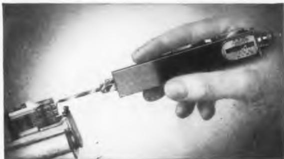
**For GO/NO-GO Tests of Springs and Contact Pressures**
