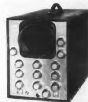
The high deflection sensitivity of 35mv, rms, per inch, from 10cy to 5Mc on both amplifiers, is another feature. This general purpose, high-gain instrument is particularly designed for color TV measurements. Crosby Laboratories, Inc., Dept. ED, Box 233, Hicksville, L. I., N. Y.
