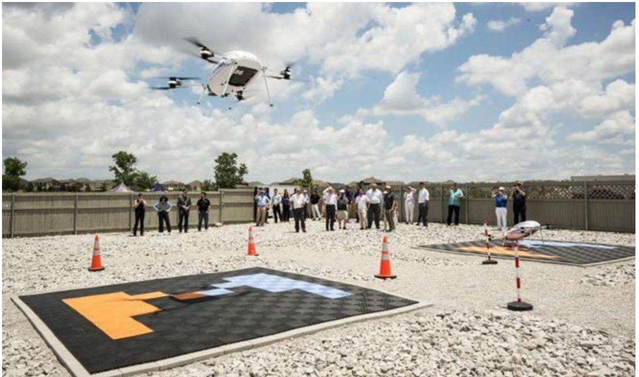
NASA gathered members of the FAA and commercial drone engineers in Dallas to show off multiple delivery drones that will operate in a shared airspace beyond the visual line of sight (LOS), using an industry-developed, NASA-originated, uncrewed aircraft system traffic management system. (Image courtesy of NASA)
