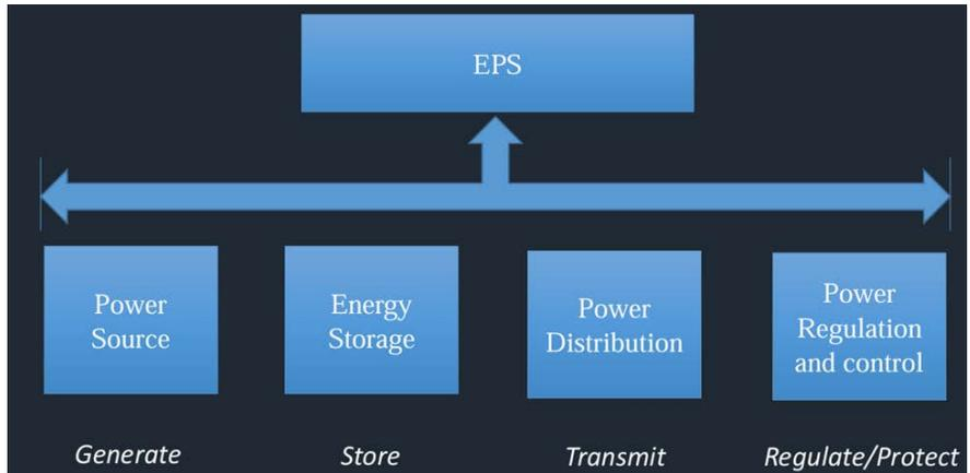
1. A typical electrical power subsystem (EPS) in space. (Image courtesy of NASA)
