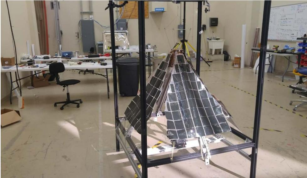
5. The LISA-T Tiny Solar Array delivers a significant amount of power in space. (Image courtesy of NASA Marshall Space Flight Center)
