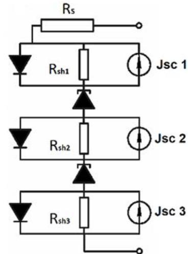
4. The illustration demonstrates the equivalent structure of “InGaP/GaAs/Ge” triple-junction solar cells and electrical equivalent structure (left). The electrical equivalent circuit model of these triple-junction solar cells is shown on the right. The power provided via these cells is decided on via the I-V curve and the external resistance of the load, using the [theory of conventional circuitry](#). (Image courtesy of Reference 4)
