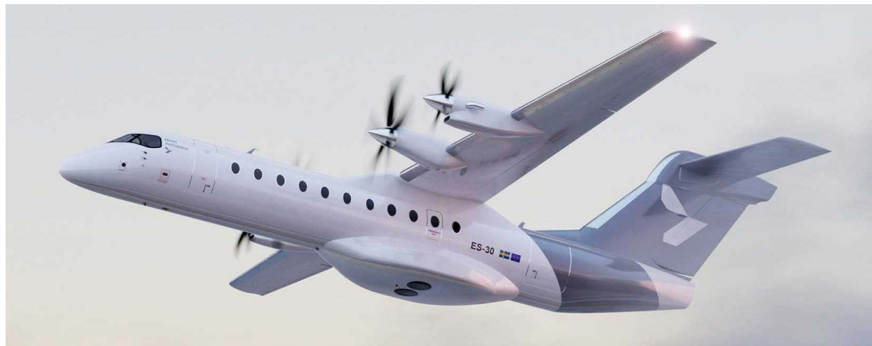
5. Capable of carrying up to 30 passengers up to 200 km in its all-electric mode and up to 800 km with its turboprop range extenders, a prototype of Heart Aerospace's ES-30 will enter testing this year with production anticipated to commence before 2030. (Credit Heart Aerospace)
