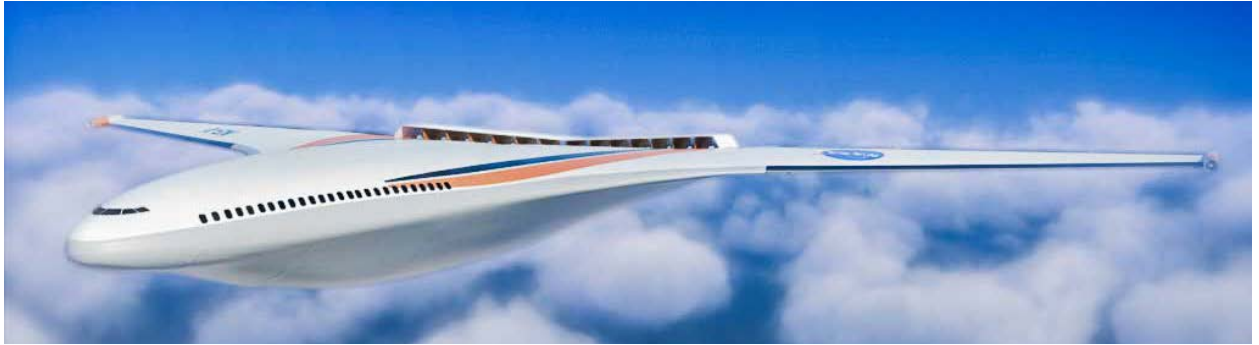
6. Designed to operate with the same range, speed, and airport infrastructure of today's large twin-aisle aircraft, the N3-X would require 70% less fuel per passenger-mile than today's most efficient wide-body jets. (Credit NASA)
