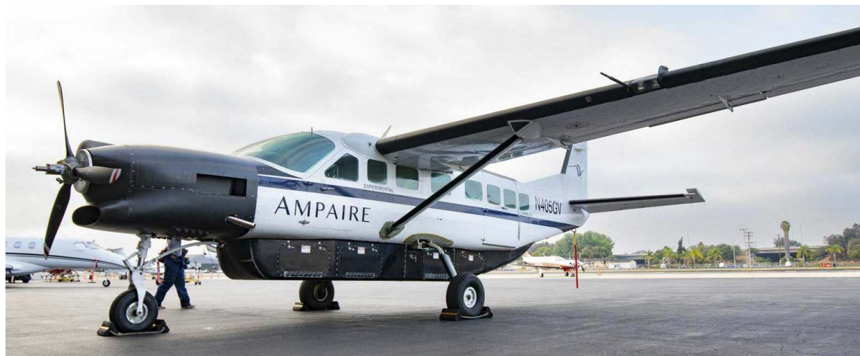
4. The Eco Caravan, equipped with Ampaire's AMP-H570 plug-in hybrid-electric powertrain, is now flying and available for pre-order. The nine-seater aircraft is powered by both a combustion engine and an electric propulsion system with energy supplied by a battery pack located in the cargo pod. (Credit: Ampaire)
