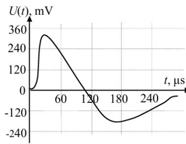
6. This is the result of physical modeling of EMI in the communication line of a real CE inside a building.
