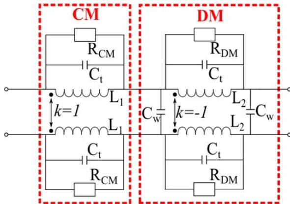
8. It's preferable to use a more precise circuit with separate common and differential blocks to show that the CMC7 behaves differently in common and differential mode. (Image courtesy of Reference 2)
