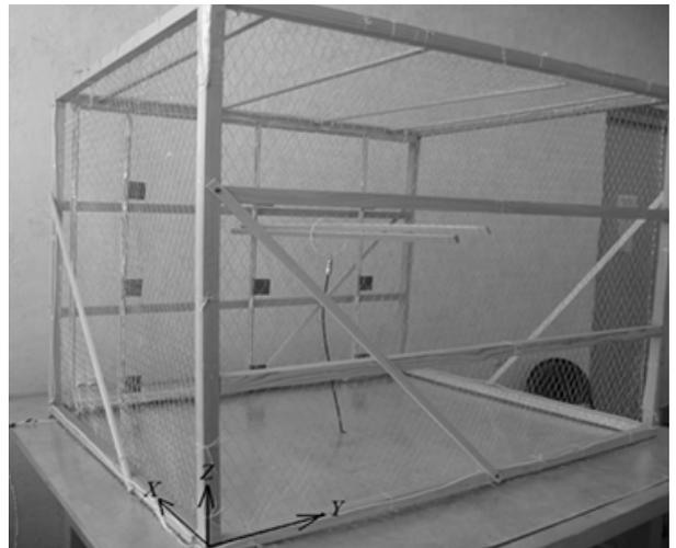
1. Shown is a scale model of a building that has walls with a reinforcing mesh and reinforced concrete. (Image courtesy of Reference 1)
