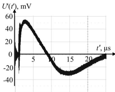
5. The measured EMI in the communication line of a scale model building at the measuring point closest to the connection point of the intentional current generator.
