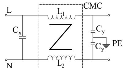
7. This image is a schematic illustration of a one-stage EMI filter (Image courtesy of Reference 2)
