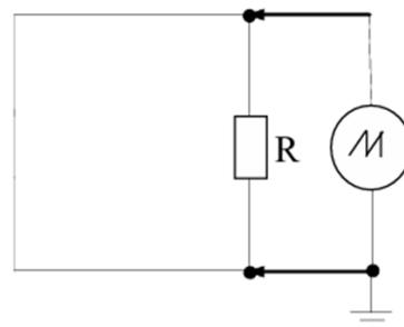
2. This is an interference measurement circuit. (Image courtesy of Reference 1)
