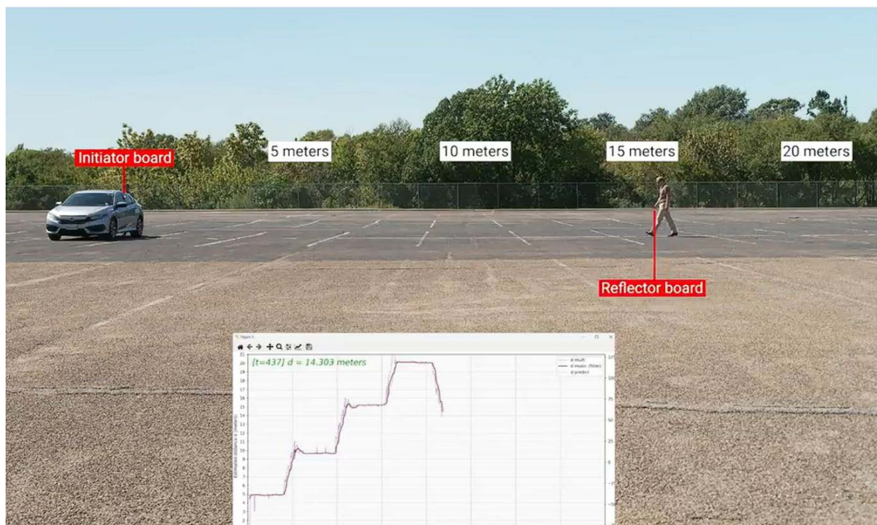
3. A channel-sounding demonstration plots distance (inset) between an initiator and reflector with minimal latency. (Credit: TI)
