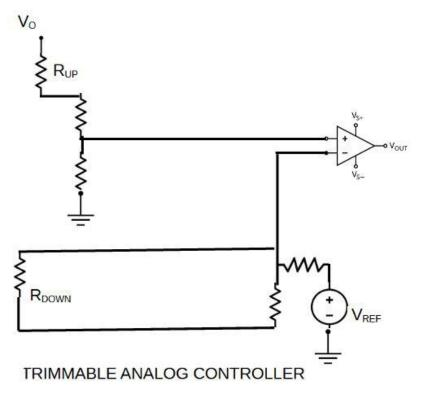
This controller uses two external resistors, RDOWN and RUP, to adjust the output voltage. RDOWN lowers the output voltage by reducing the signal to the error amplifier's positive input. RUP raises the output voltage by reducing the signal to the error amplifier's negative input. (Credit: Alan Earls)
