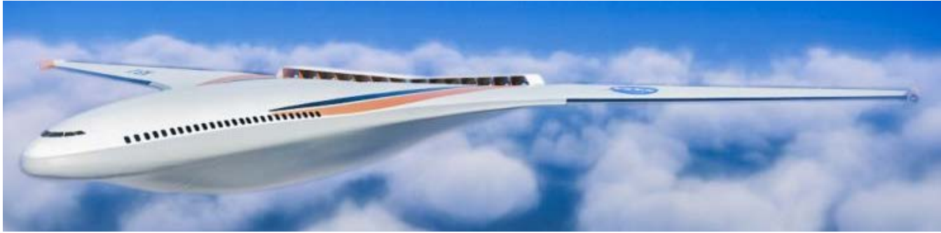
10. This is an artist rendering of the N3-X concept aircraft with hybrid wing body airframe. Credits: NASA
