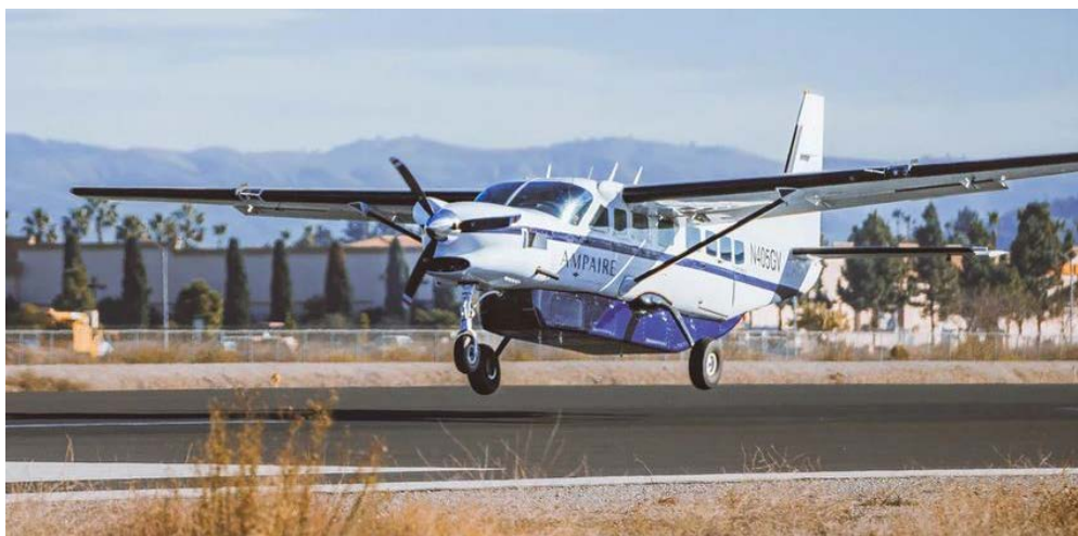
6. Both Ampaire and Textron are developing variants of Cessna's popular Caravan utility aircraft that replace the airframe's turbine power plant with a hybrid-series powertrain. Credit Ampaire and Textron
