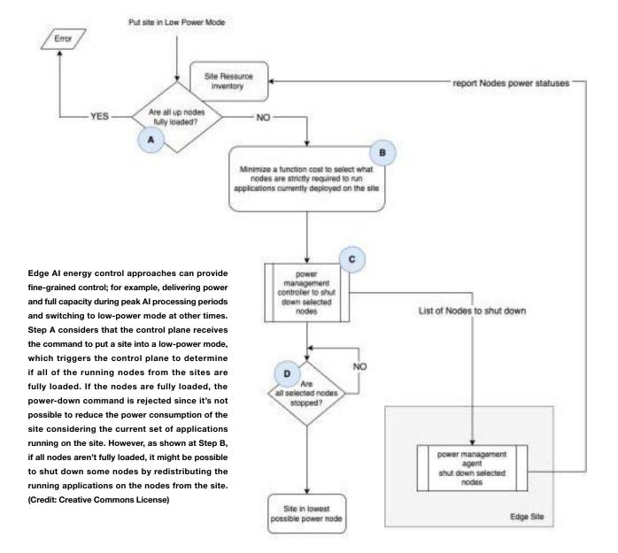
periods of operation based on the specific use case. They also outline various schema for logically controlling such situations (*Fig. 1*) "by determining an optimal compromise between application availability and edge site power consumption without the use of specialized/bespoke hardware at edge sites."
