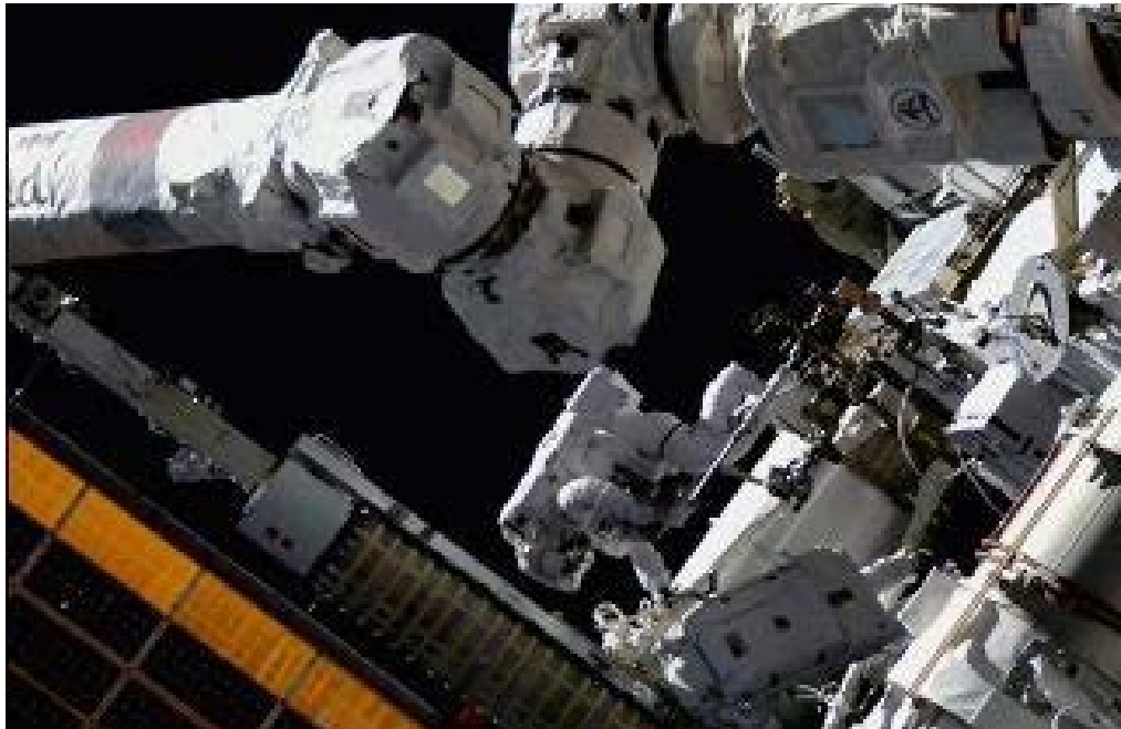
2. NASA astronaut Warren “Woody” Hoburg (who can be seen in the center, partially obscured, with red stripes on the astronaut’s space suit legs) is holding on to an ISS Roll-Out Solar Array (iROSA) as he grasps the end of the ISS Canadarm2 robotic arm. Also shown is Stephen Bowen, an Expedition 69 crewmate, preparing the solar array’s mounting bracket at the bottom of this image during the spacewalk on Thursday, June 15, 2023. (Image credit: NASA TV)
