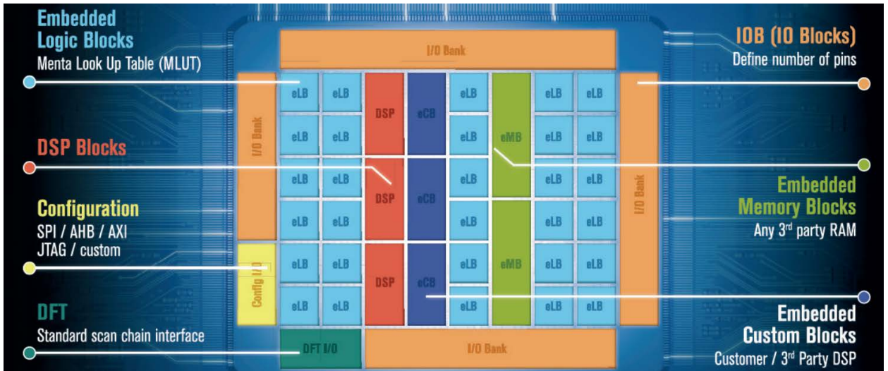
1. Menta's eFPGA consists of smaller elements, with the I/Os and components that make up the Matrix.
