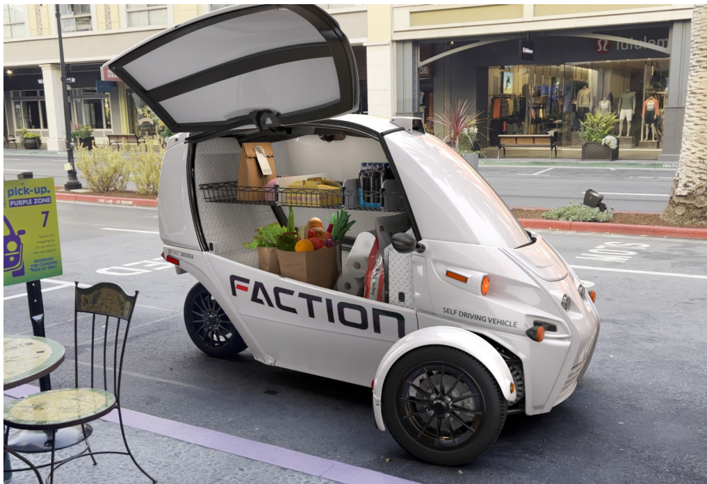
5. Faktion relies on RTK to help its self-driving delivery vehicles achieve centimeter-level precision.
