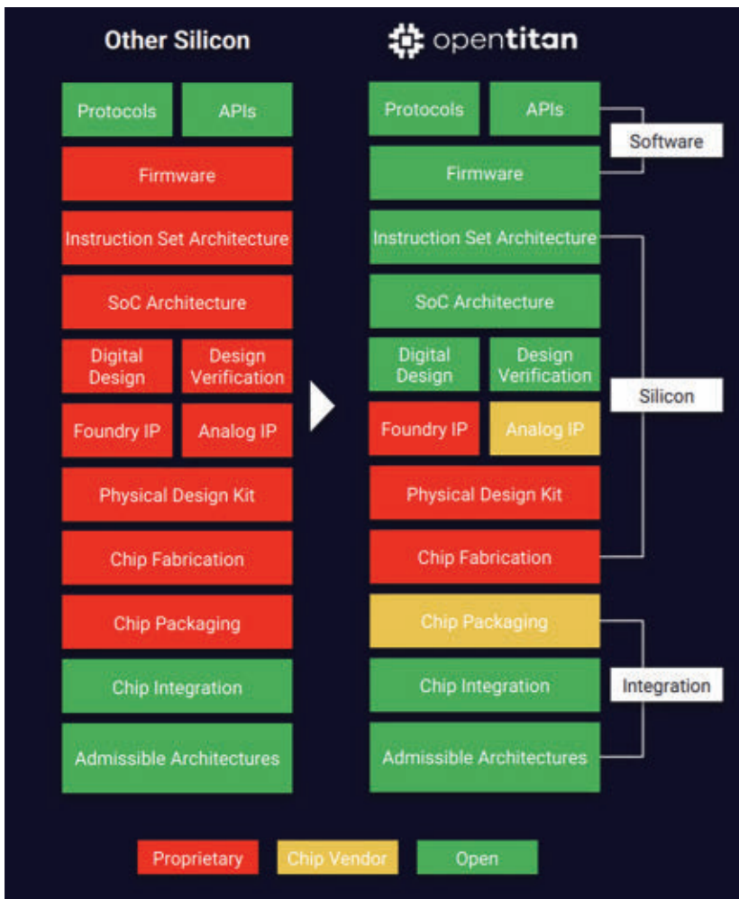
The core differences between open and closed approaches to chip design. zeroRISC
