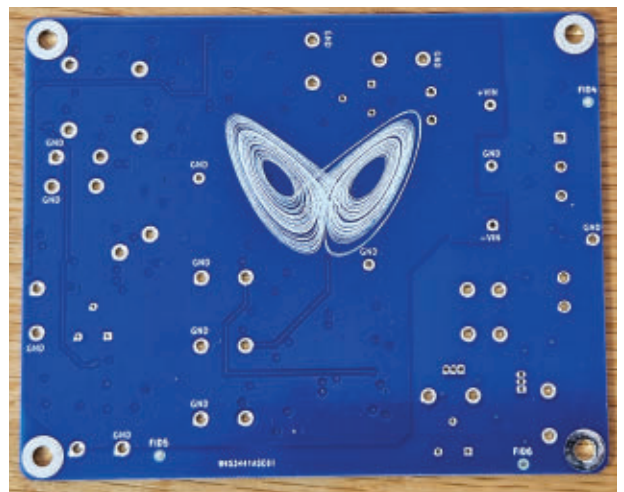
2. Bottom view: Chaotic Circuits PCB.
