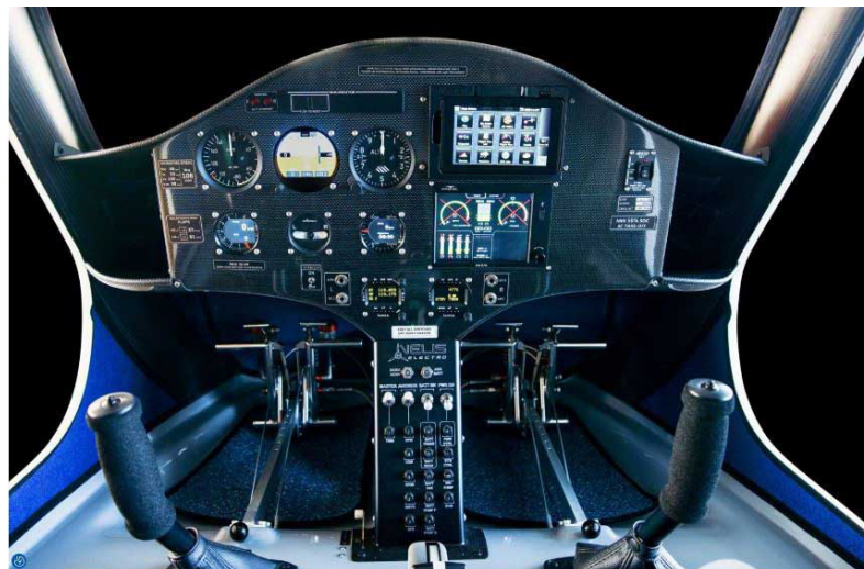
3. The Pipistrel Velis is a two-place all-electric aircraft, intended primarily for aviation training. With a cost that's comparable to other trainer aircraft and able to fly for roughly an hour on a charge, the Velis costs a small fraction of a conventional aircraft to operate. As a result, it's becoming increasingly popular with flight schools in Europe and elsewhere. (Pipistrel)
