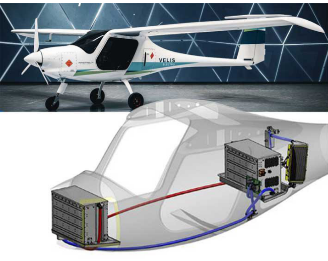
3. The Pipistrel Velis is a two-place all-electric aircraft, intended primarily for aviation training. With a cost that's comparable to other trainer aircraft and able to fly for roughly an hour on a charge, the Velis costs a small fraction of a conventional aircraft to operate. As a result, it's becoming increasingly popular with flight schools in Europe and elsewhere. (Pipistrel)
