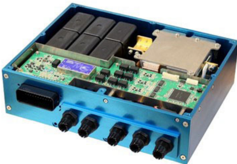
5. Shown is GaN Systems' (now part of Infineon) automotive traction inverter. (Image courtesy of Infineon)
