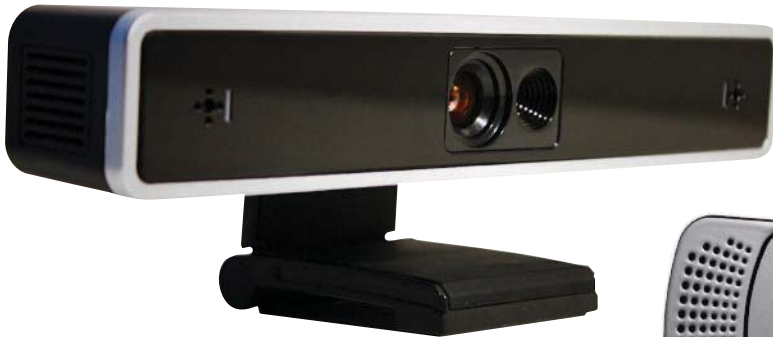
2. The SoftKinetic module allows developers to easily incorporate 3D sensing in embedded applications.
