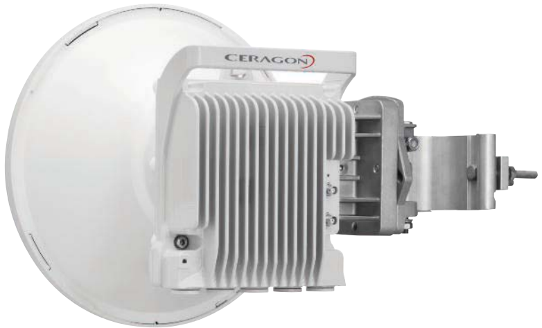
5. The Ceragon FibeAir IP-20C is typical of the small-cell backhaul units available. It is available in standard licensed band frequencies from 6 to 42 GHz. Typical data rate is 1 Gbit/s in a single channel. It uses 2048 quadrature amplitude modulation (QAM) and can implement 4x4 MIMO in line-of-sight situations.
