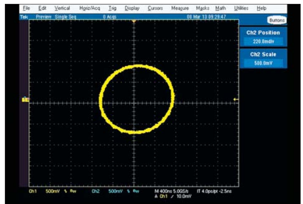
6. The Lissajous curve for the circuit using the MSVHFS6 3.3-V filters shows the outputs' phase relationship.
