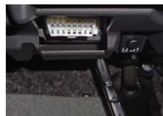
Audiovox's Car Connection dongle (a) plugs into a socket found under the dash (b).
