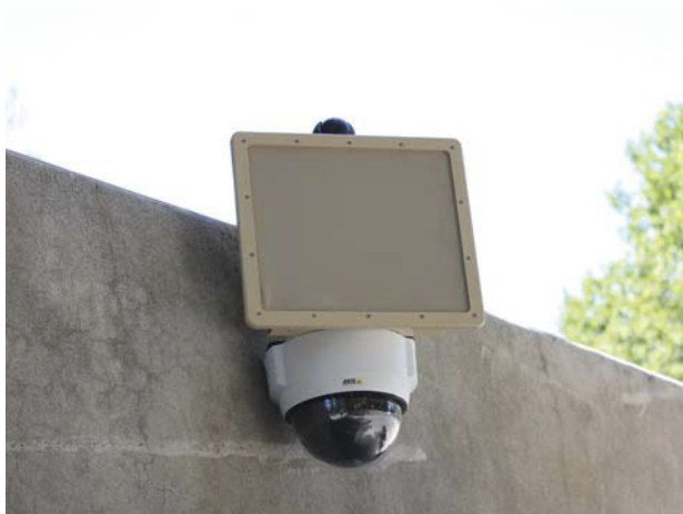
2. A key part of the Radar Backpack Kit is the SpotterRF M600C radar unit which includes an Ethernet port for ease of connection to a portable computer.
