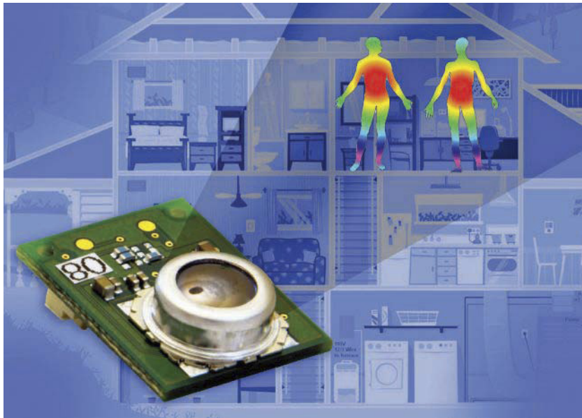
6. Omron's non-contact D6T MEMS sensor offers high noise immunity. It is more reliable than conventional pyroelectric, IR, and passive IR sensors used in industrial, building, and home automation applications.
