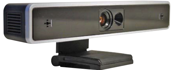
1. SoftKinetic's DS311 can handle hand and finger recognition at a range of 0.15 to 1 m. It can also manage body recognition from 1.5 to 4.5 m using a brighter IR emitter setting.
