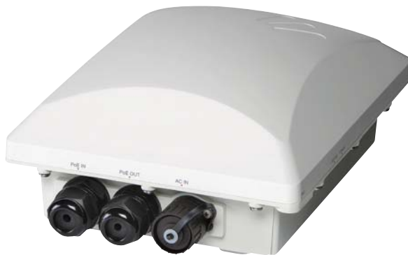
3. The Ruckus Wireless 7782 outdoor carrier-grade access point uses 30° and 120° antenna patterns to improve link reliability, capacity, and speed.
