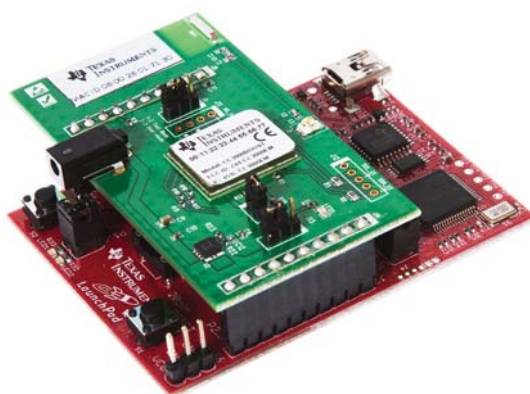
2. The Texas Instruments SimpleLink Wi-Fi CC3000 Booster-Pack development board and MSP430 LaunchPad evaluation kit speed the creation of Wi-Fi based IoT applications.
