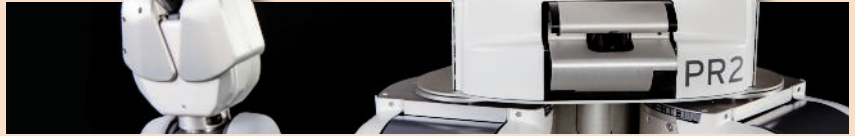
The PR2 from Willow Garage includes a variety of stereo cameras in its movable head and hides a Hokuyo UTM-30LX laser scanner in the neck. Microsoft Kinects have been seen to sprout from the top of the head.
