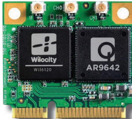
2. Incorporating the 802.11n chip from Qualcomm Atheros and the 60-GHz chip from Wilocity, this three-band module suits hot spots, routers, and other WLAN products.
