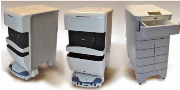
2. Hundreds of Aethon TUGs are being deployed in hospitals to deliver everything from medicine to meals.
