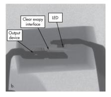
3. Optocouplers incorporate light emitting diodes, phototransistors, and an insulating dielectric film between these elements.
