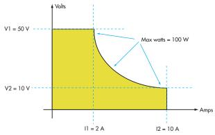
2. In this output characteristic of an autoranging power supply, VI represents the maximum voltage and II represents the corresponding current such that II = max watts/V1. I2 represents the maximum current, and V2 represents the corresponding voltage such that V2 = max watts/I2. Along the curved portion, the available voltage and current is limited by max watts. The characteristic shown is for a 50-V, 10-A, 100-W 5:1 autoranging power supply.
