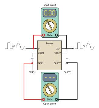
1. An ideal isolator offers an open current path for the signal while also appearing to be a short circuit.
