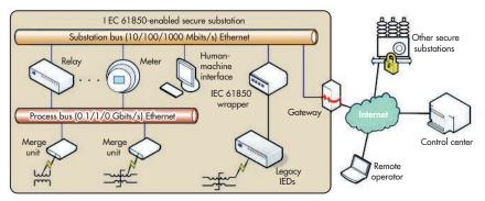
2. IEC 61850 envisions a substation network connected to the outside wide area network via a secure gateway. Outside remote operators and control centers can use the abstract communication service interface (ACSI) to query and control IEDs in the substation. One or more substation buses connect all the IEDs inside a substation.
