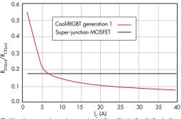
3. IGBTs like those made on International Rectifier's Cooll2R platform offer reduced conduction losses and greater efficiency at higher currents than MOSFETs. (courtesy of "IGBTs or MOSFETs: Choose Wisely" by Carl Blake and Chris Bull, International Rectifier)
