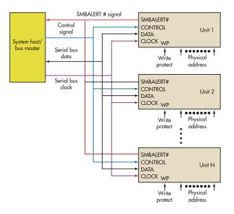
1. Electrically, PMBus is  $I^2C$  with an added "alert" signal back to the controller.
