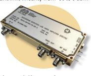
log-video output rise time and 40-ns maximum output settling time. The amplifier provides a limited intermediate-frequency (IF) output of typically +5 dBm and has an output video log slope of nominally 40 mV/dB. Propagation delays are typically only 7 ns. The compact SDLVA measures  $3.75 \times 1.50 \times 0.50$  in. It draws 200 mA current from supplies of +12 to +15 VDC and 190 mA current from negative supplies of -12 to -15 VDC.
