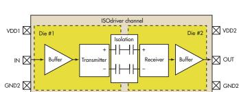
4. Modern CMOS isolation devices incorporate SiO<sub>2</sub>-based capacitors.
