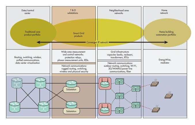
I. Cisco sees design opportunities across many network levels using IP. Note that there isn't necessarily any utilization of the tactically vulnerable conventional Internet in the critical functions at the left side of the diagram.
