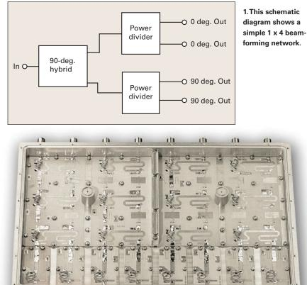
2. This is a commercial 8 x 8 beamforming network designed to operate within two frequency bands from 1025 to 1095 MHz. [Photo courtesy of TRM Microwave (www. trmmicrowave.com).]
