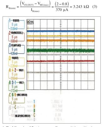
3. The falling edge of  $Q_A$  triggers an oscilloscope, which uses  $V_{RB1}$  (trace A) and  $V_{RC1}$  (trace B) to calculate  $h_{FE}$  (trace D).
