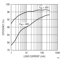
Figure 2. Efficiency of Circuit in Figure 1
