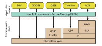
3. The IEC standard defines a communication structure with four communication profiles: ACSI, the generic object-oriented substation event (GOOSE), the generic substation status event (GSSE), and the sampled measured value multicast profile (SMV).
