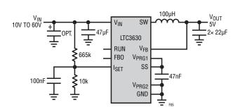
Figure 5. 5V Regulator with 55mA Input Current Limit
