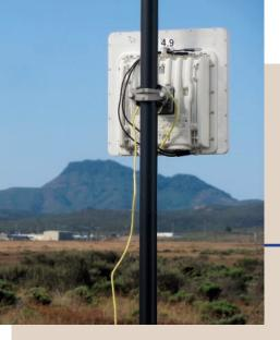
icrowave backhaul systems such as the PTP 600 series of wireless Ethernet bridges from Cambium Networks Ltd. (www.cambiumnetworks.com) are invaluable for both licensed and unlicensed links. Designed for licensed use in the 2.5-, 4.5-, and 4.9-GHz bands (with license holders such as NATO) and unlicensed use support data rates to 300 Mb/s at dis- communications. tances to 124 miles.
