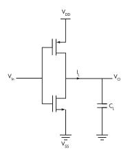
In a basic CMOS inverter, power is dissipated across a PMOS transistor when the load capacitor is being charged and across an NMOS when the load capacitor is being discharged.
