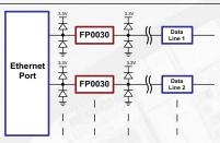
The Supertex FP0030 is a 20V current limiting protection device. It is designed to protect Internet devices from high transient voltages.
