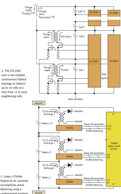
flyback dc-dc converter accomplishes active balancing using a unidirectional topology.
