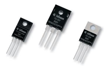
2. The Infineon Technologies 650-V TrenchStop 5 process reduces switching losses by more than 60% compared to current leading solutions. Thin wafers provide what Infineon calls best-in-class IGBT device performance. The devices come in TO-220, TO-220 FullPak, and TO-227 packages.
