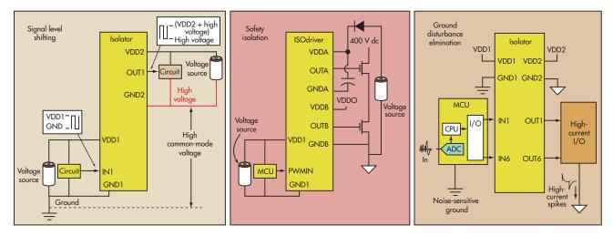
2. Isolation tasks include safety isolation, level shifting, and eliminating ground noise.
