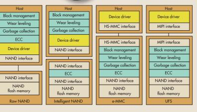
NAND flash requires a number of features for reliable operation, including error correction and provide all services usu- wear leveling. These services can be performed by the host or offloaded to the memory using ally within the device standard interfaces like e-MMC and UFS.
