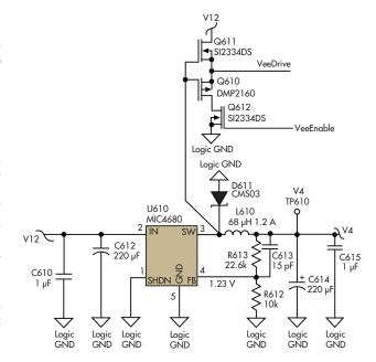
1. The 12-V downswitcher, which is already in the design, provides a square-wave to generate VeeDrive from V12 with about a 10-V swing.
