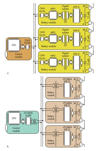
I. Contemporary production vehicles with modular battery packs have used a combination of CAN communications and digital isolators to interface the modules (a). In Linear Technology's alternative approach, multiple ICs are connected using the company's proprietary two-wire isoSPI interface, using the LTC6820 isoSPI transceiver and a simple Ethernet transformer (b).
