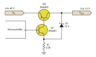
The microcontroller turns the load off by controlling a high-side switch formed by Q1 and Q2. The current-sink action of Q1 controls the load voltage.
