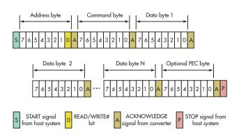
2. The standard master-to-slave communication sequence comprises multiple data packets.
