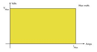
I. A rectangular output power supply can operate anywhere within the limits of  $V_{Max}$  and  $I_{Max}$ , but achieves max watts only at V =  $V_{Max}$  and I =  $I_{Max}$ .
