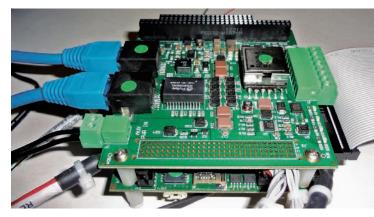
2. The WinSystems PPM-PS394 PoE node can power a PC/104-Plus stack.
