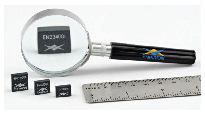
5. Enpirion's EN2300 4- to 15-A buck converter module includes a controller, inductor, filter capacitors, and MOSFETs, all in a single QFN package.
