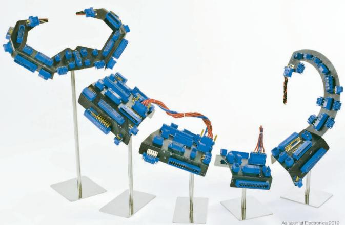
Scorpion by Positronic provides the ultimate flexibility in configuring your power/signal connector layout of choice. Every connector shown in this sculpture was made from the same set of tools using modular inserts. Insert options exists for size 8 high power contacts up to 80 amps continuous. Other inserts include size 12, 16, 18 and 22 for power and/or signal use. Visit www.connectpositronic.com/scorpion for more details.
