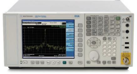
Signal analyzers in the N9010A EXA series offer tremendous capability and numerous options, with the broadest-frequency model spanning 10 Hz to 44 GHz. [Photo courtesy of Agilent Technologies (www.agilent.com).]
