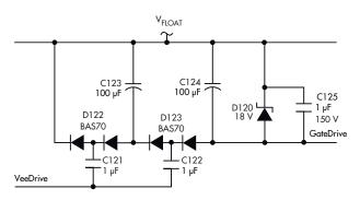
2. The charge pump generates a robust supply that always tracks 15 V below V<sub>FLOAT</sub>, even if that voltage is below ground. The voltage also can be placed above V<sub>FLOAT</sub> by simply reversing the diodes and the polarized capacitors.
