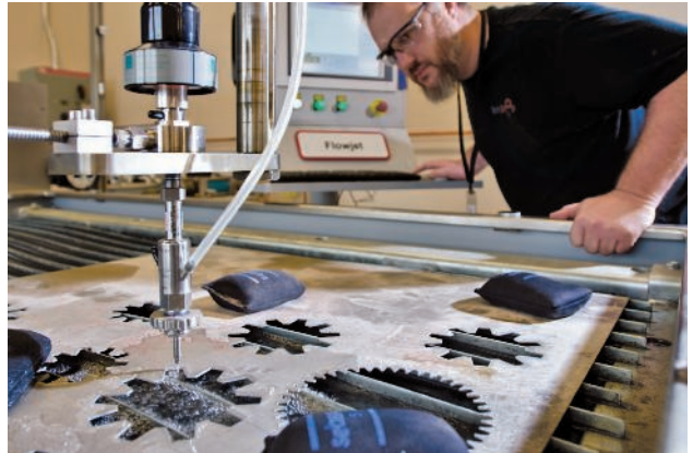
3. TechShops members have access to a wide range of tools in electronics labs as well as metal and wood shops. Lead dream consultant Shawn Simone is using the DETflowjet water jet, which can cut precisely through 6 inches of almost any material.
