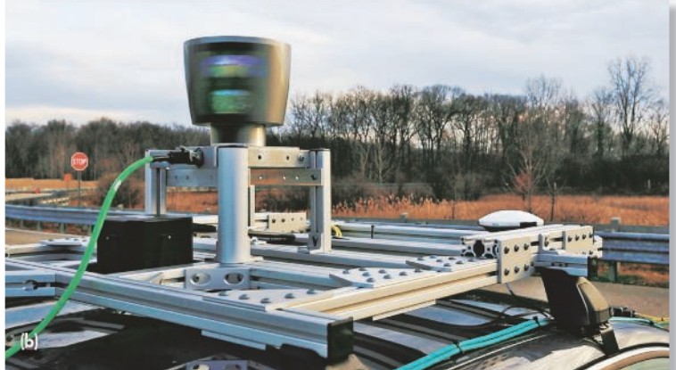
Toyota showed off its self-driving Lexus LS600 research vehicle (a) at the C2013 International CES in Las Vegas. It uses a 360° laser tracking system on the roof (b).
