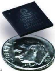
5. The Greenview GV7011 Hybrii-XL integrates a full ZigBee radio and a HomePlug Green PHY transceiver including the full analog front end, RF, baseband, media access controller (MAC), and embedded memory. An 8051 microcontroller implements low-power energy management.
