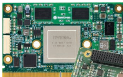
6. Kontron's ULP-COM-sAT30 runs a 1.2-GHz NVidia Tegra 3.
