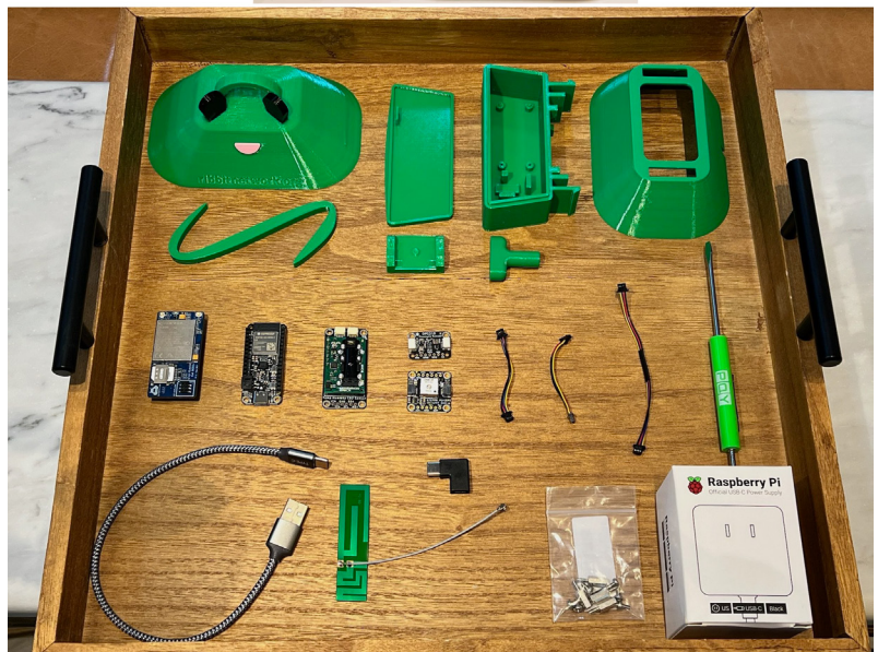
The open-source Frog Sensor (top) from Ribbit Network is built around a Raspberry Pi CM4 module. (Ribbit Network)
