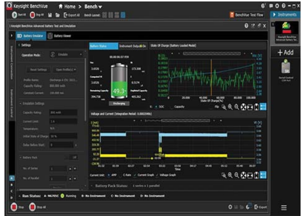
3. BV9210B/11B software is used for battery emulation.
