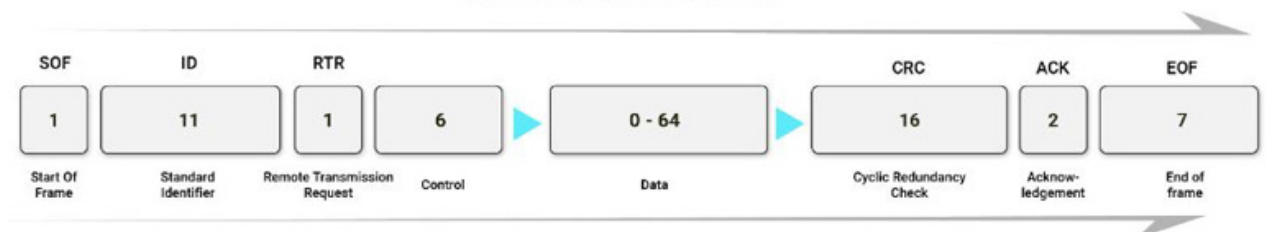
3. Shown is the CAN Bus packet structure. (Credit: AutoPi)
