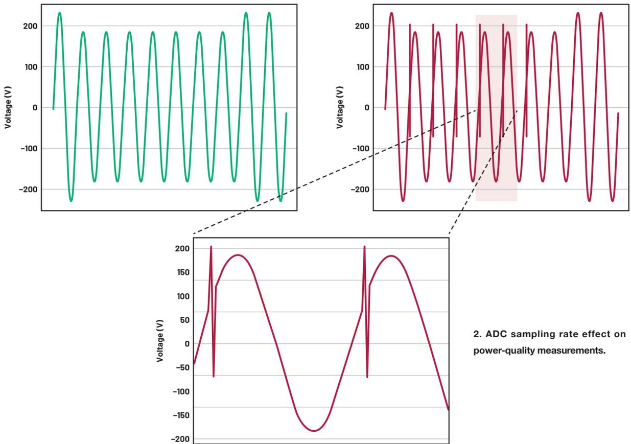
2. ADC sampling rate effect on power-quality measurements.
