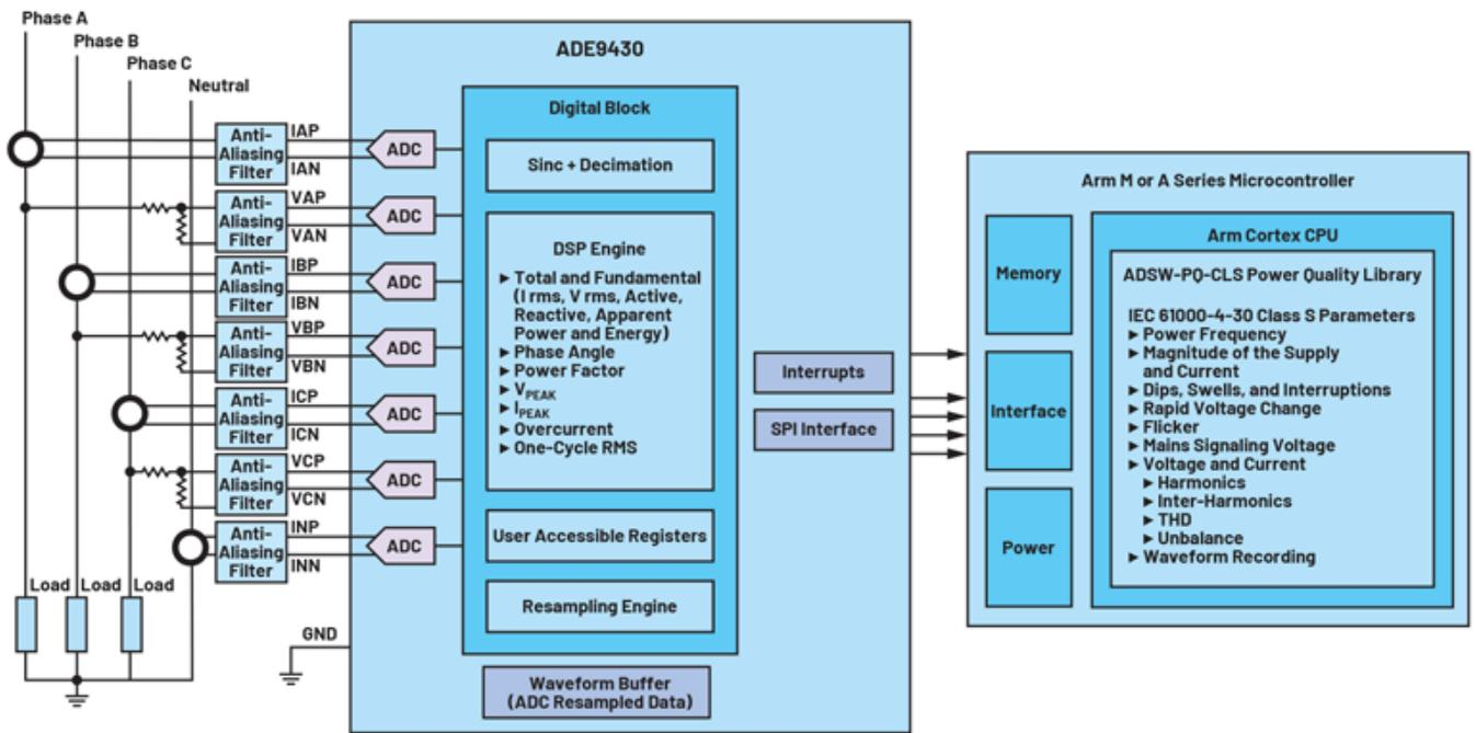
5. An ADE9430 and ADSW-PQ-CLS PQ three-phase system diagram.
