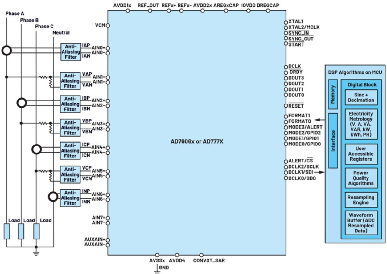
4. A power-quality three-phase applications system diagram for the AD777X and AD7606x families of ADCs.
