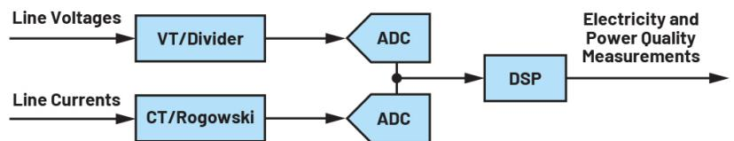
1. The main components of an instrument that handles power-quality measurements.
