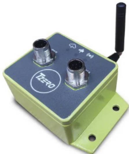
5. The RTOS Zephyr RTOS provides a lightweight, reliable platform for the firmware that drives the TZero IoT module, a simple way to collect data from industrial processes. (Image: Zephyr Foundation)
