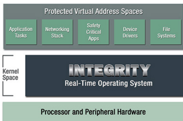
3. The INTEGRITY architecture supports multiple protected virtual address spaces, each of which can contain multiple application tasks. (Credit: Green Hills Software)
