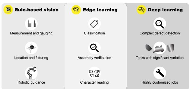
Edge learning bridges the gap between conventional rule-based machine vision and complete deep-learning solutions, thereby addressing the needs of intermediate applications.
