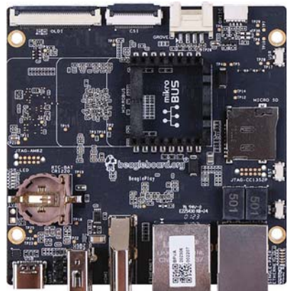
4. The BeaglePlay from BeagleBone is built around Texas Instruments' (TI) AM6254 featuring Arm Cortex-A53, Cortex-R5, Cortex-M4, and TI PRU cores. BeagleBone
