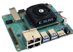
2. Xilinx's KR260 Robotics Starter Kit can be customized to include support for time-sensitive networking (TSN). Xilinx
