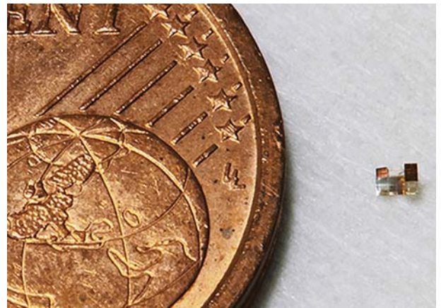
1. Shown is the finished 3D-printed MEMS accelerometer next to a 2-cent Euro coin (coin diameter is 18.75 mm/0.75 in.).
