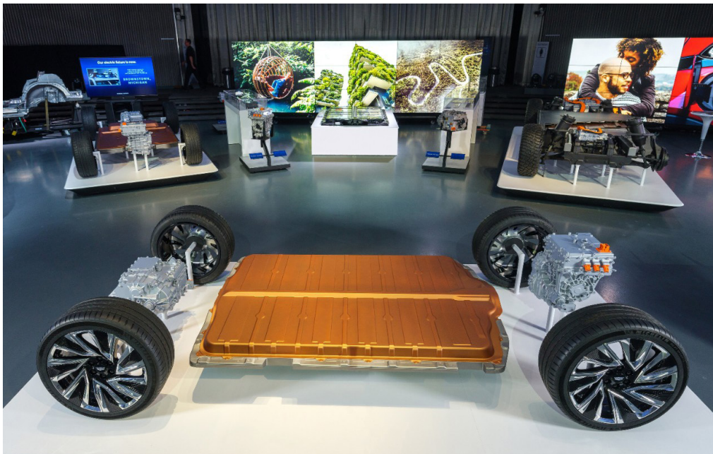
4. An Ultium modular battery pack can contain either vertically or horizontally stacked cells to integrate into vehicle design—vertically for trucks, SUVs, and crossovers, or horizontally for cars and performance vehicles. (Credit: General Motors)
