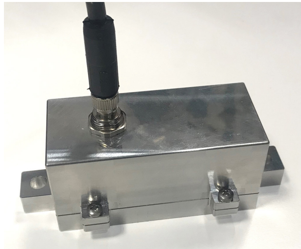
1. Shown is a 10BASE-T1L single-pair Ethernet condition-monitoring (vibration) sensor prototype.
